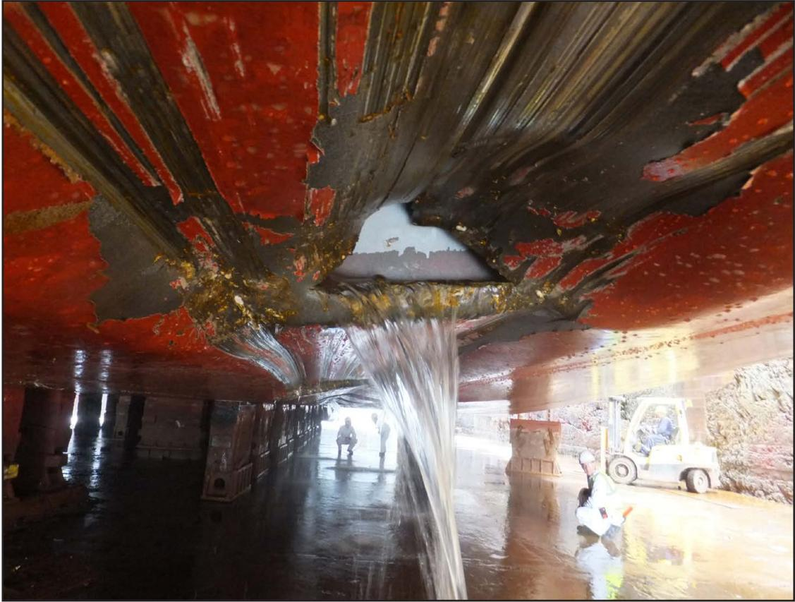
**Figure 9:** Second hole in water ballast tank 4
