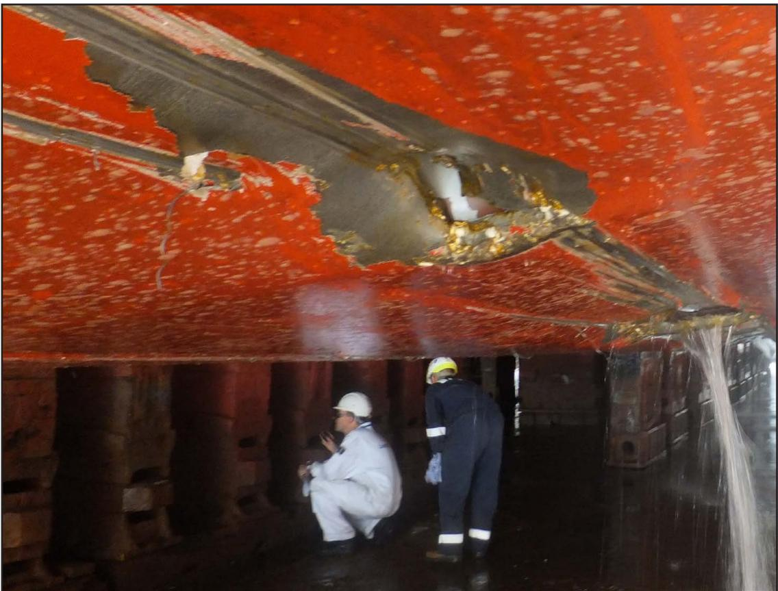
**Figure 8:** First hole in water ballast tank 4
