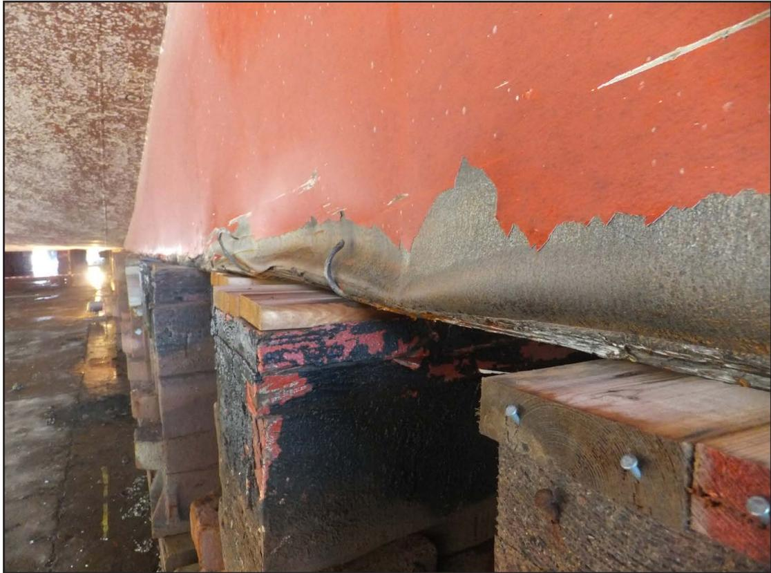
**Figure 11:** Detail of damage to keel skeg
