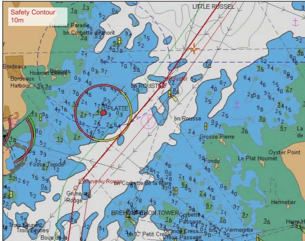
Figure 21: Comparison of ECDIS 2m and 10m safety contour lines in the Little Russel
