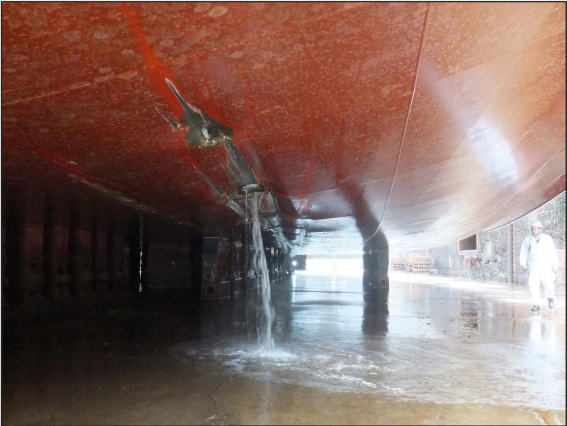
**Figure 7:** Hull gouging looking aft
