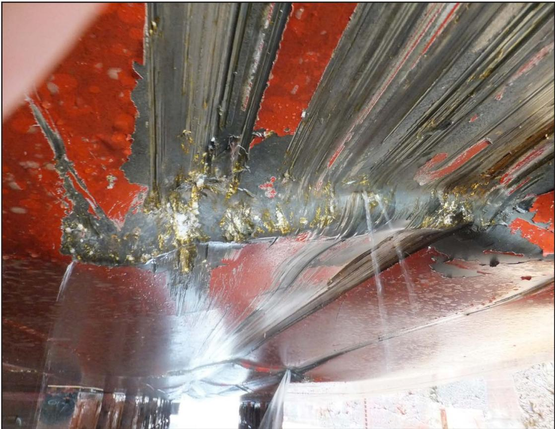
**Figure 10:** Detail of hull fracture damage
