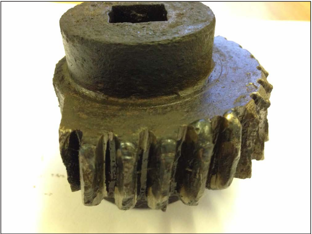
Figure 9: Gearbox quadrant, showing signs of damage and previous repair
