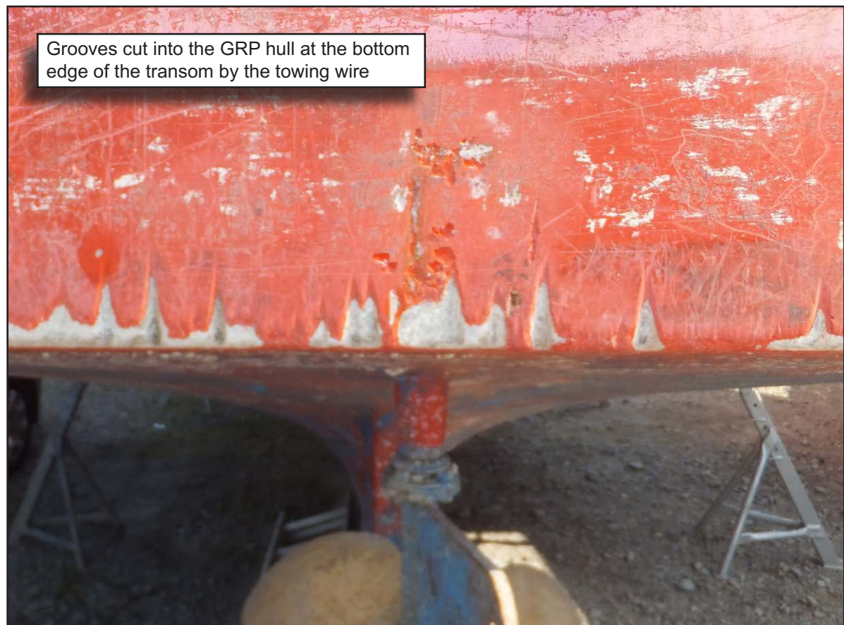
Figure 12: Damage caused to the hull by the towing wire
