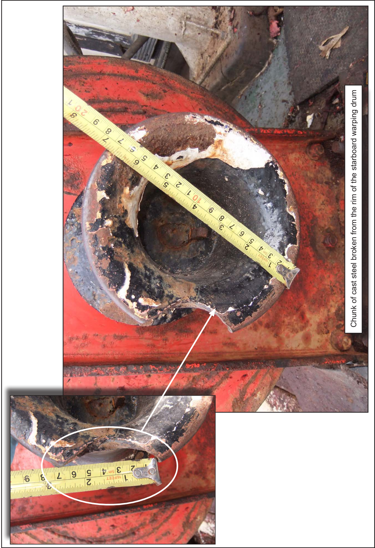
Figure 16: Damaged outer rim of the starboard warping drum
