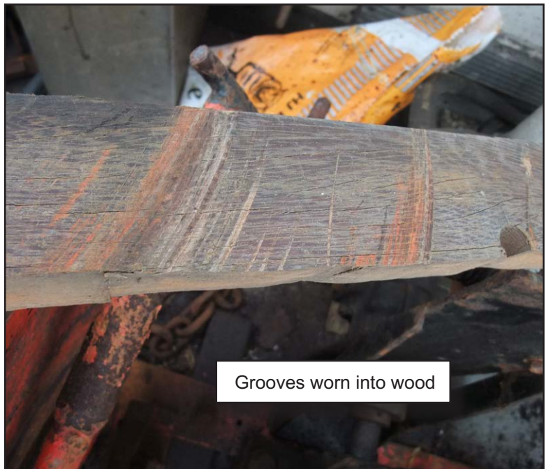
Figure 15: Plank of wood wedged between the hoisting drum flange and the winch support frame
