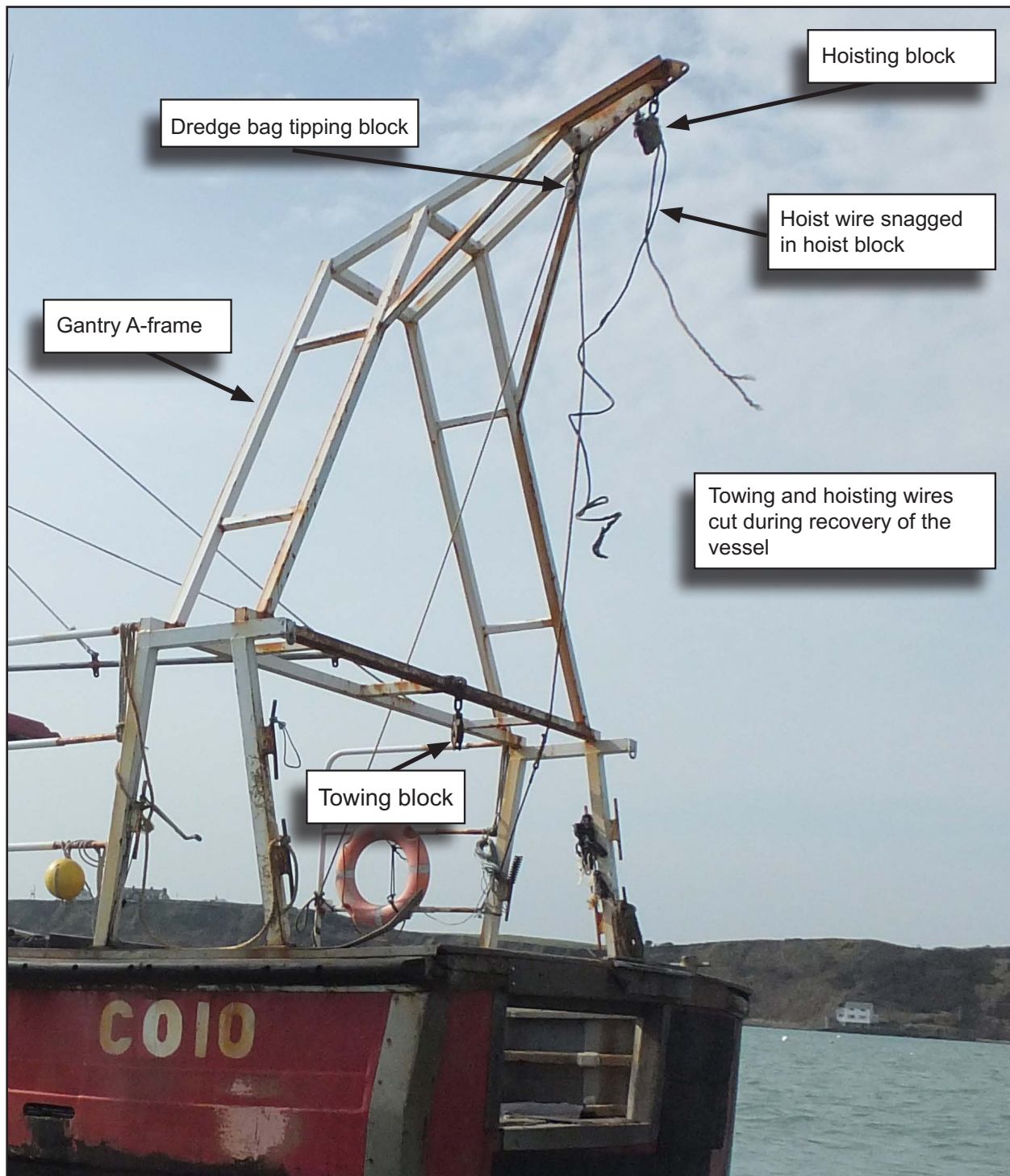
Figure 5: Ronan Orla 's modified gantry
