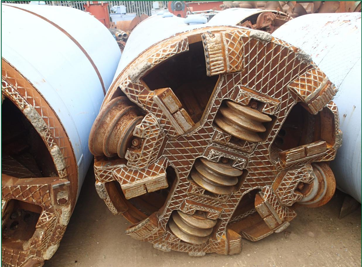
Figure 10: TBM cutter head
