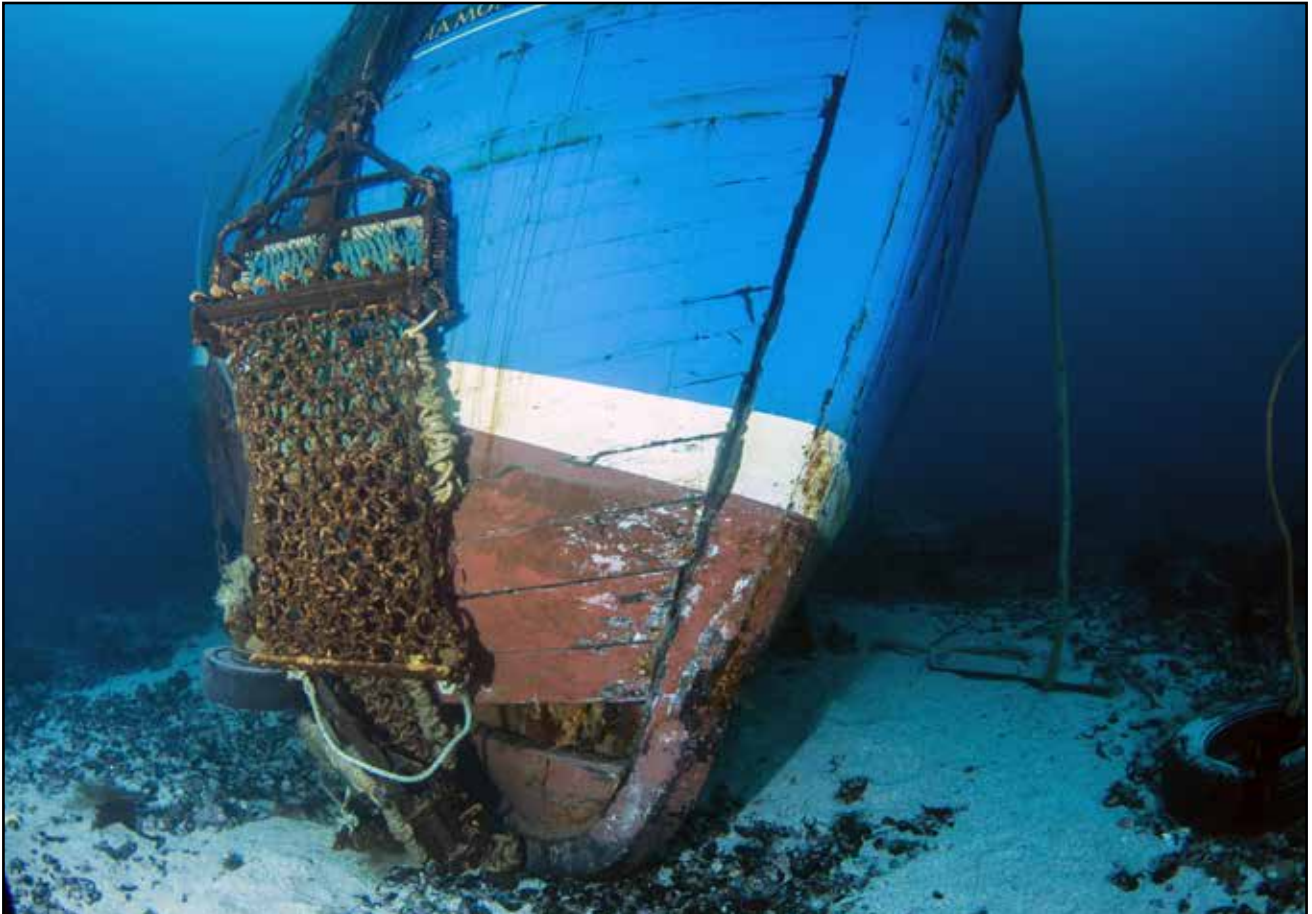
Figure 5: Photograph of stem and starboard side of Diamond showing missing and displaced planks
