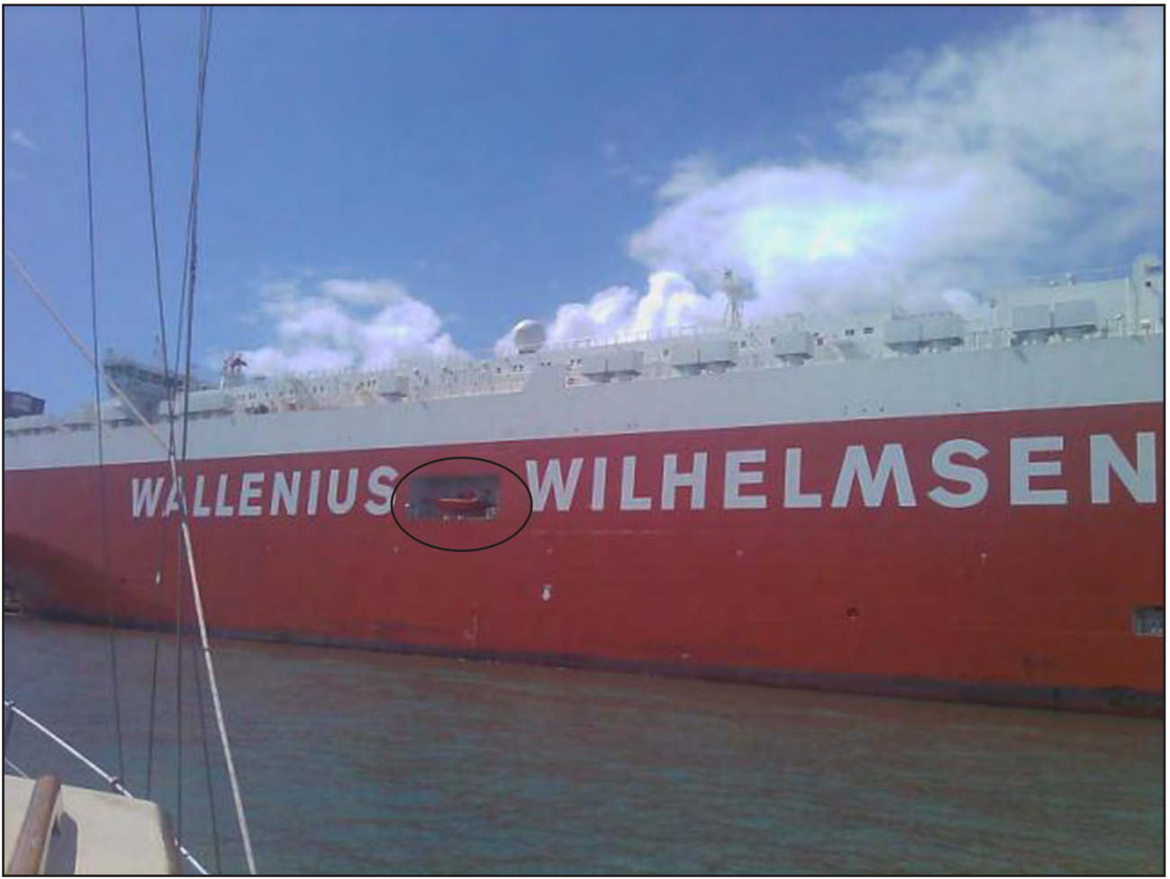
Figure 14: Rescue boat located below the upper deck on a different series of car carrier also operated by Wilhelmsen
