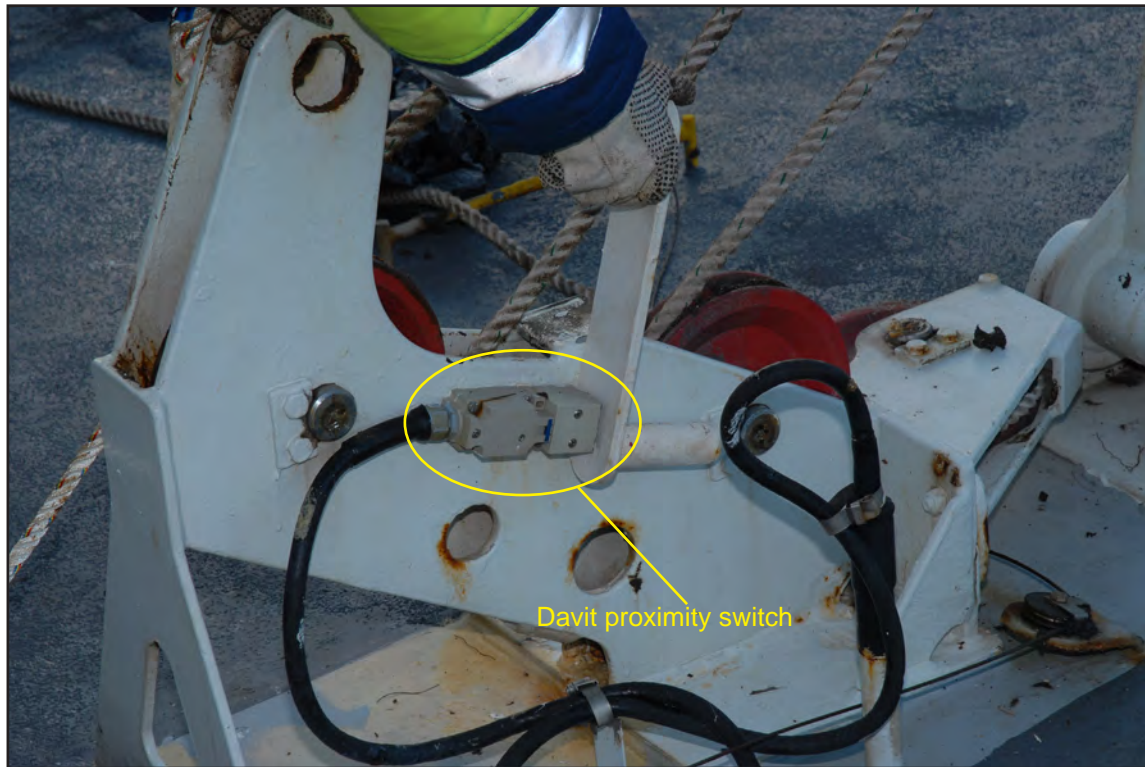
Figure 9: Proximity switch testing in situ
