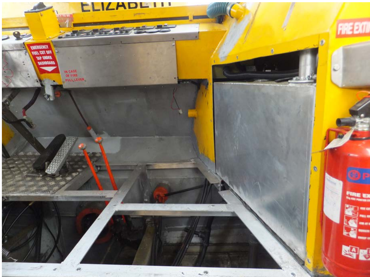
Machinery removed from port and starboard void spaces below the passenger compartment
