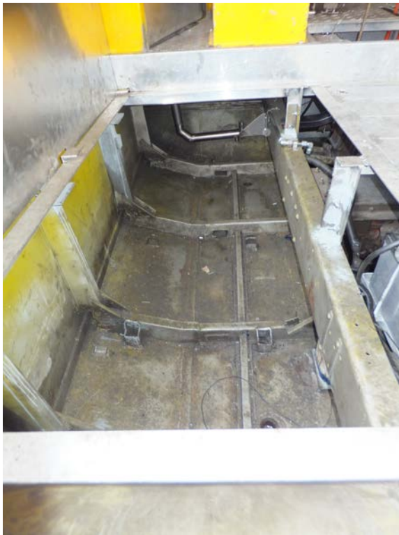
Fuel tank(s) moved forward from aft compartment
