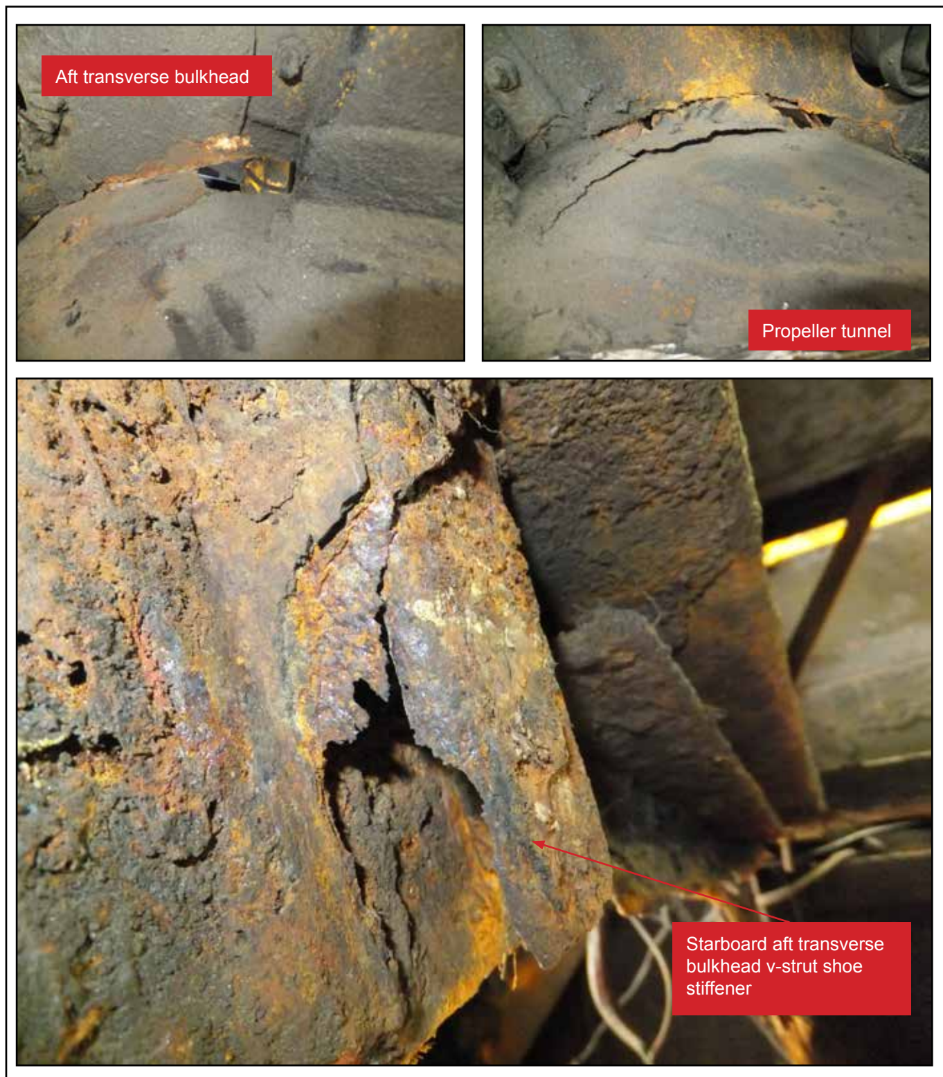
Figure 60: Hull corrosion within Wacker Quacker 1 's aft void space
