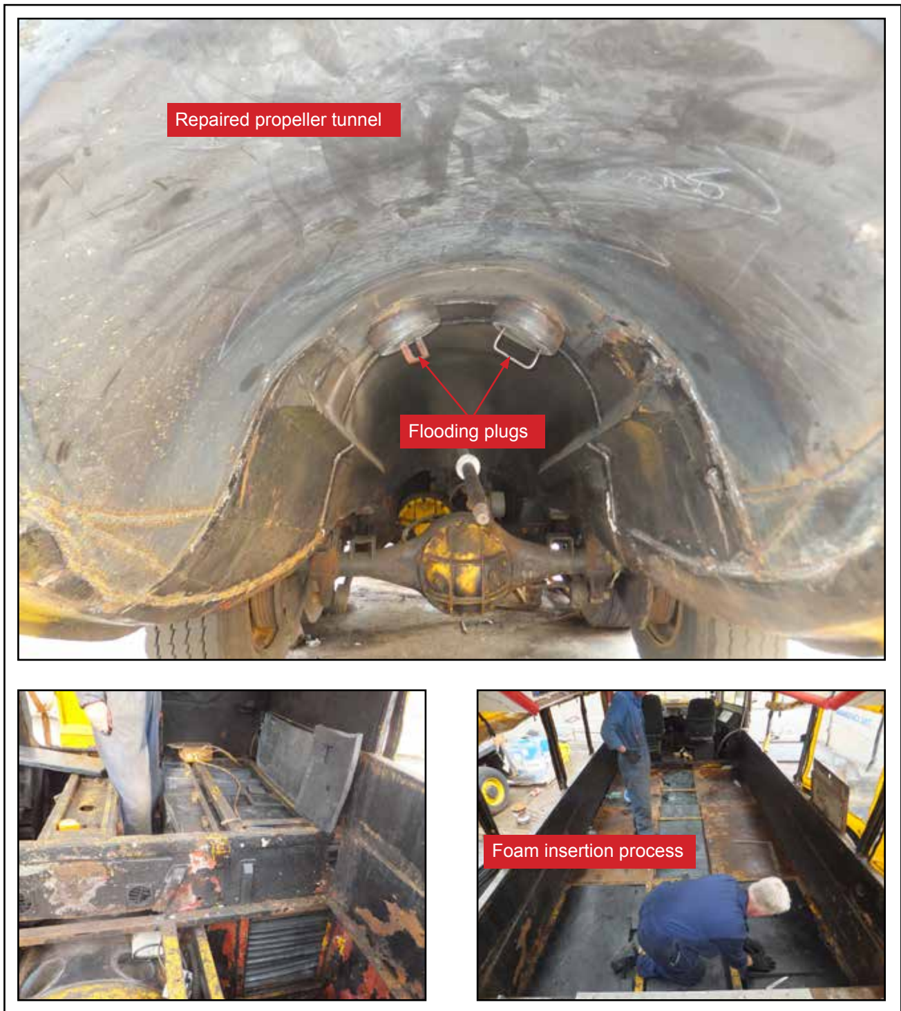
Figure 26: Hull preparations and foam insertion process
