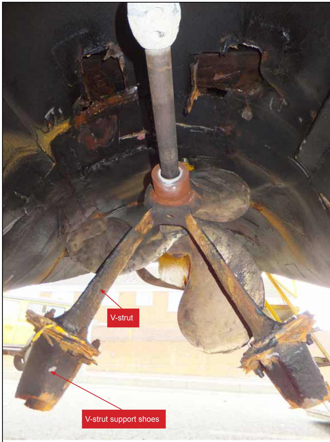
Figure 22: V-strut suspended from Wacker Quacker 1 's propeller shaft
