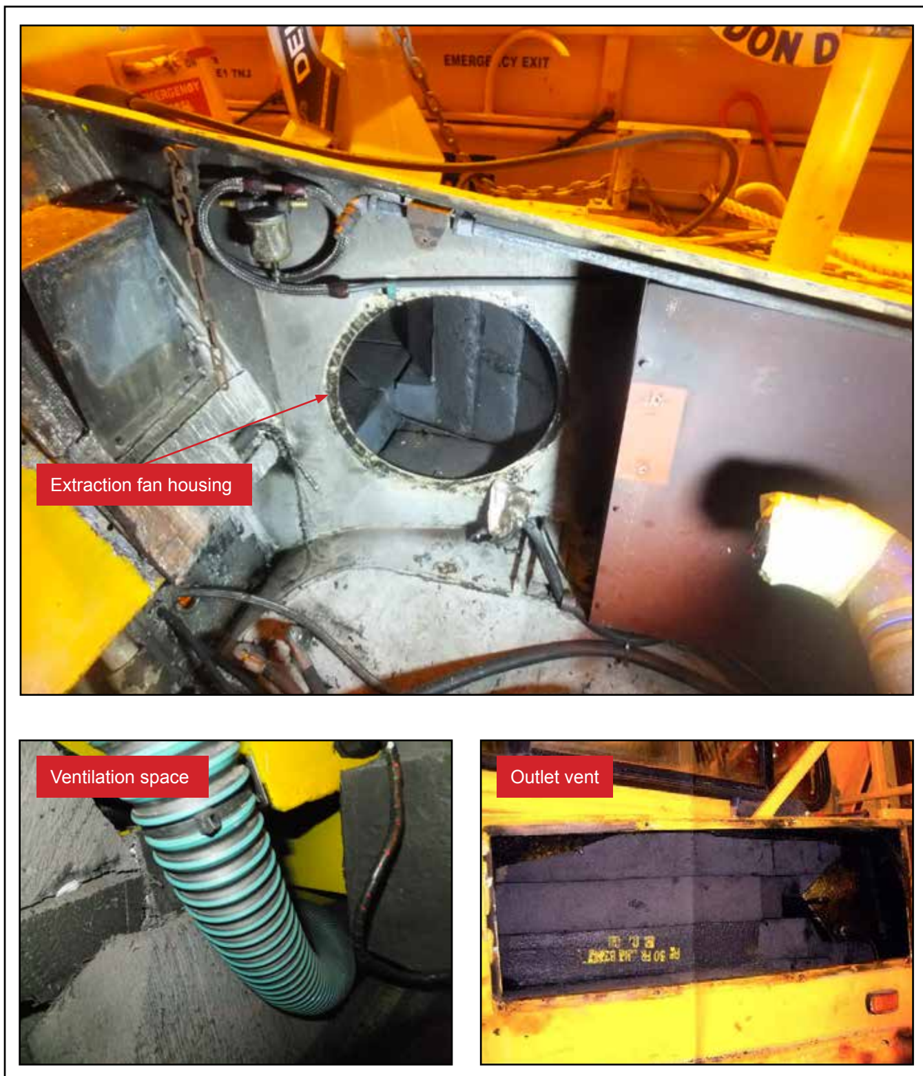
Figure 51: Buoyancy foam packed into the engine compartment ventilation void spaces
