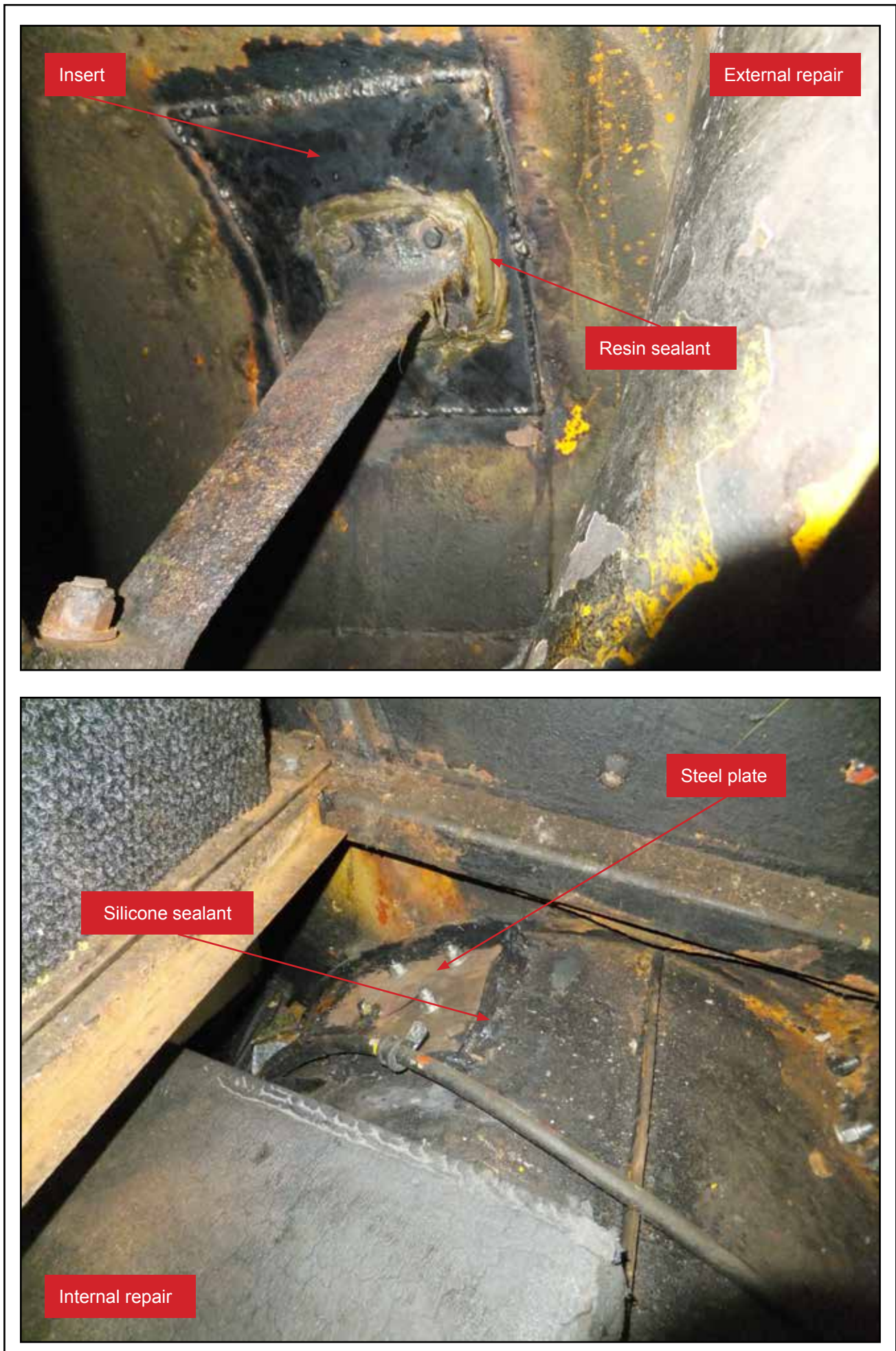
Figure 30: Hull repairs carried out by garage staff
