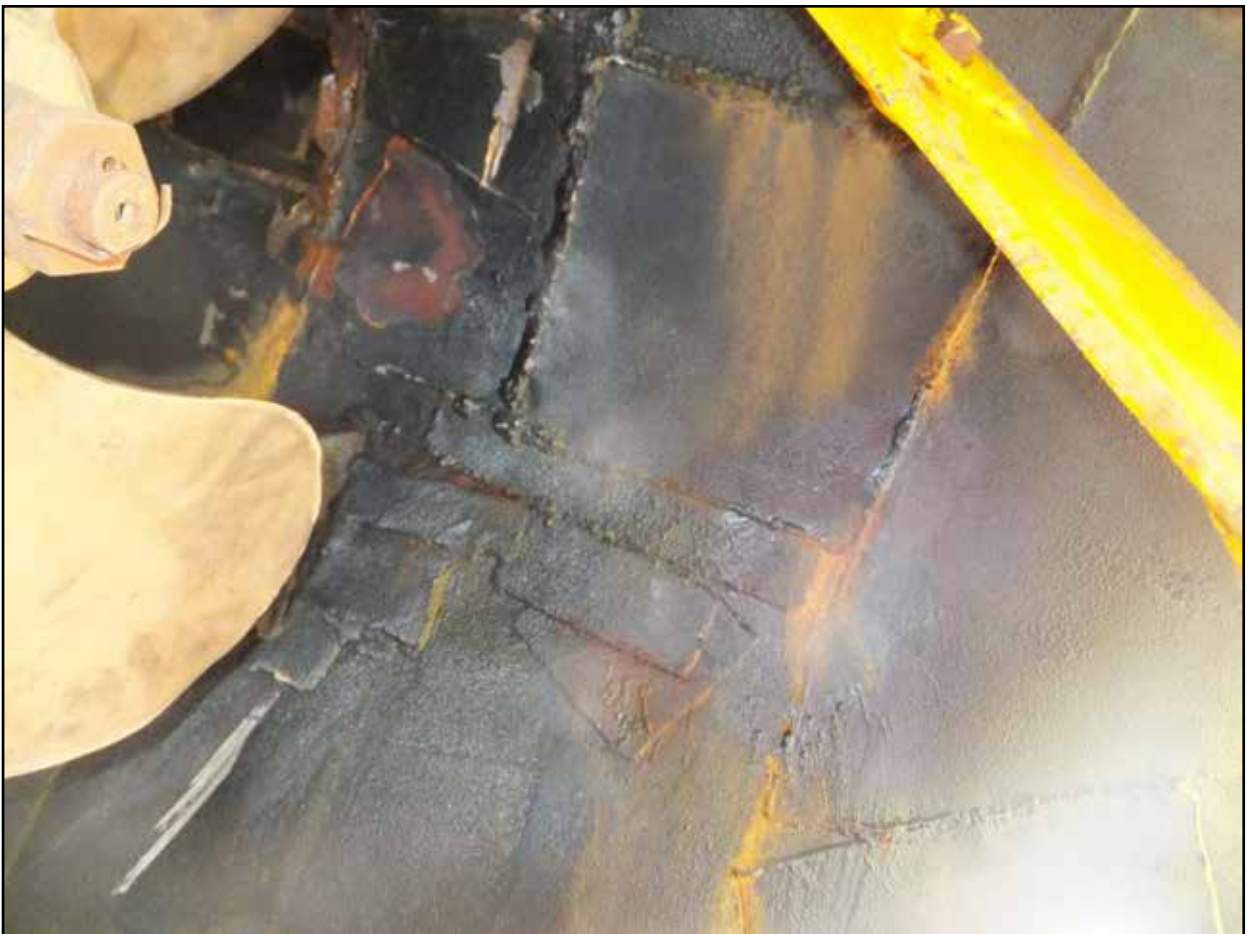
Figure 21: External patch repairs to the hull of Wacker Quacker 1
