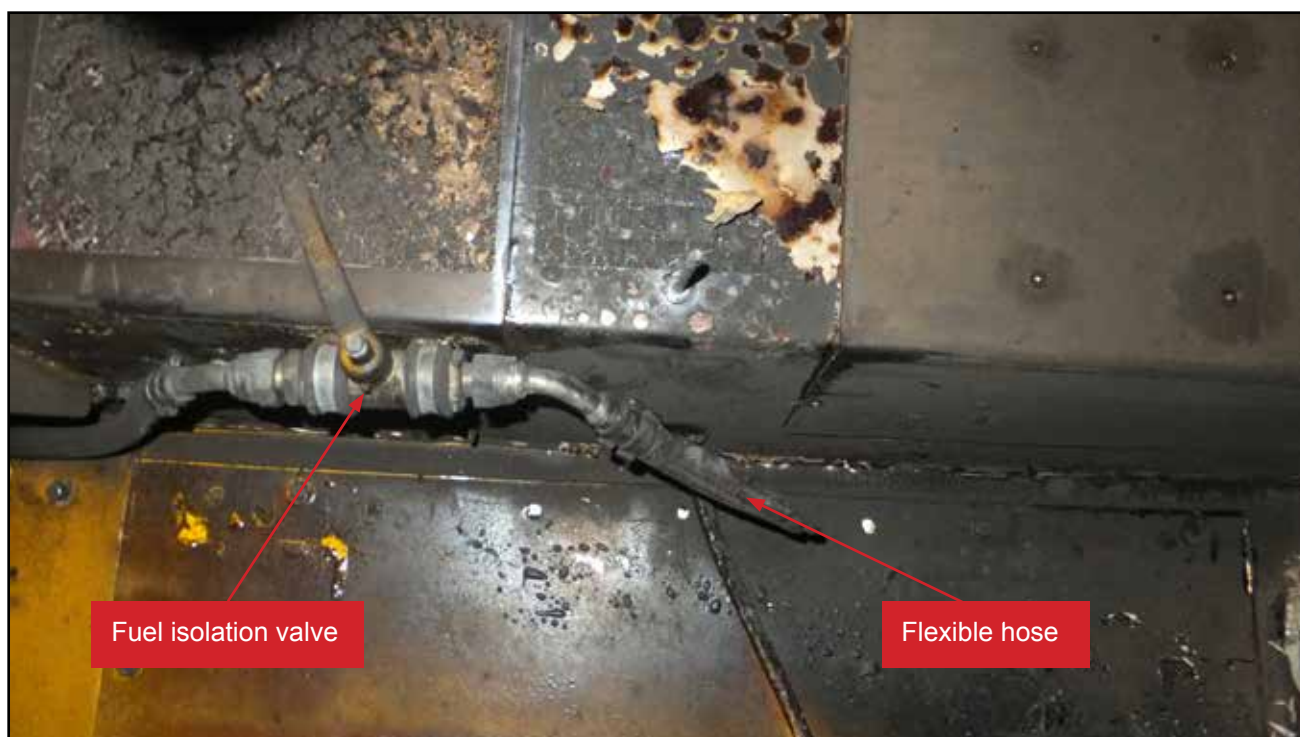
Figure 56: Burnt through section of flexible hose
