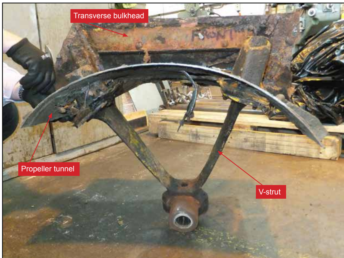
Figure 23: Sections of propeller shaft tunnel and aft transverse bulkhead cut away and despatched for metallurgical analysis
