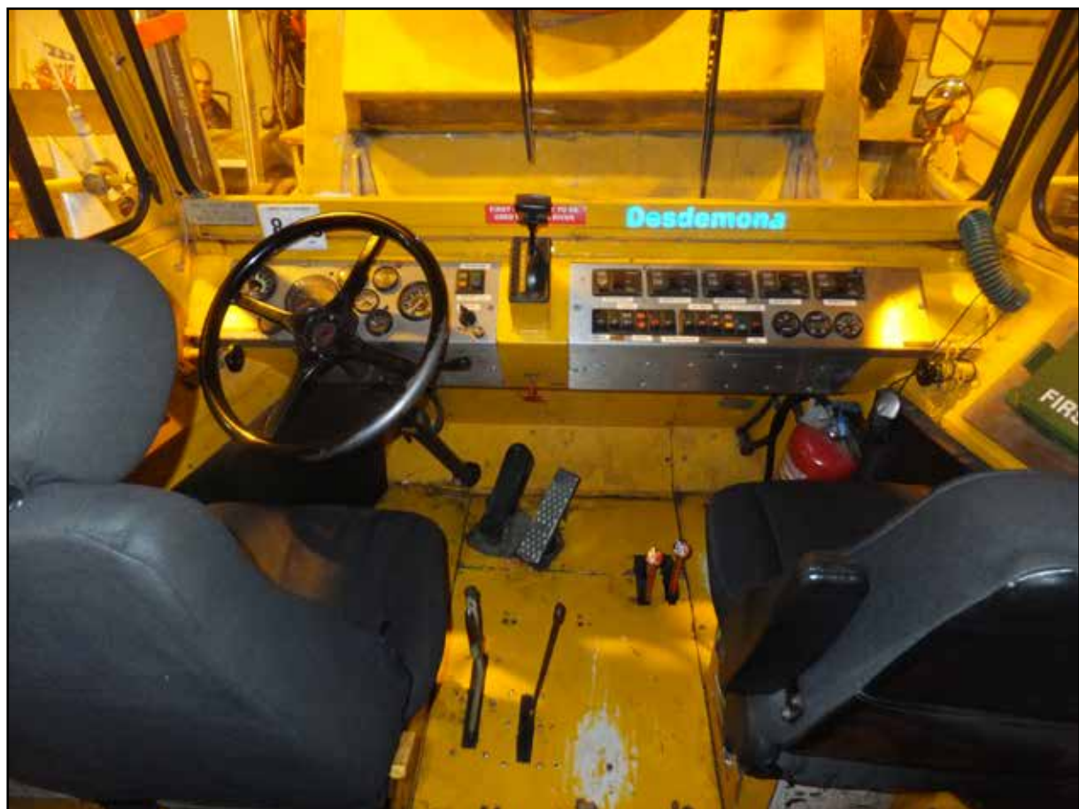
Figure 44: Typical London Duck Tours DUKW passenger compartment and crew cab layout
