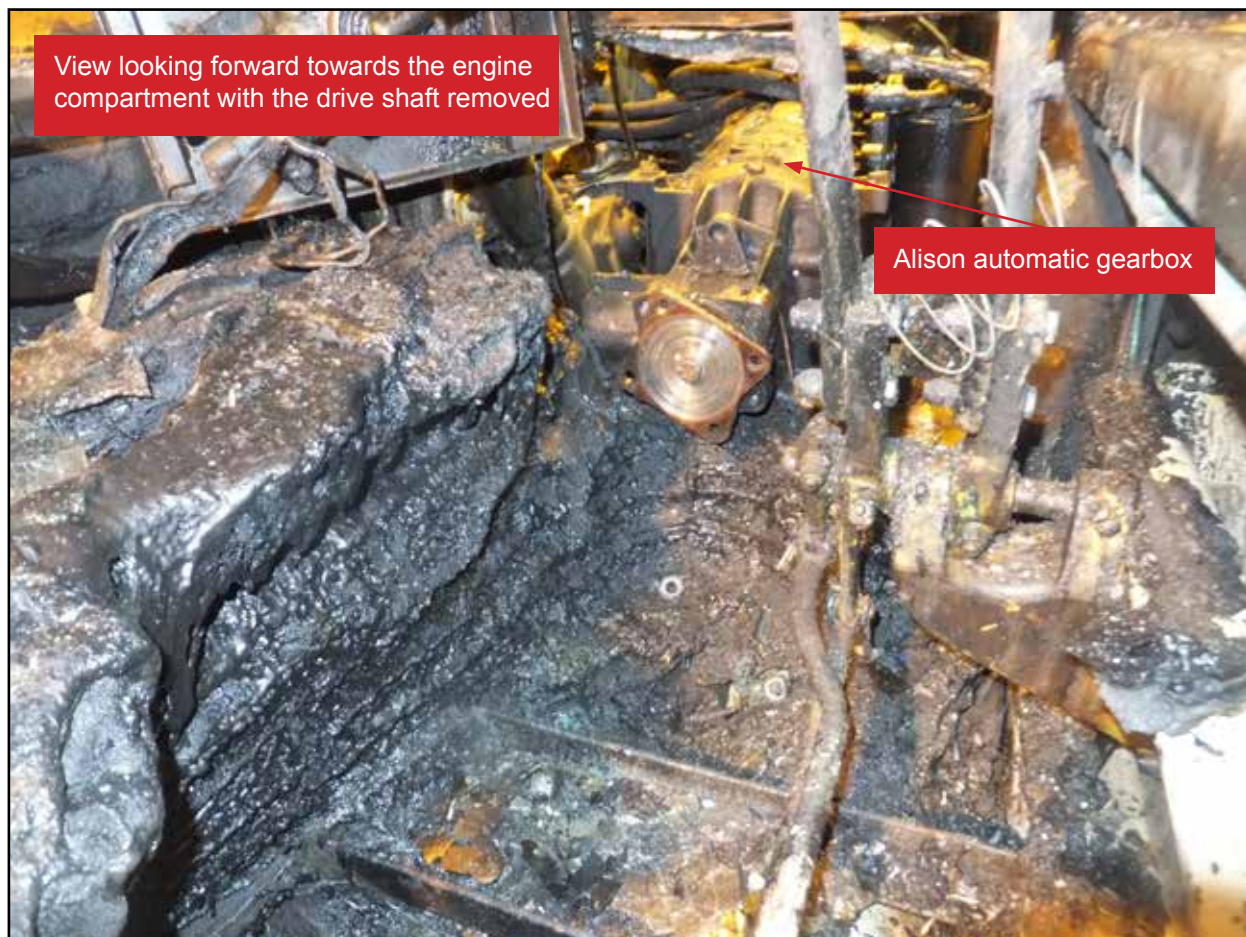
Figure 55: Area of deepest burn within central void space aft of the automatic gearbox
