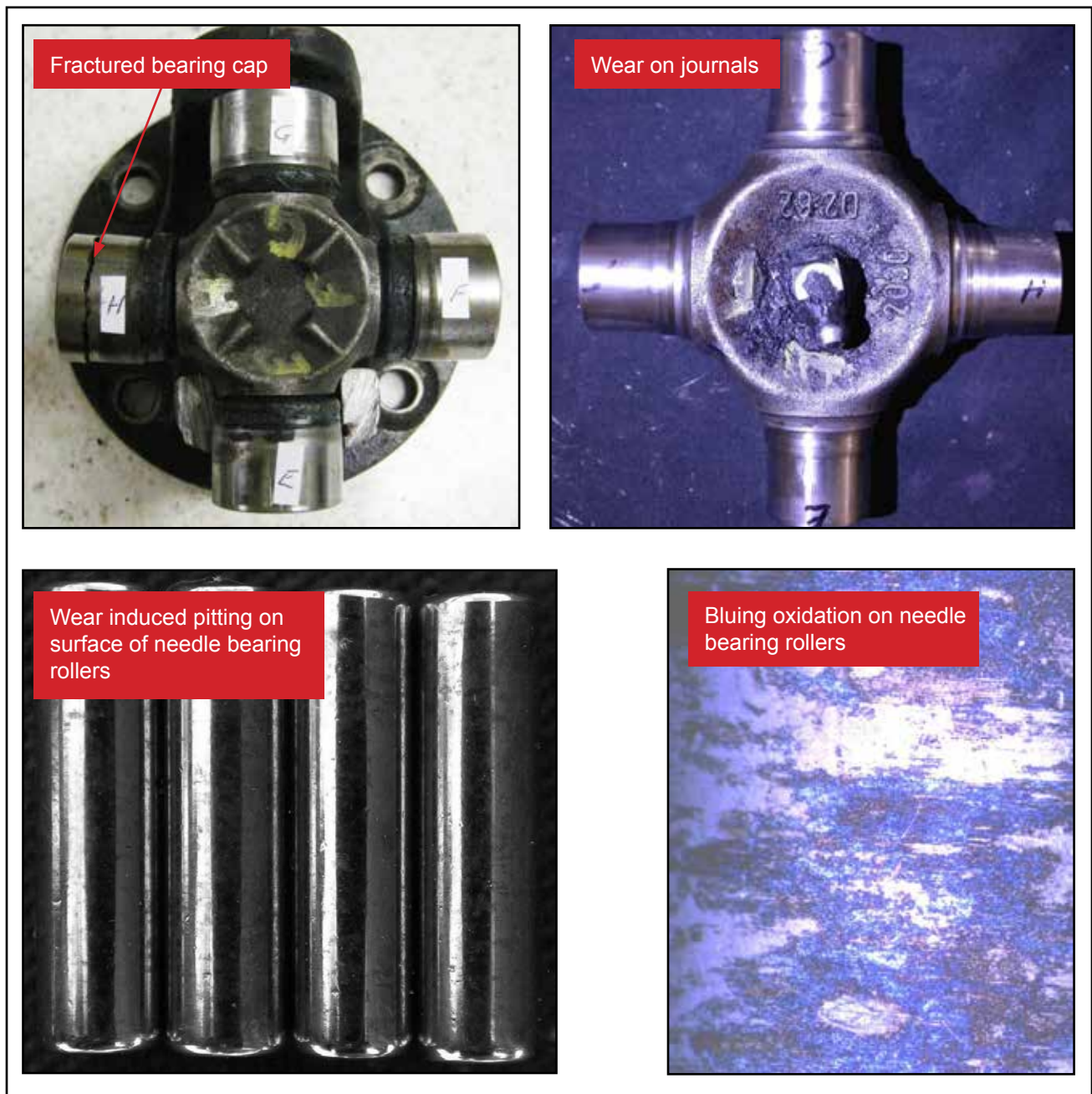
Figure 58: Laboratory analysis of the forward drive shaft universal joint
