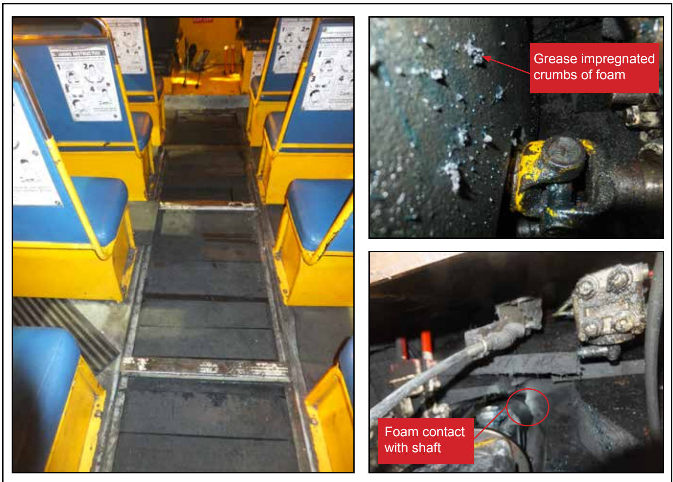
Figure 59: Tightly packed foam in central void space
