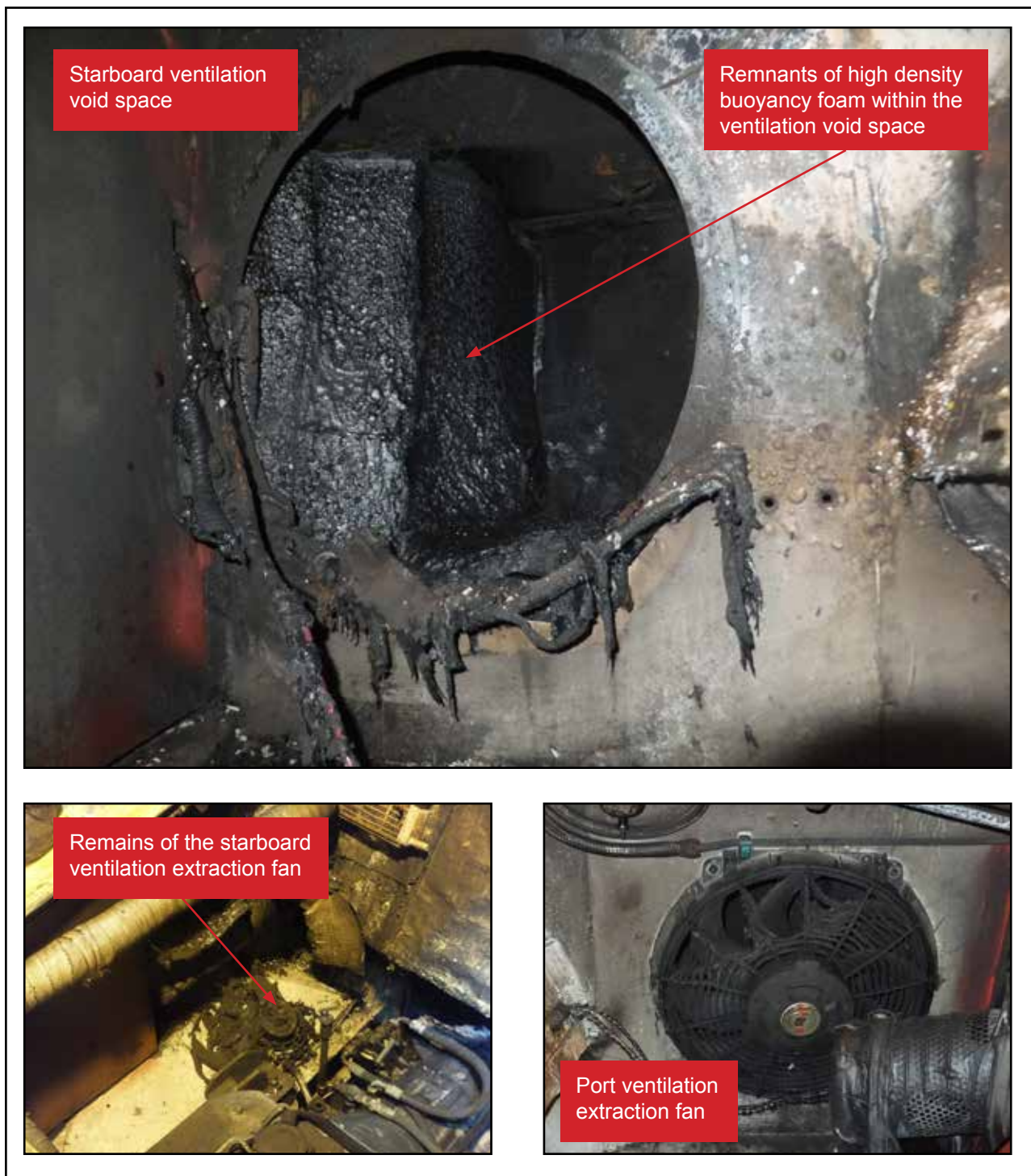
Figure 53: Fire damage within the engine compartment and starboard ventilation void space
