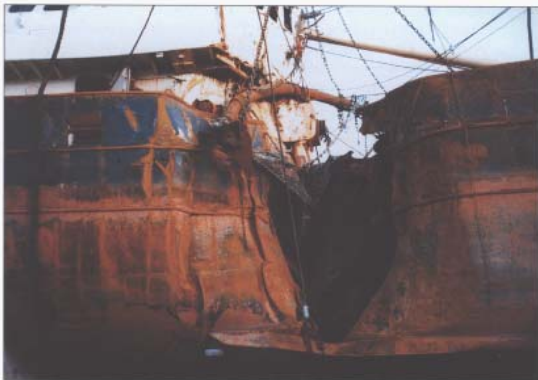
Figure 9: Damage to FV LARISSA shows serious hull failure (Note the bilge keel is bent down and split from the hull)
