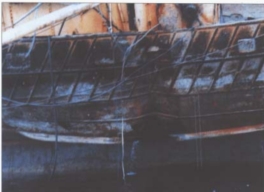
Figure 10: Damage to WILHELMINA J is severe with hull failure from keel to top of rail with damage to derrick and associated gear
