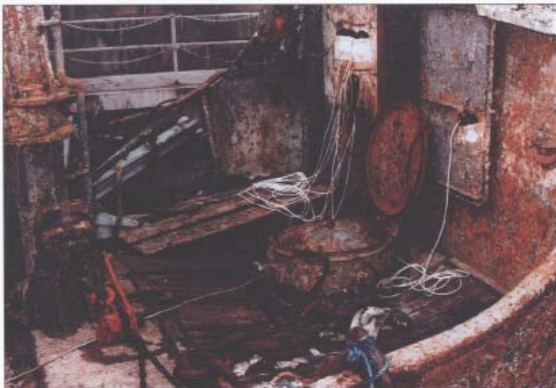
Figure 8: View of fore deck showing damage to deck sheathing. [Photograph by courtesy of the Chief Constable of the Devon and Cornwall Constabulary]
