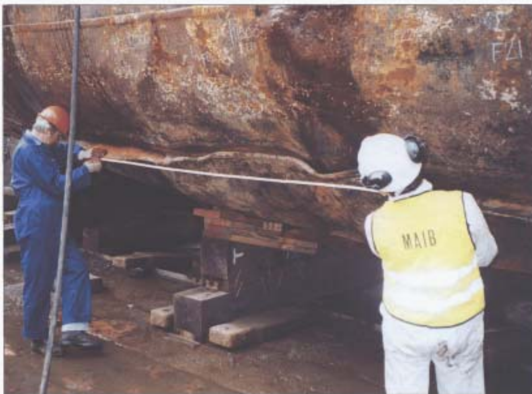
Figure 7: Damage in way of starboard bilge keel
