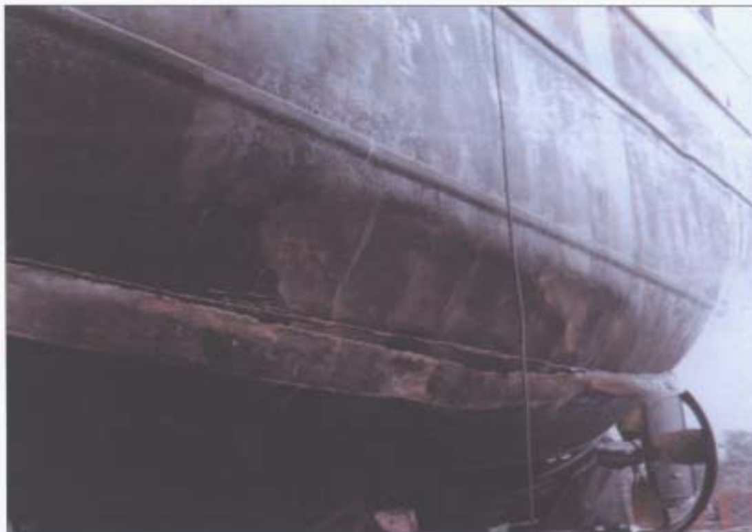
Figure 11: Photograph shows minor collision damage with bulbous bow vessel (Note bilge keel is deflected downwards and split away from the hull) [Photograph courtesy of Hodge Jones and Allen, Solicitors]
