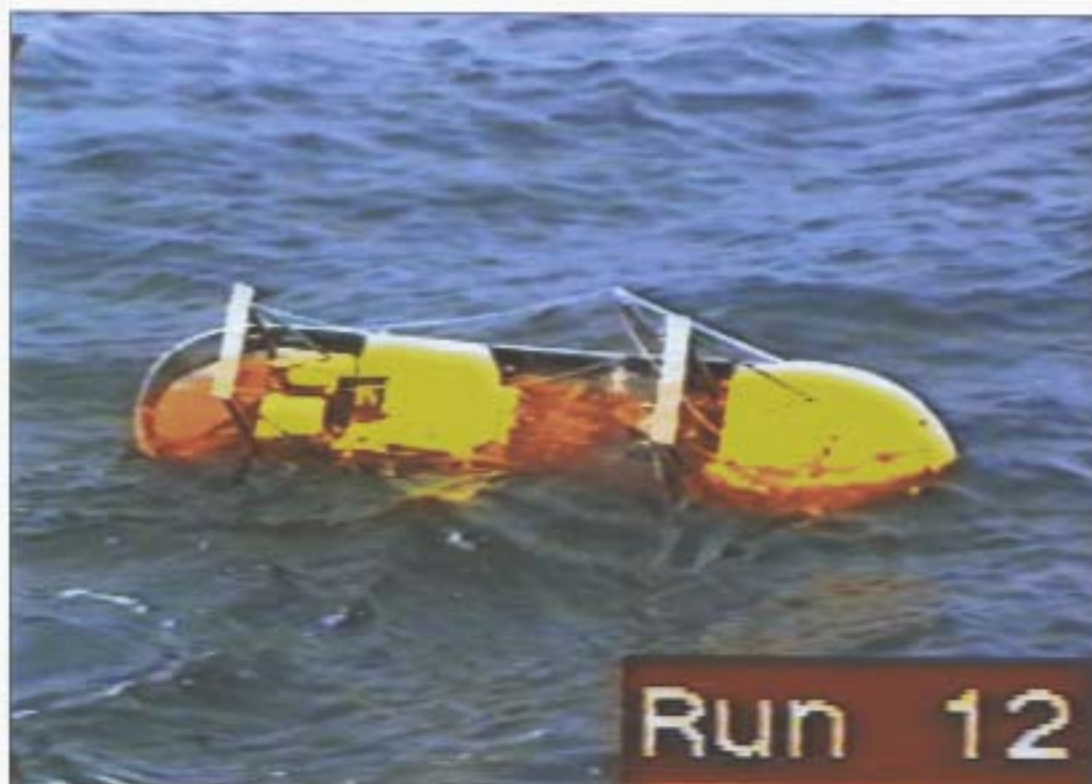
Figure 14: Model heeled heavily to starboard with weather deck awash and wheelhouse flooded
