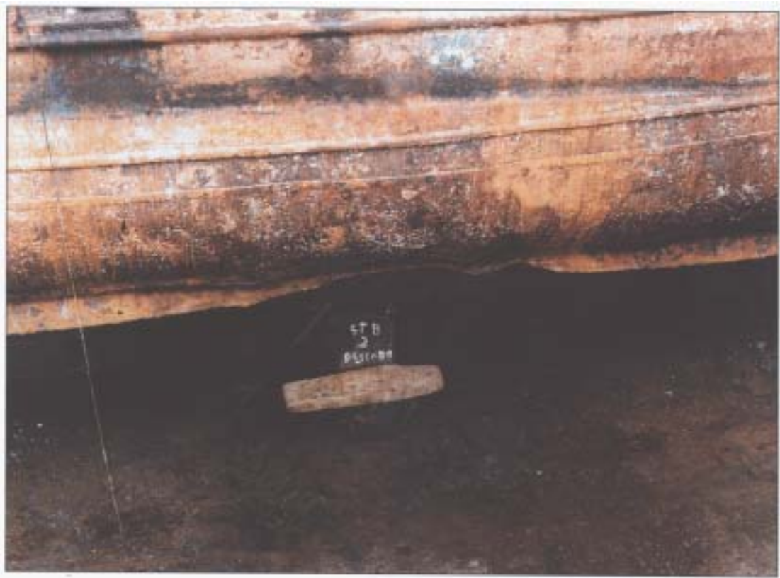
Figure 12: Local damage to PESCADO’s starboard side as seen in dry dock [Photograph by courtesy of the Chief Constable of the Devon and Cornwall Constabulary]
