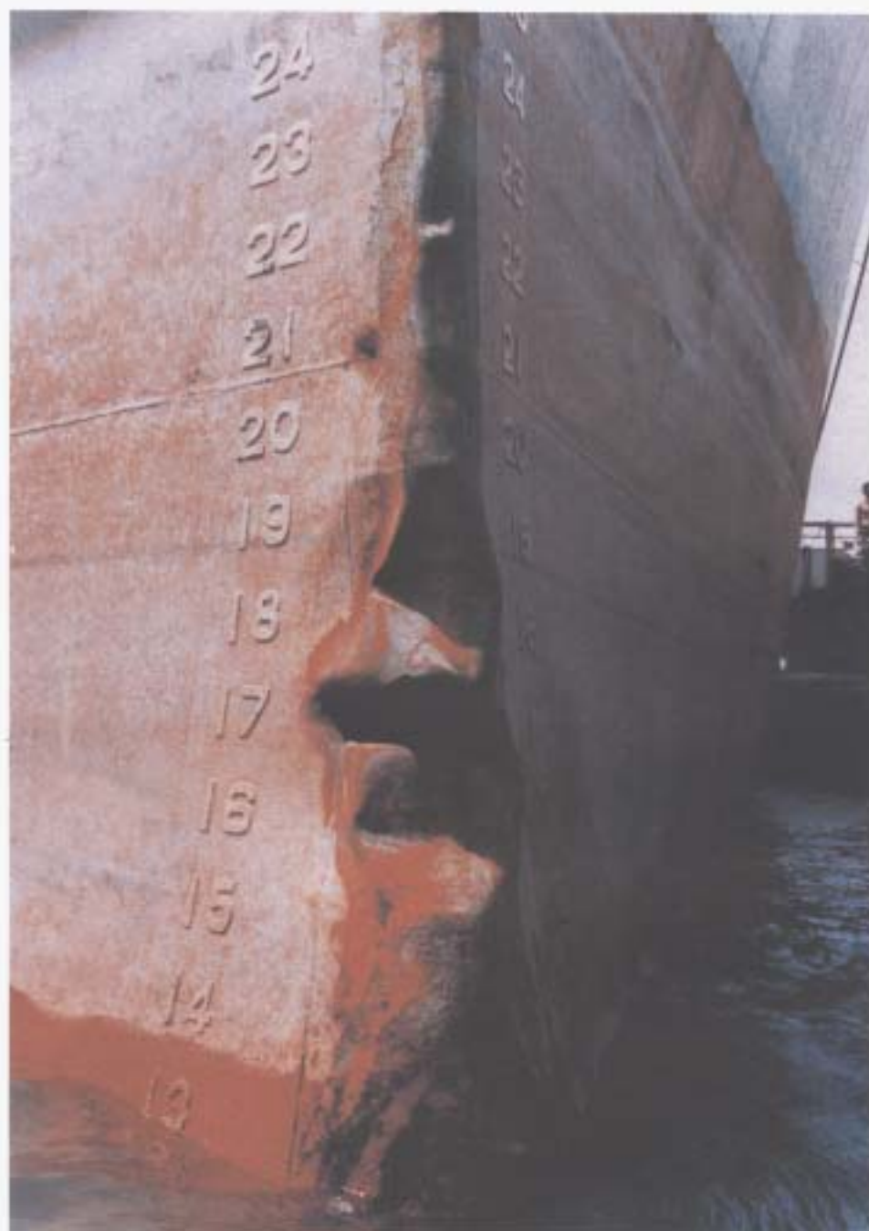
ZULFIKAR - FORWARD VIEW OF DAMAGE TO BOW
