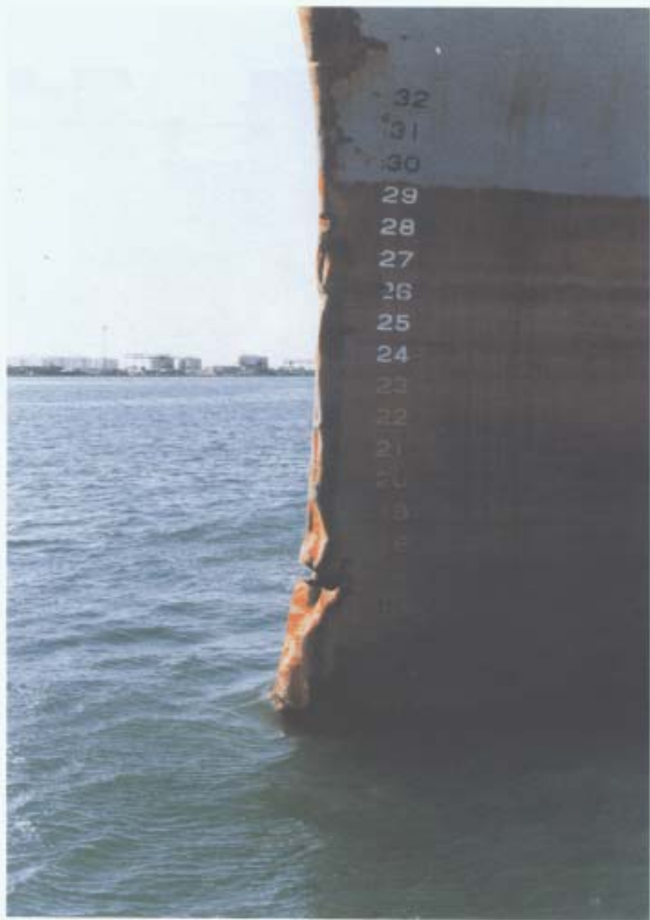
ZULFIKAR - SIDE VIEW OF DAMAGE TO BOW
