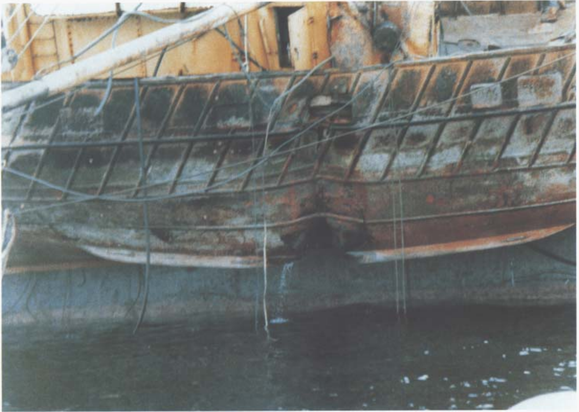
WILHELMINA J - DAMAGE TO STARBOARD SIDE OF HULL
