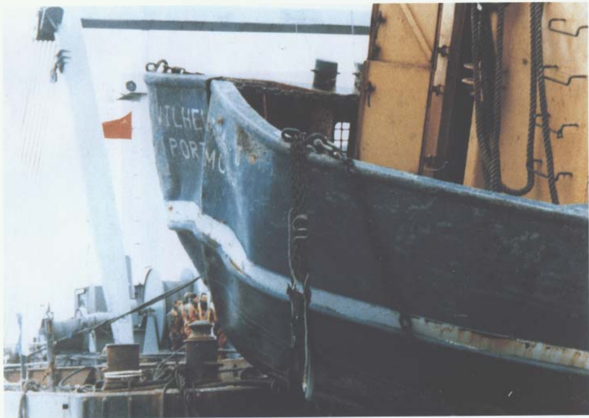
WILHELMINA J - DAMAGE AT STERN
