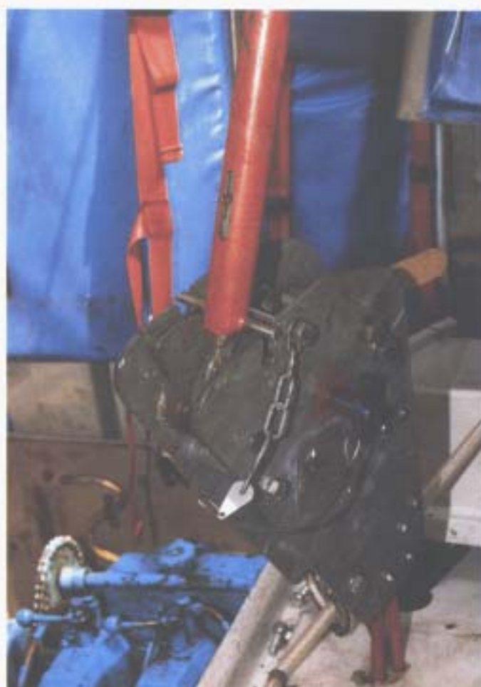
Release handle assembly pin fully home (as found by Inspector)
