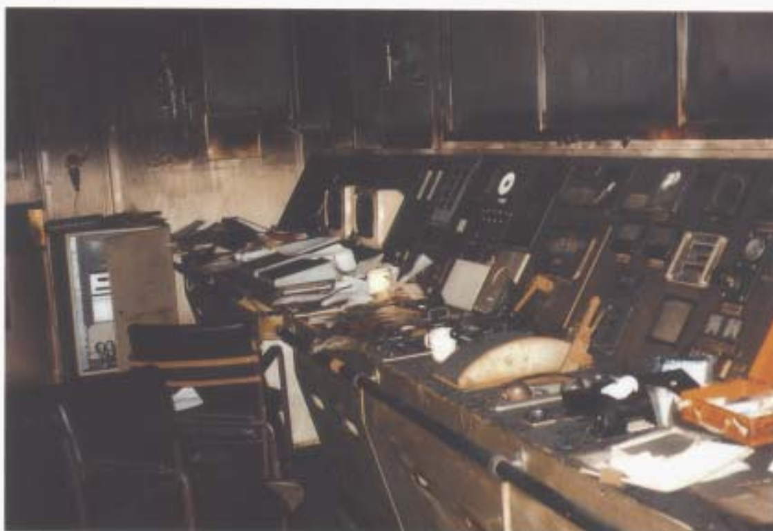
BRITISH TRENT - Extent of heat and smoke damage in engine control room
