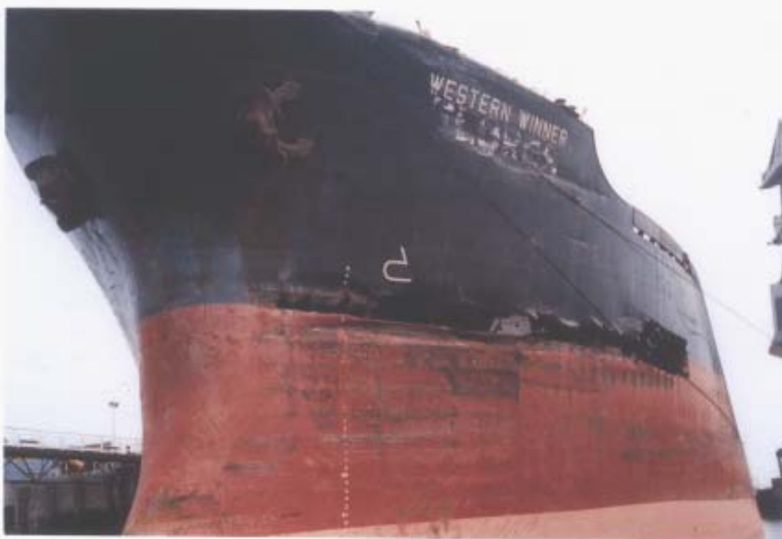
WESTERN WINNER - showing extent of damage to Port bow
