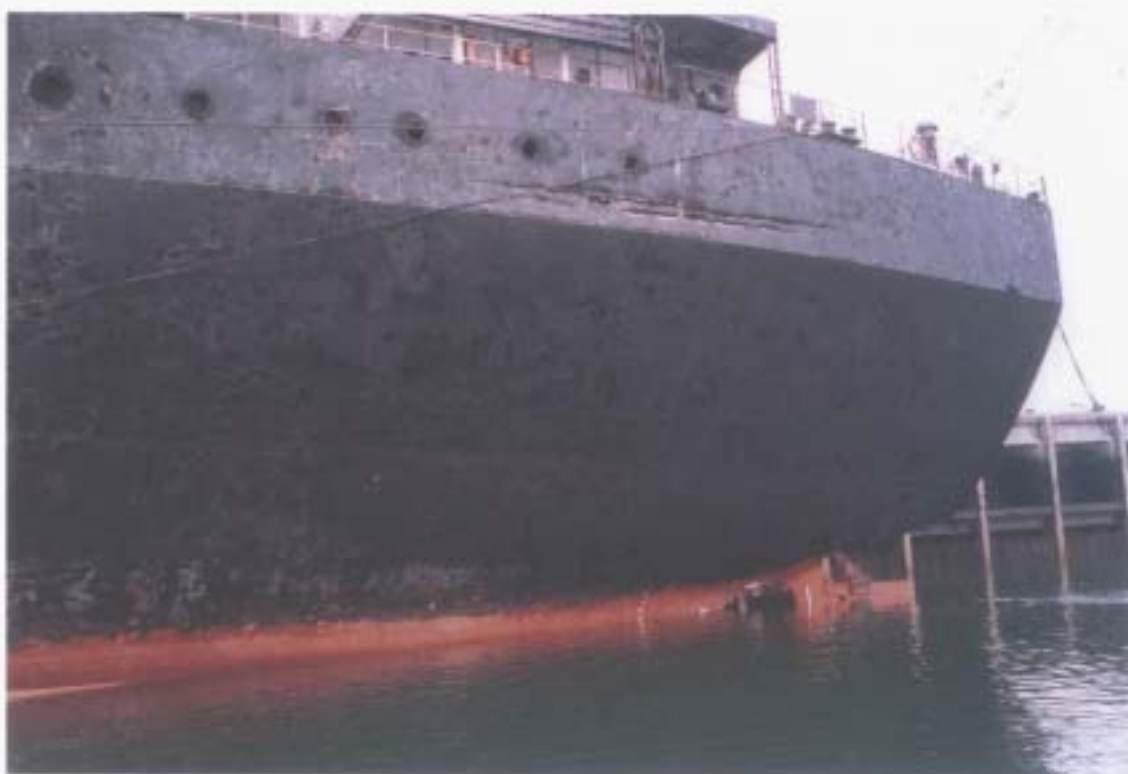
WESTERN WINNER - Port quarter showing collision damage and fire scorched paintwork
