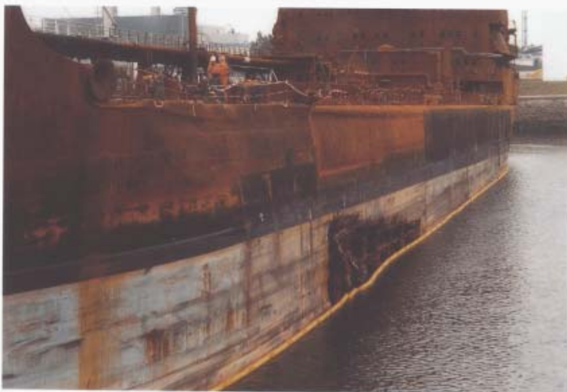
BRITISH TRENT - Port side showing the ruptured tanks and distorted sheerstrake
