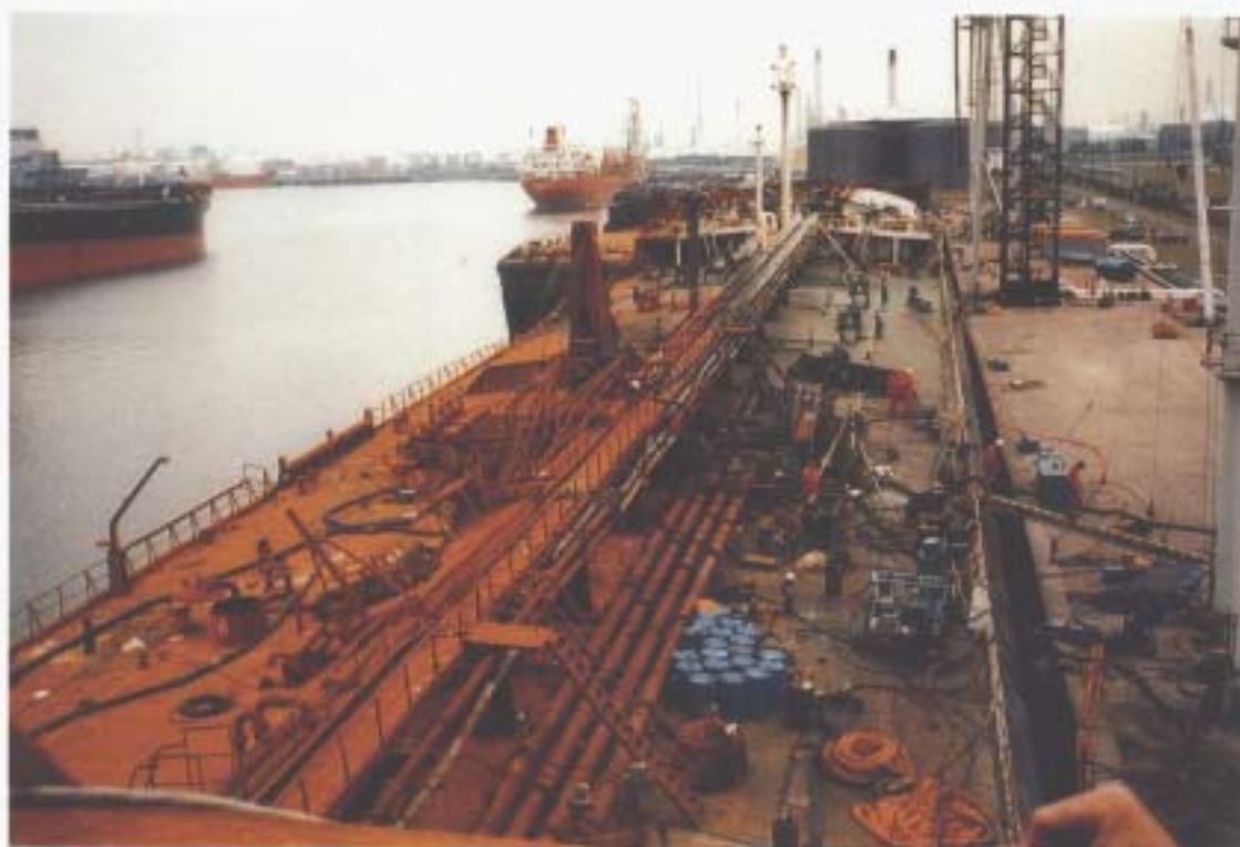
BRITISH TRENT - View of main deck clearly showing the boundary between the fire damaged and undamaged areas
