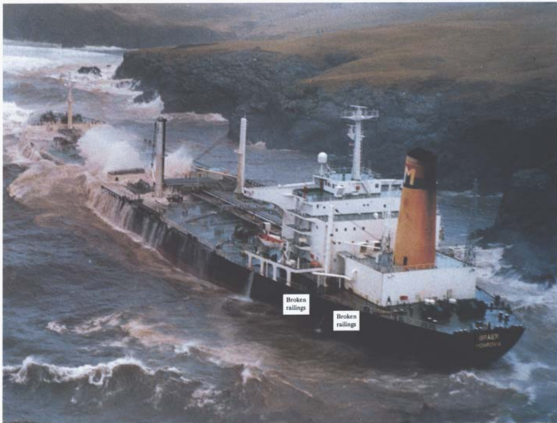
BRAER aground showing broken rails port side aft in way of air pipes
