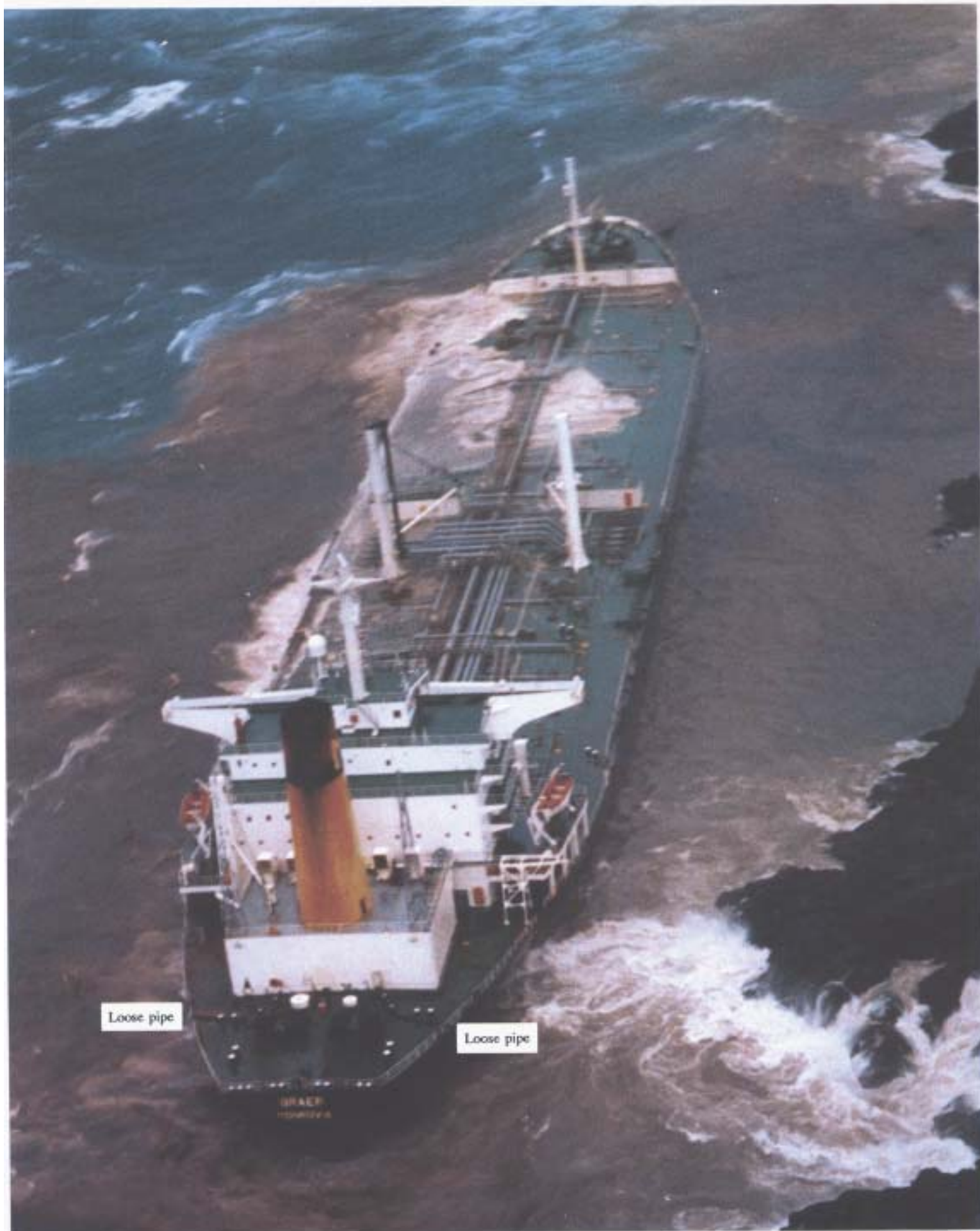
BRAER aground showing loose pipes, port and starboard sides aft
