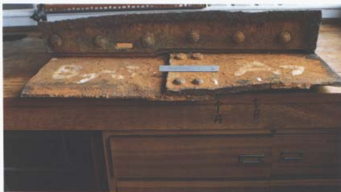
Oblique view of fracture of B7, A7. Note wastage of B7 and sources of fracture A and B.
