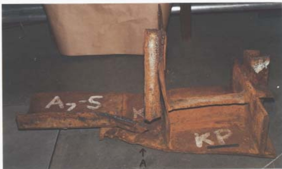
Part of A7 (starboard) and part of keel plate.
