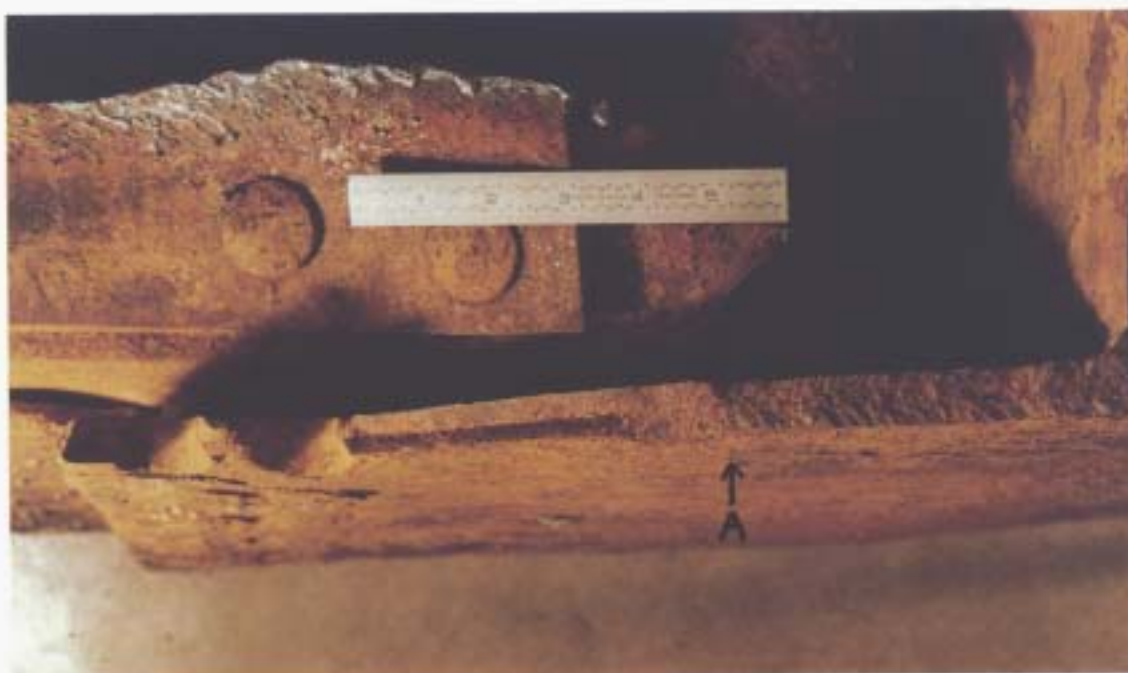
Detail of fracture in keel plate, showing transition from ductile fracture to brittle fracture at A. Fracture has progressed from left to right (starboard to port).
