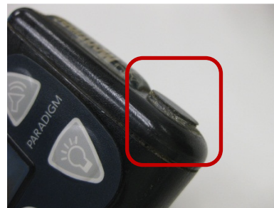
Loose Drive Support Cap- Cap sticking out
