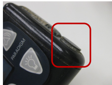
Loose Drive Support Cap- Cap sticking out
