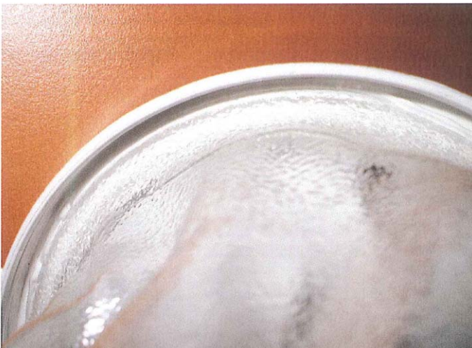
Image depicting misalignment of the Receptal liner within the Receptal liner lid. Towards the top, the liner is close to the edge of the lid; on the right there is a gap
