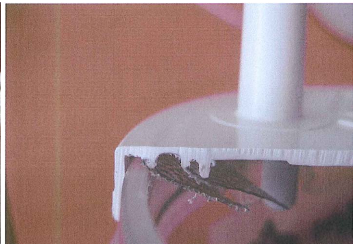
Image highlighting how the misaligned liner prevents a flush connection of the lid with the edge of the canister, which gives rise to inadequate vacuum.
