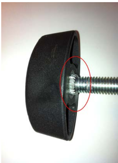
Fig. 1 Wing handle to ReTurn where the attachment of the screw is visible in the handle.
