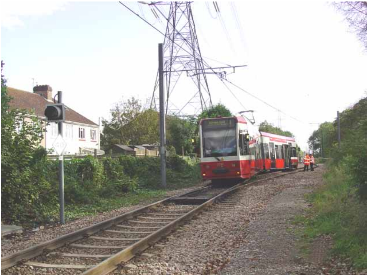
Figure 5: The derailed tram from the rear, showing the points position indicator and speed restriction sign
