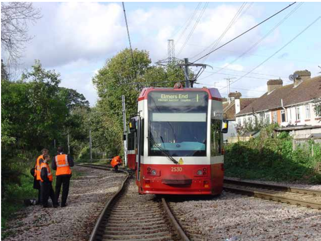
Figure 4: The derailed tram from the front, showing distortion of the track
