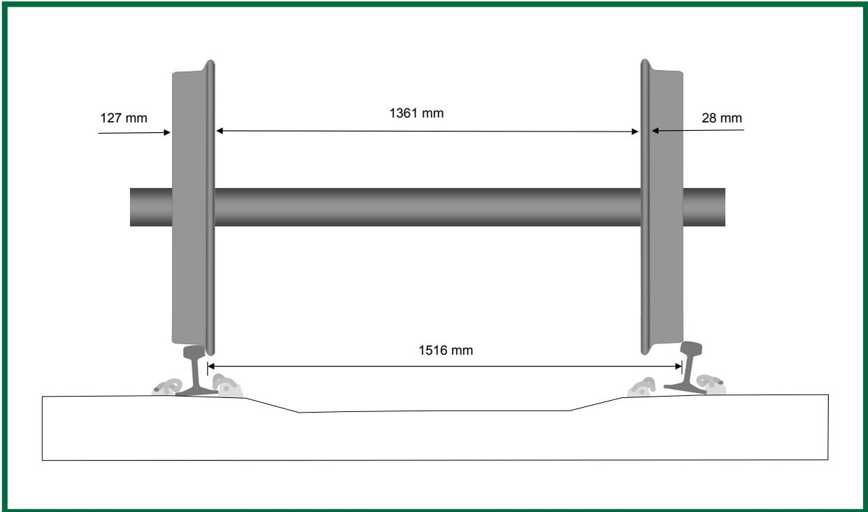
Figure 8: Diagram of critical gauge spread dimensions to cause derailment
