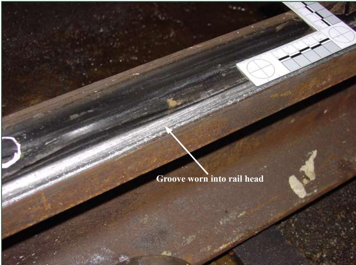
Figure 11: Groove on the low rail just before the point of derailment
