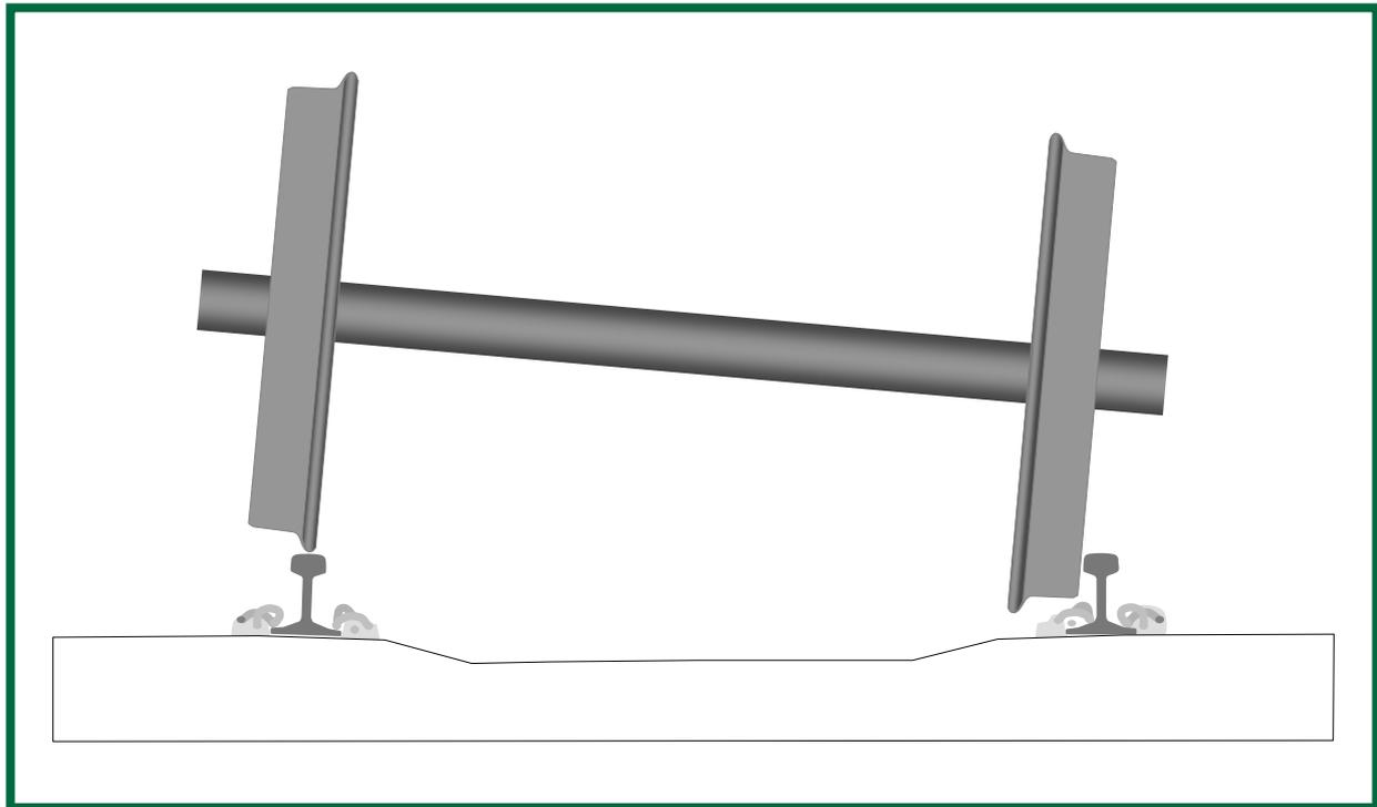
Figure 10: Diagram of wheelset showing how the left hand wheel has flange climbed onto the rail head allowing the right hand wheel to fully derail
