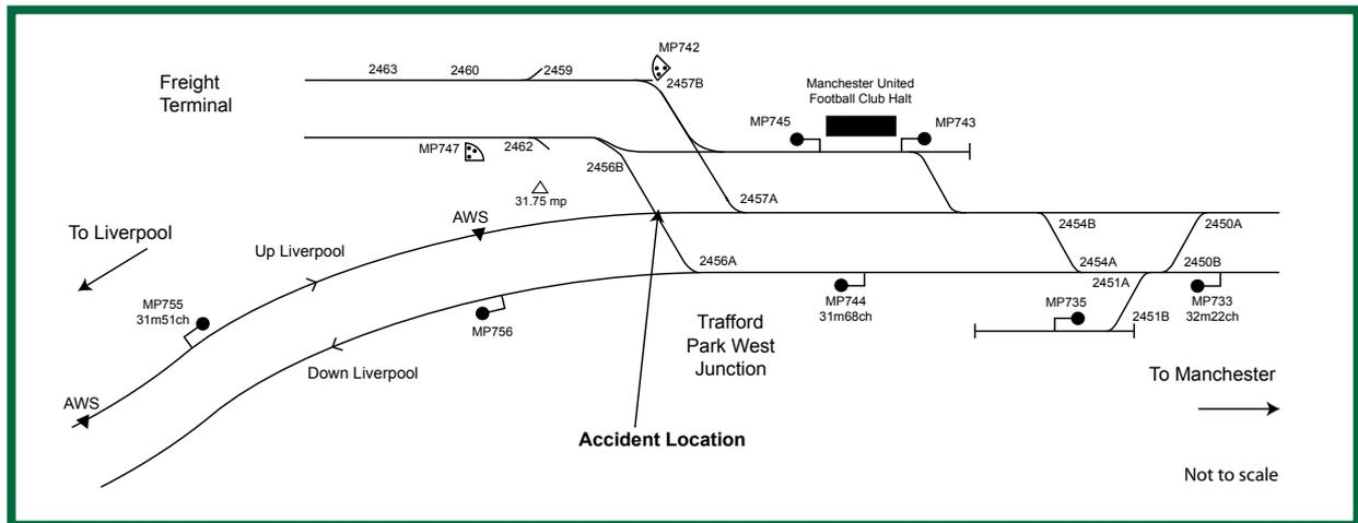
Figure 3: Track layout at the accident site
