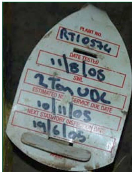
Figure 7: Bull tag on the incident trolley. This correctly indentifies the 3 month service date and incorrectly shows the annual inspection date as 2005
