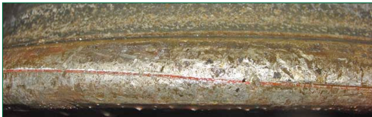
Figure 14: Cross contamination samples and flange climb marks (shown in red) on trolley wheel and Haughhead Junction number 58 points blade
