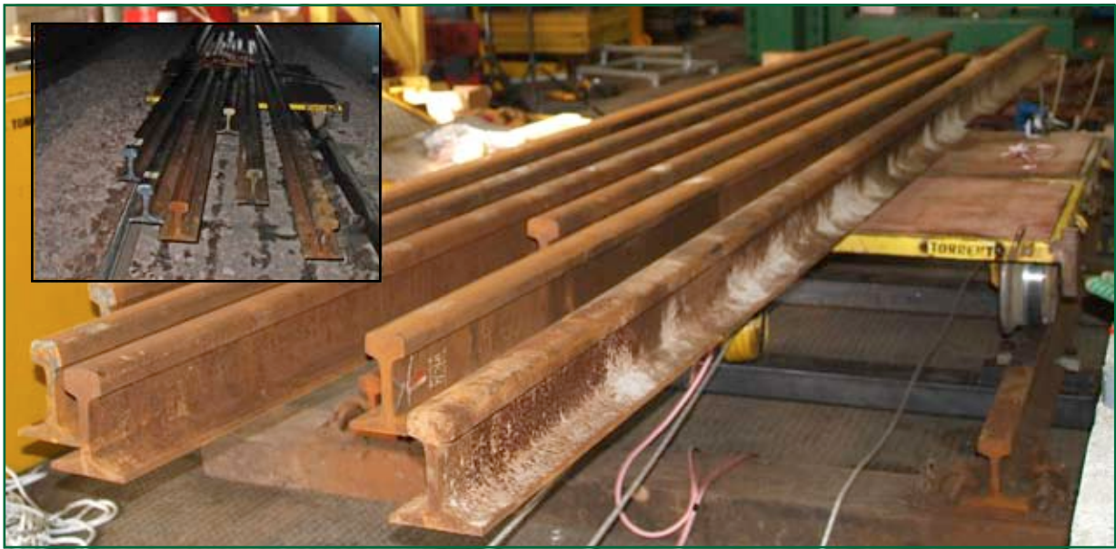
Figure 6: The incident trolley showing rails and relationship to 'as found' condition in Barncluith Tunnel
