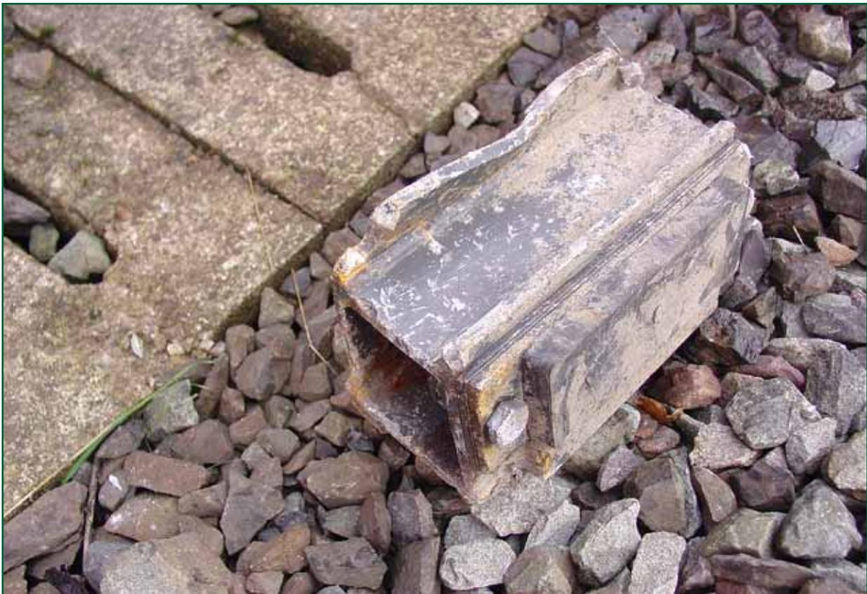
*Figure 11: Coupler lateral bump stop in the 'as found' condition*
