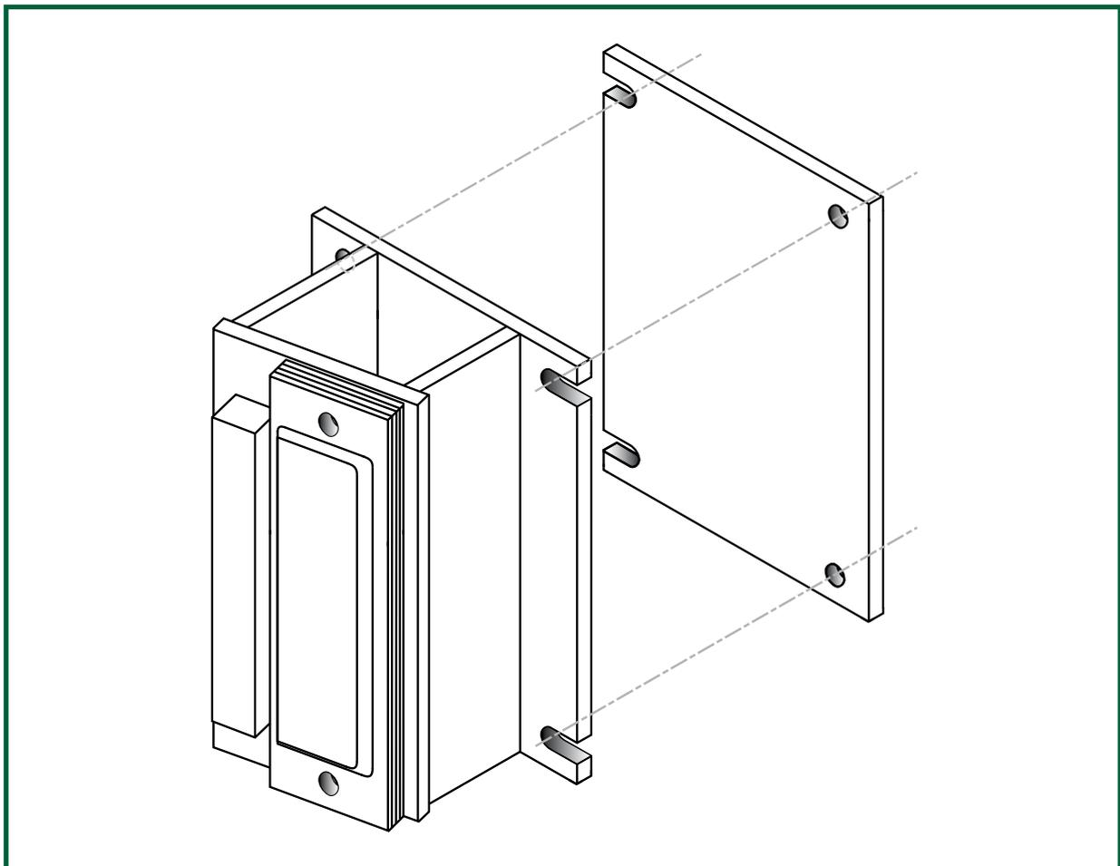
Figure 9: Class 175 coupler lateral bump stops
