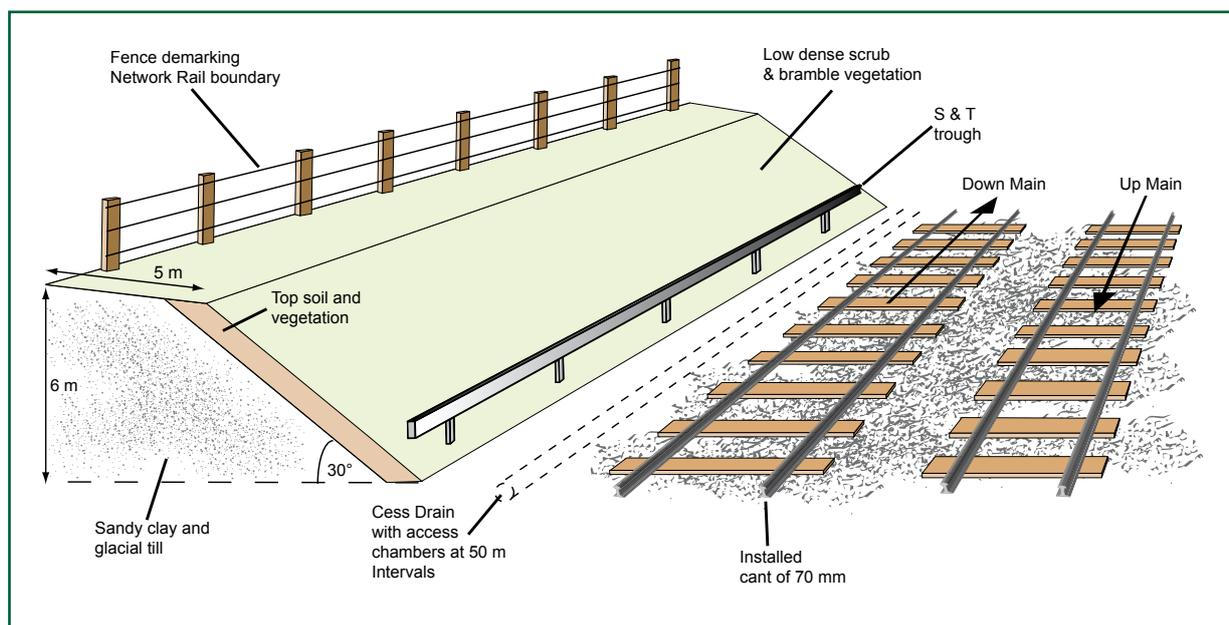
Figure 2: Diagrammatic presentation of the cutting slope prior to failure
