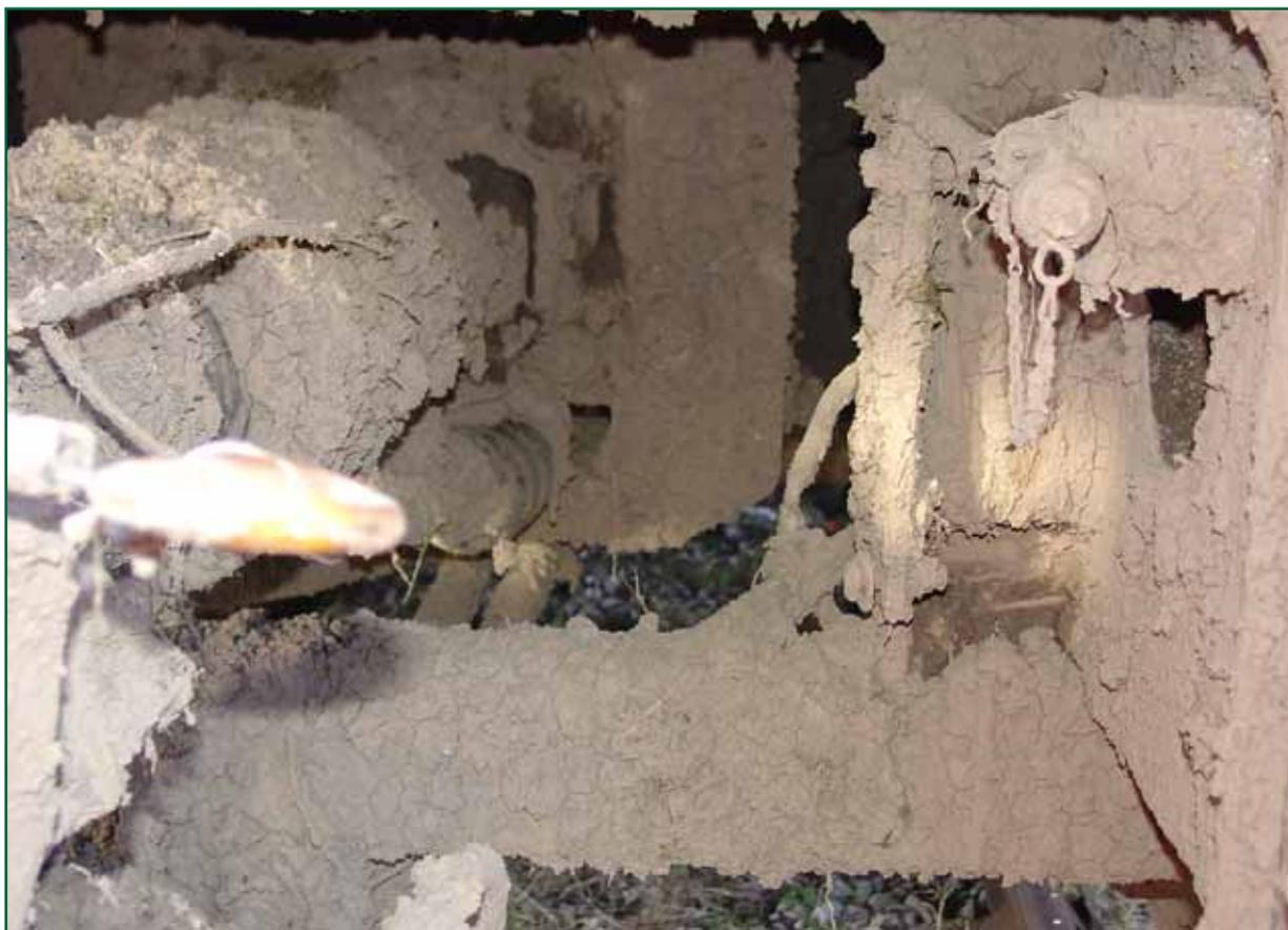
Figure 12: Coupler pocket following passage through landslip
