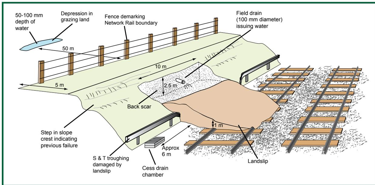
Figure 7: Cutting slope after landslide
