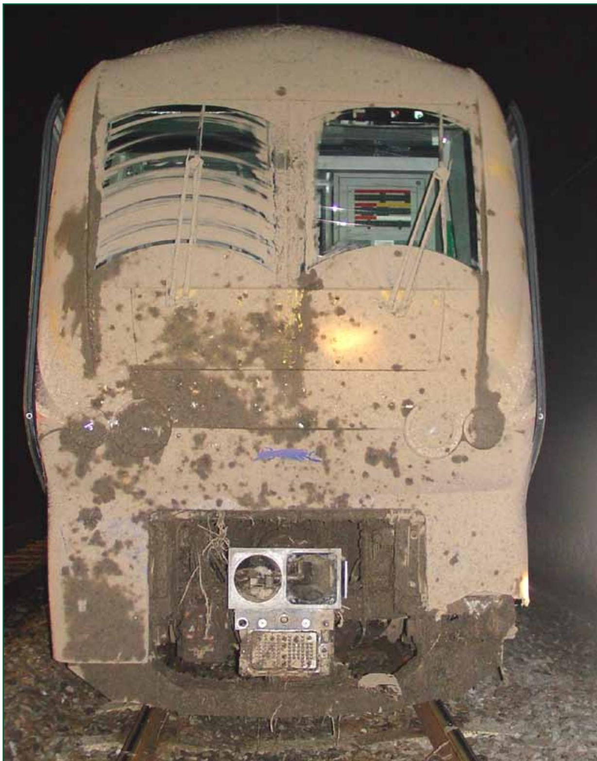
*Figure 8: Exterior of the vehicle following derailment*
