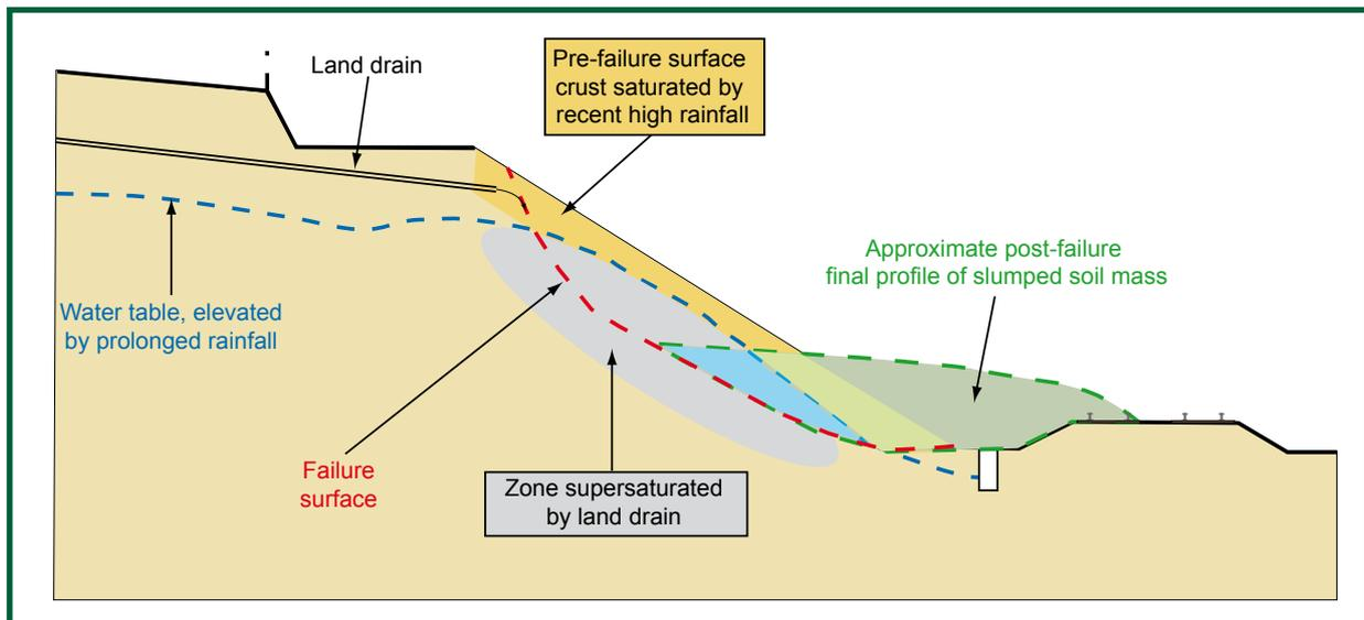
Figure 10: Sketch section through the failed cutting slope
