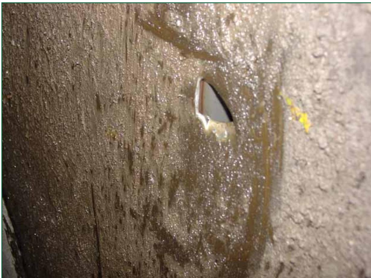
Figure 3: Hole in fuel tank
