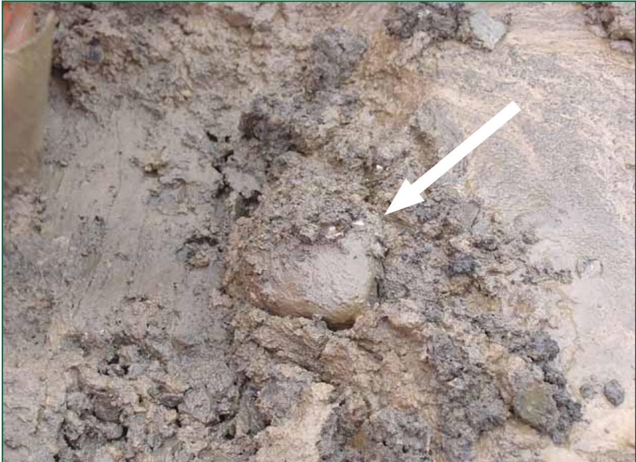
Figure 6: Indication of consistency and boulders in the landslide material
