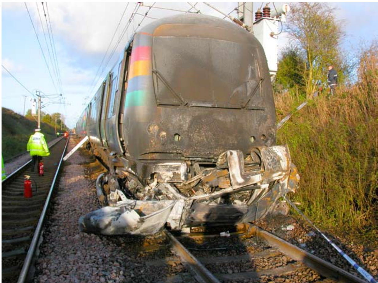
Figure 2: Damage caused to class 170 170207 as a result of the collision (courtesy of Norfolk Police)
