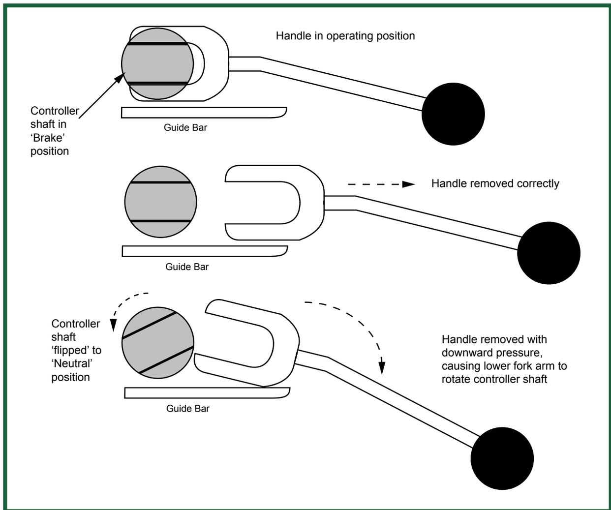
Figure 9: Removal of handle and 'flipping' of controller shaft
