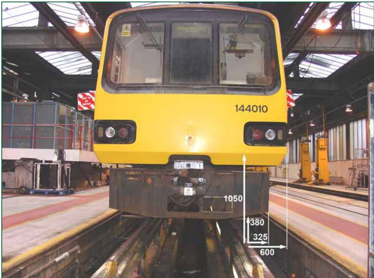
Figure 8: A class 144 DMU showing measured dimensions (mm) from the rail
