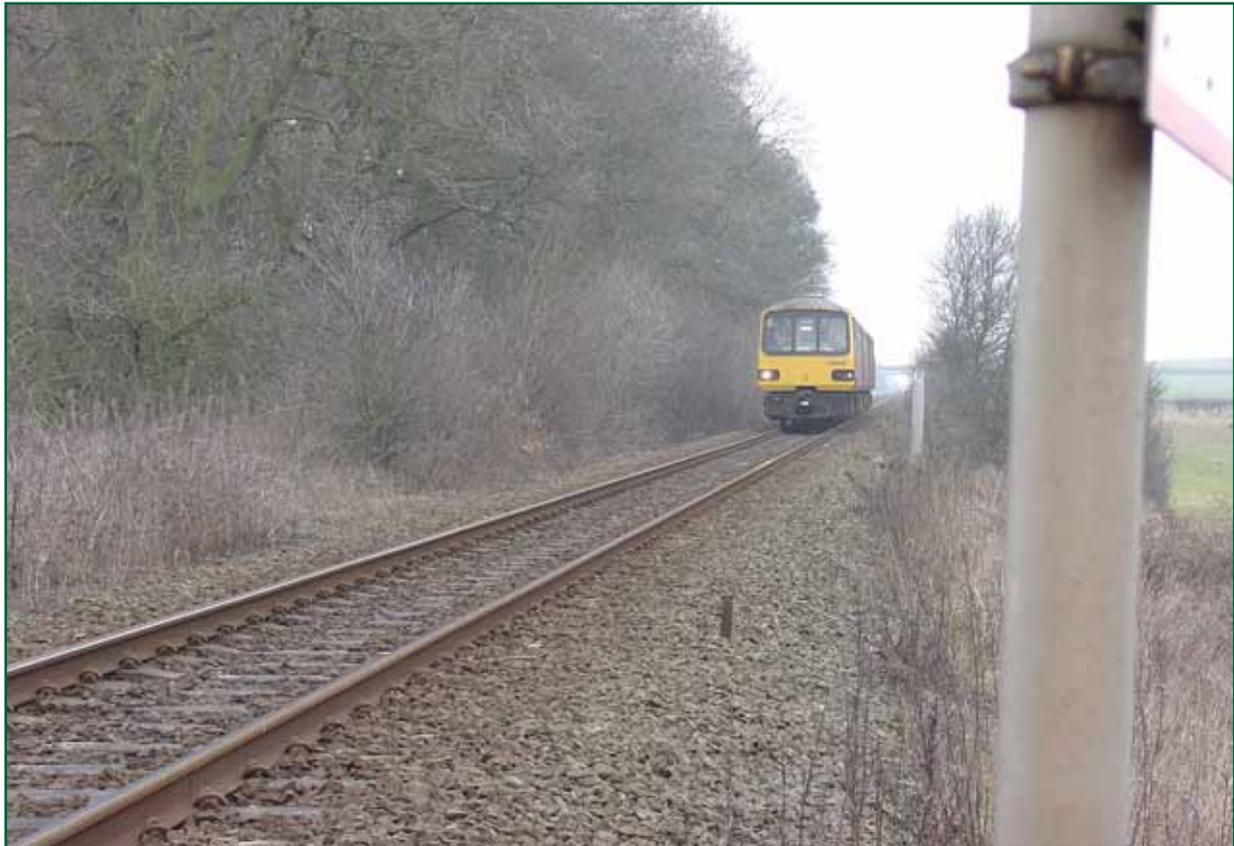
*Figure 11: A class 144 DMU approaching the crossing in daylight – approximately 80 m and 4 seconds from the crossing*
