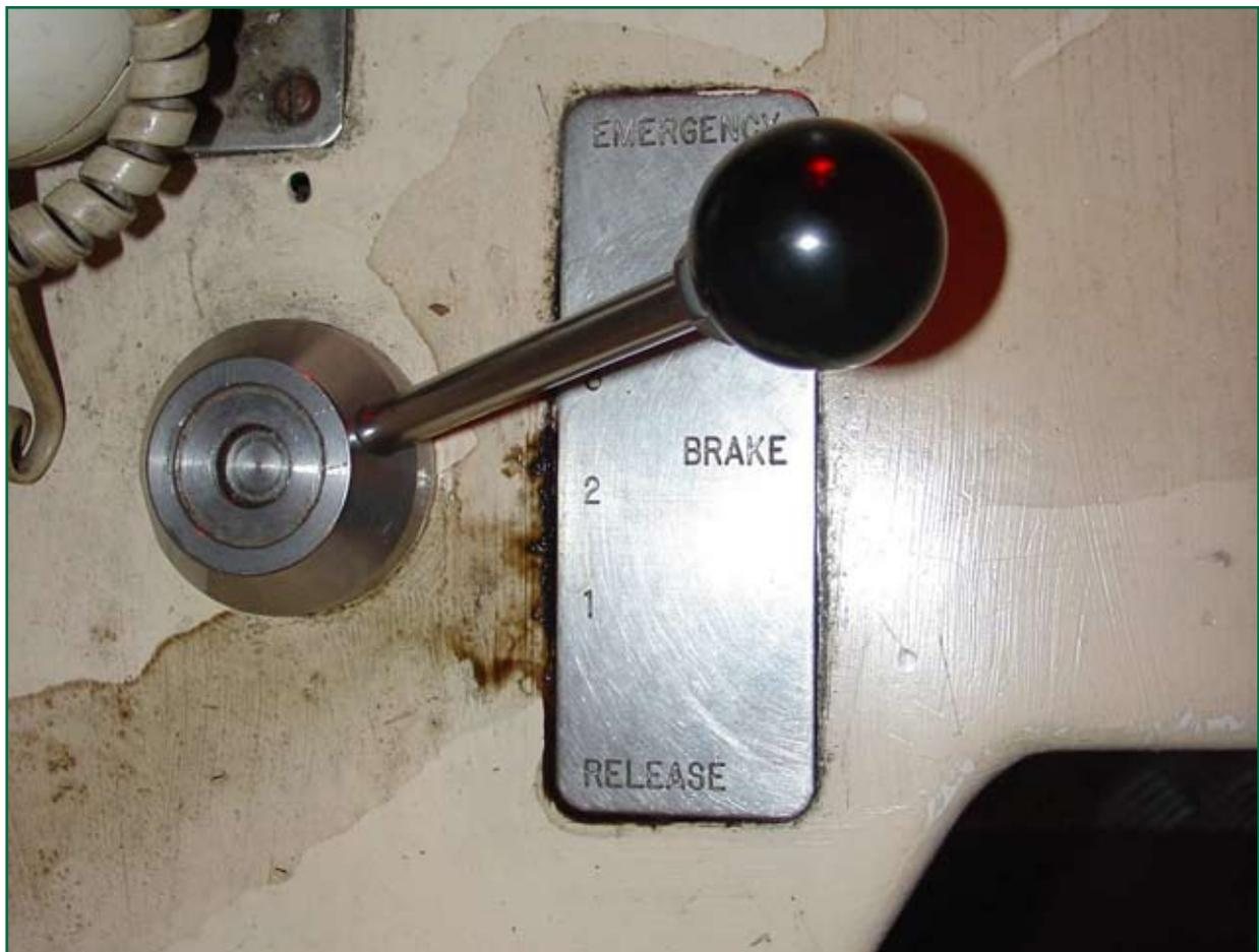
Figure 10: Brake control handle
