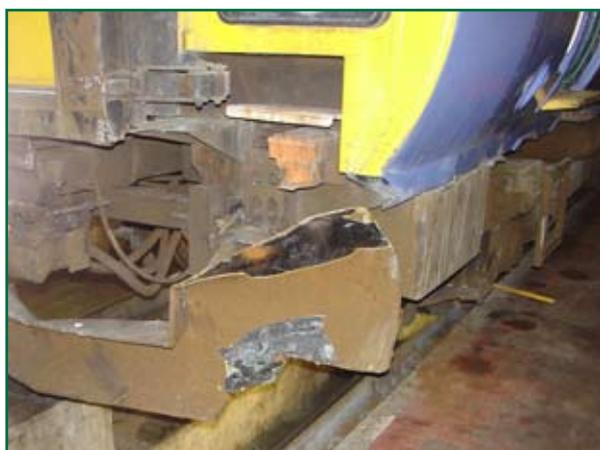
*Figure 16: Damage to 57422 (left-hand side)*
