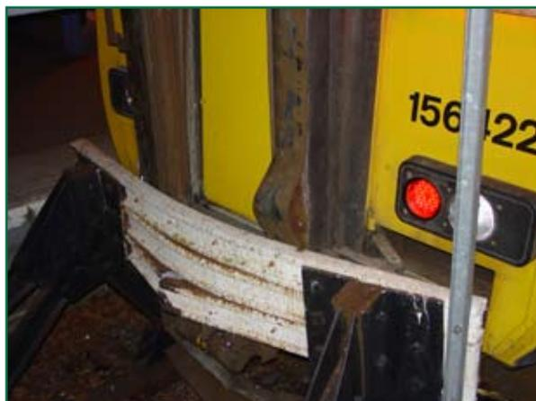
*Figure 15: Damage to buffer stop with 57422 in its final position*
