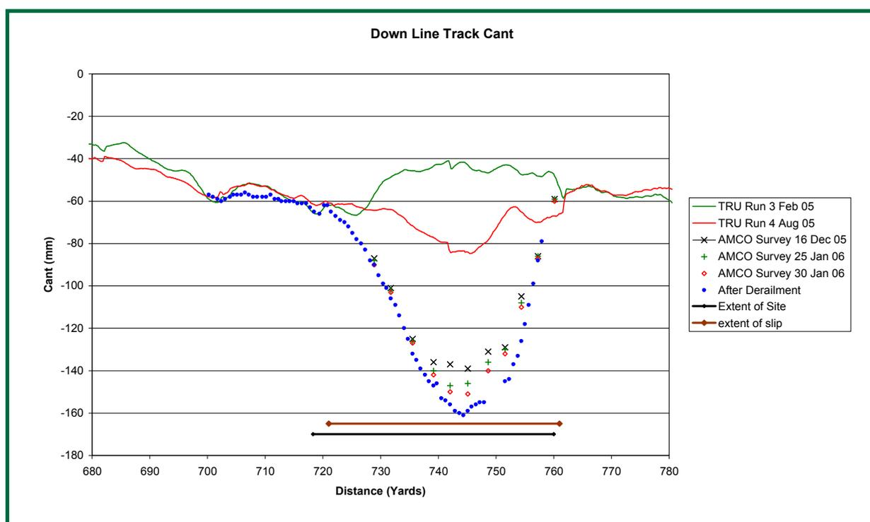
Figure 7: Track cant plotted against distance over time.
