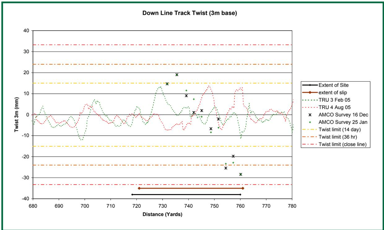
Figure 8: Track twist plotted against distance.
