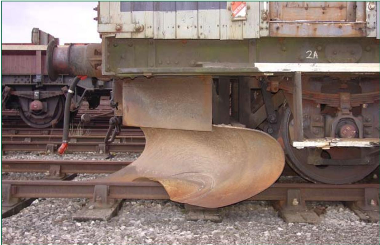
Figure 3: Detailed view of the ballast plough
