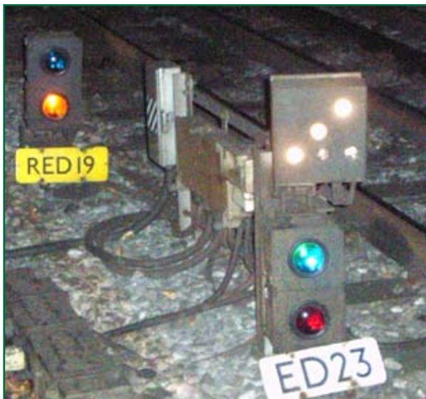
Figure 11: Signal ED23 showing route to terminal Platform 3
