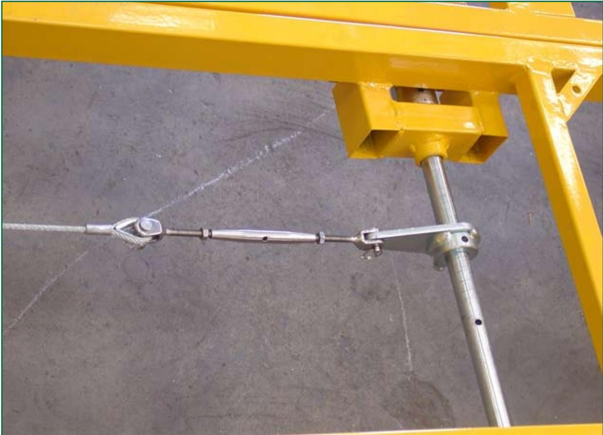
Figure 5: A Rotamag slack adjuster.
