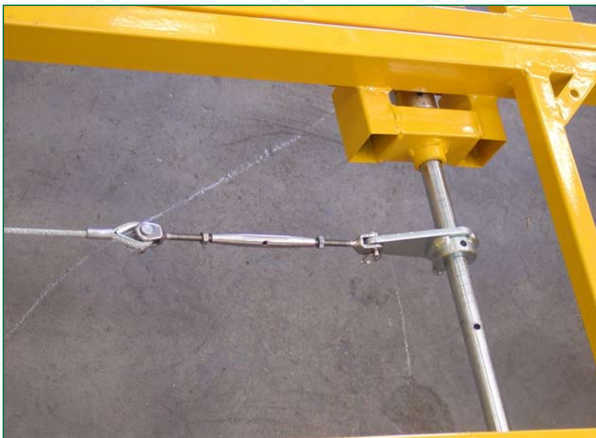
Figure 5: A Rotamag slack adjuster.
