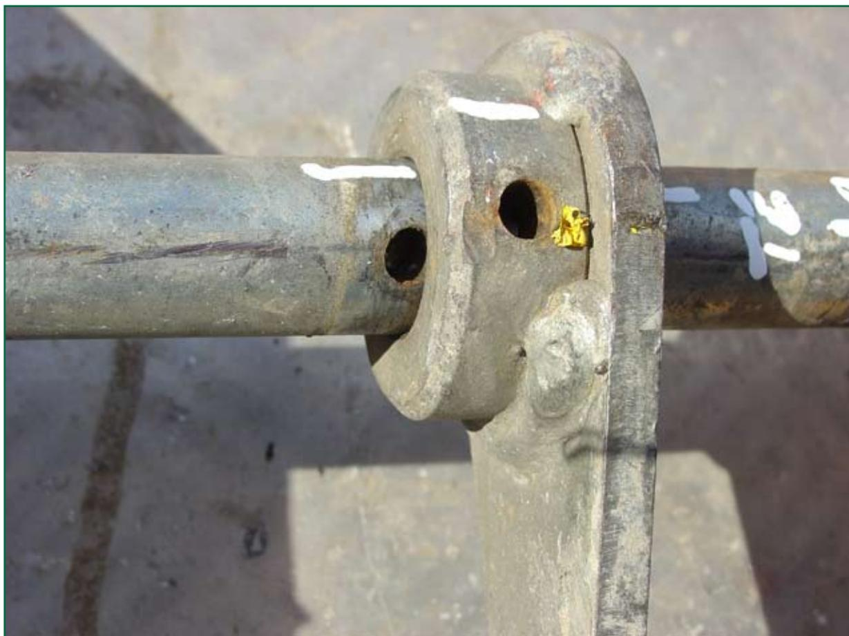
Figure 7: Detail of the release arm boss.
