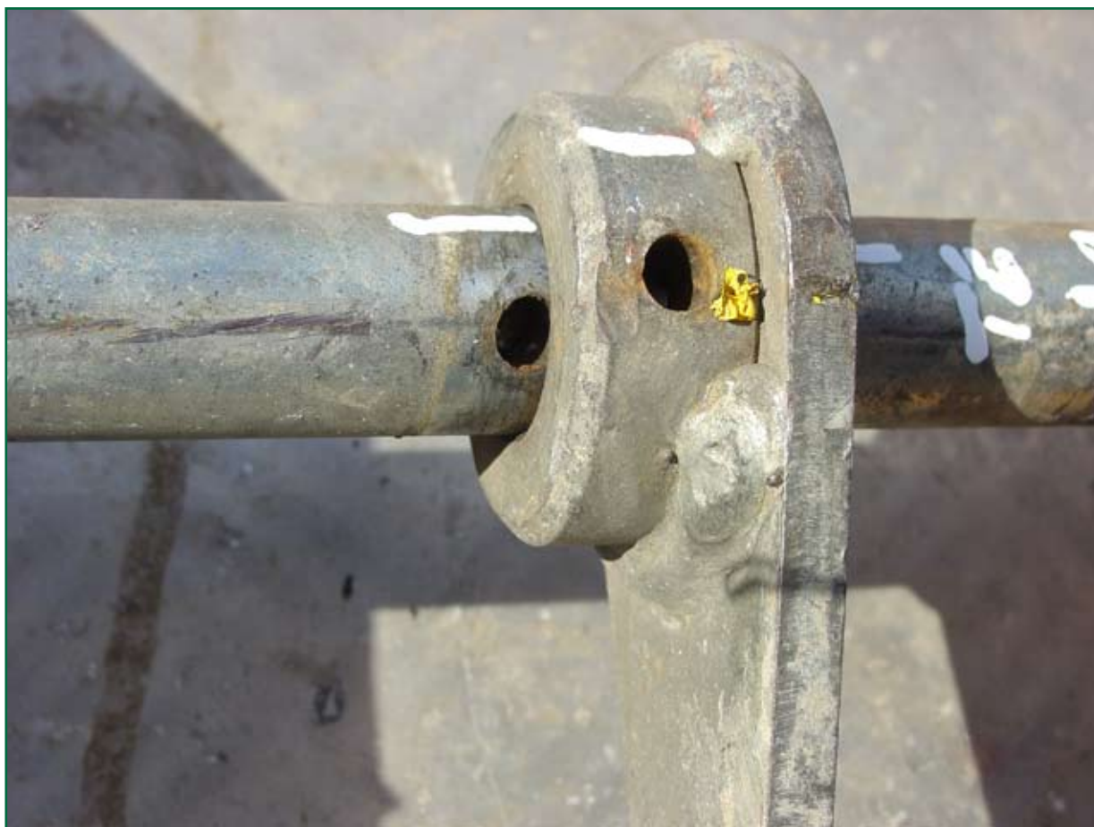
Figure 7: Detail of the release arm boss.
