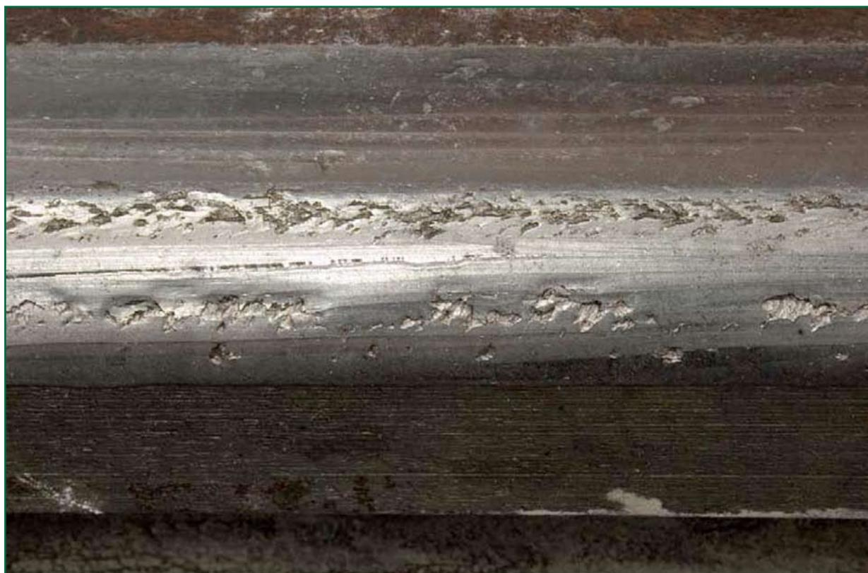
Figure 10: Rolling contact fatigue marks on the switch rail, overlaid by wear on the gauge corner.
