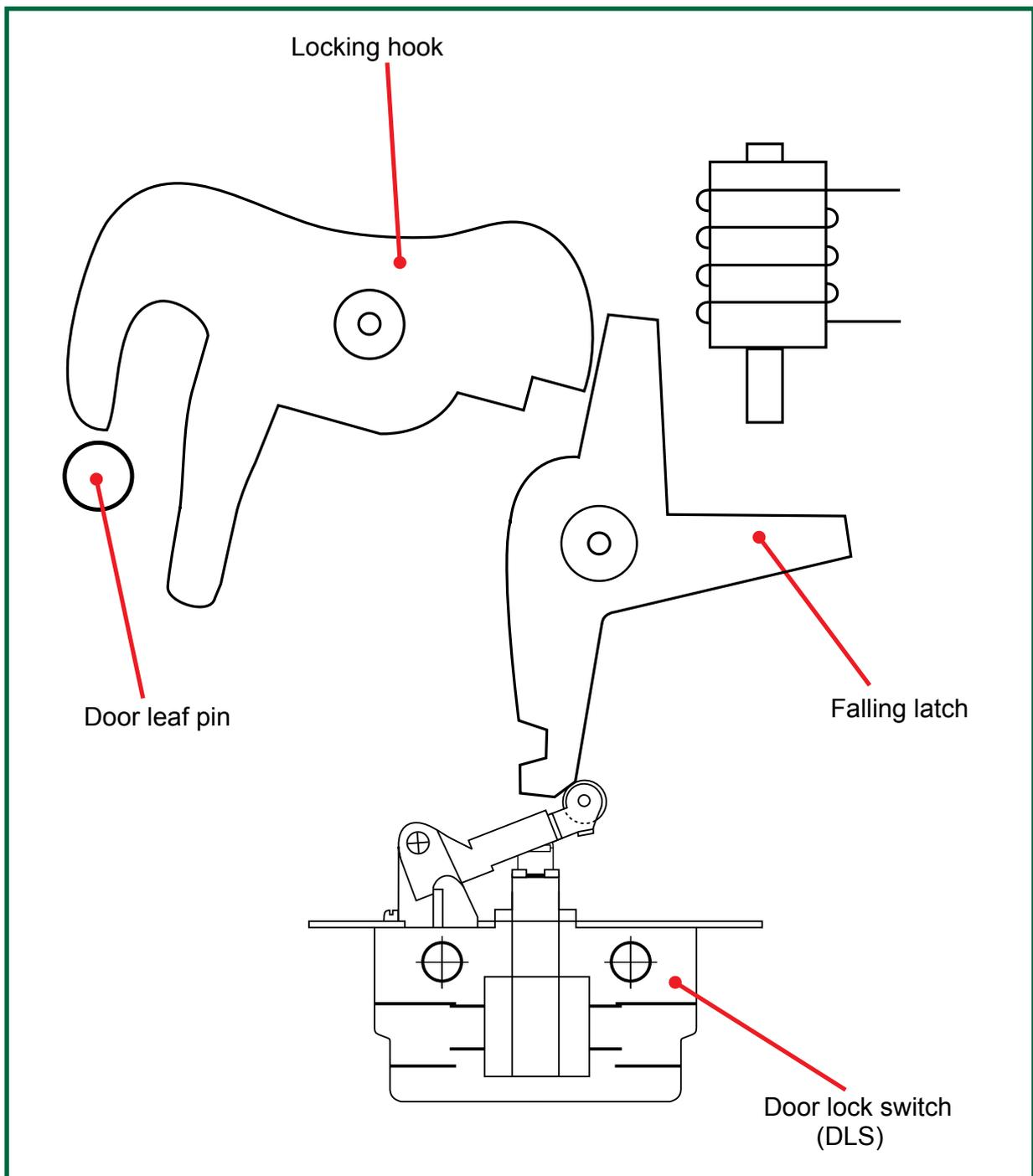
Figure 9: Door locking mechanism in unlocked state
