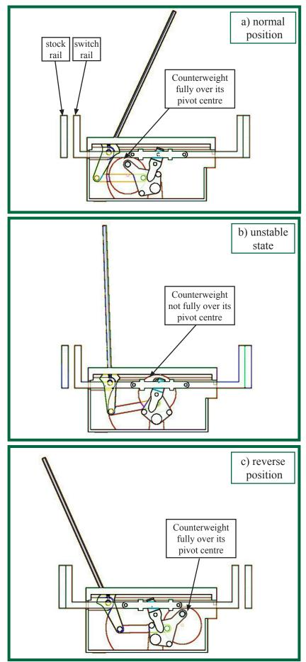
Figure 7: The hand points mechanism under operation
