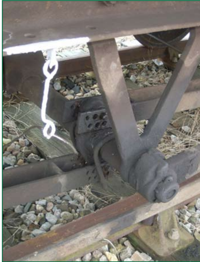
Figure 8: Adjustment of the push rod on ZBA type wagons
