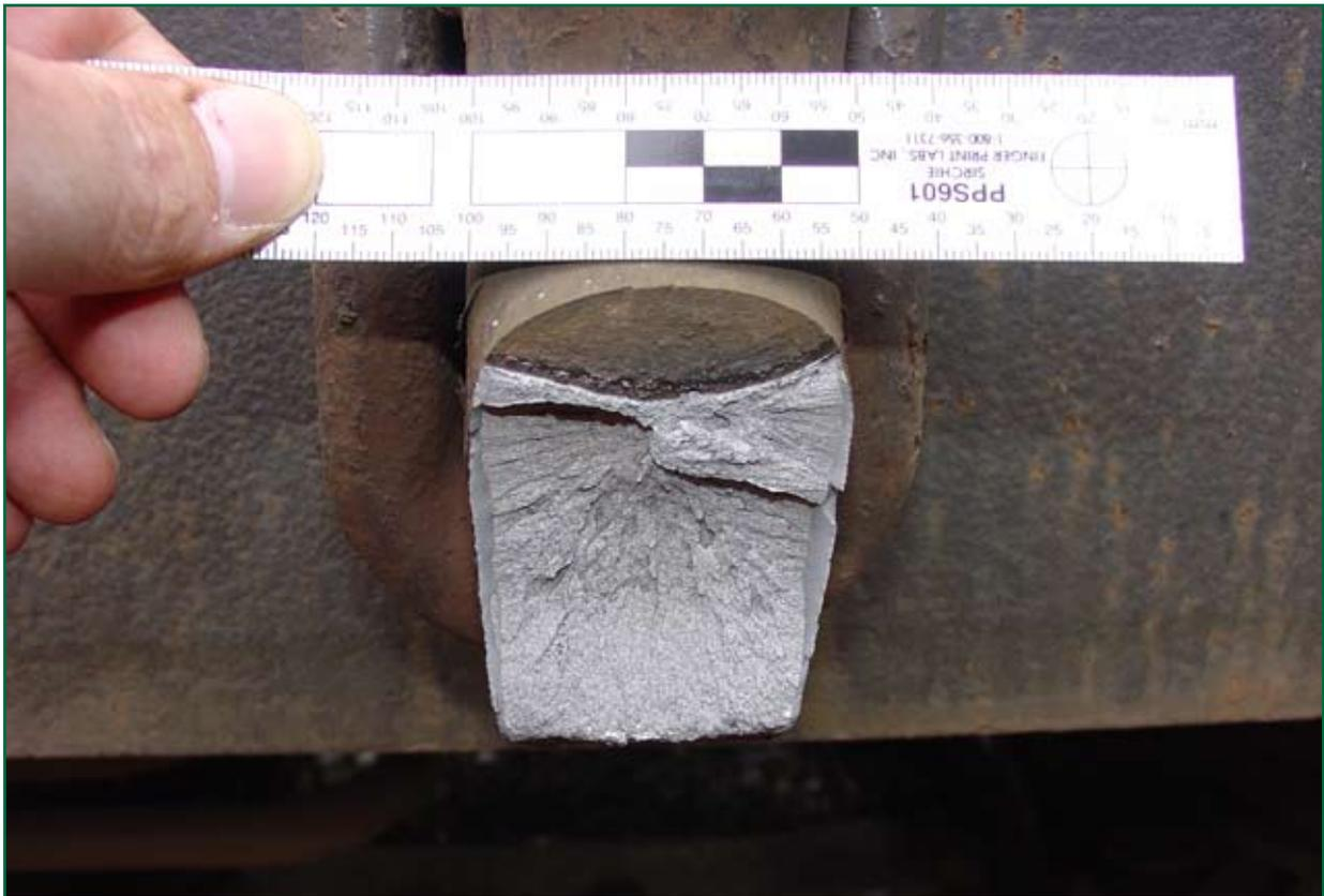
Figure 5: Wagon drawhook fracture face
