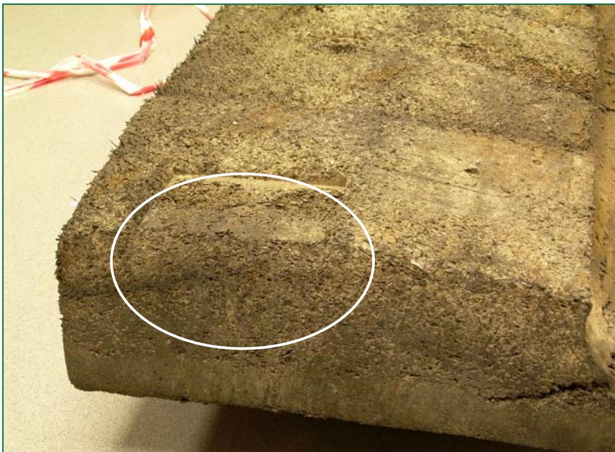
*Figure 29: Panel B4 underside showing wear on panel edge in the base plate location area*
