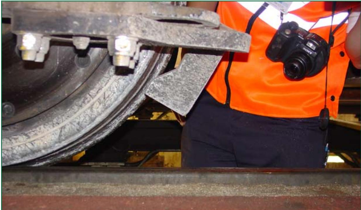
Figure 11: Distorted lifeguard on leading right-hand (six foot) side of derailed train
