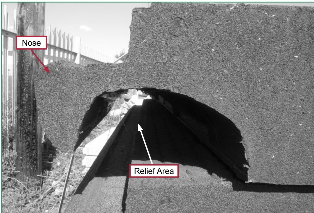
Figure 15: End view of panel nose area
