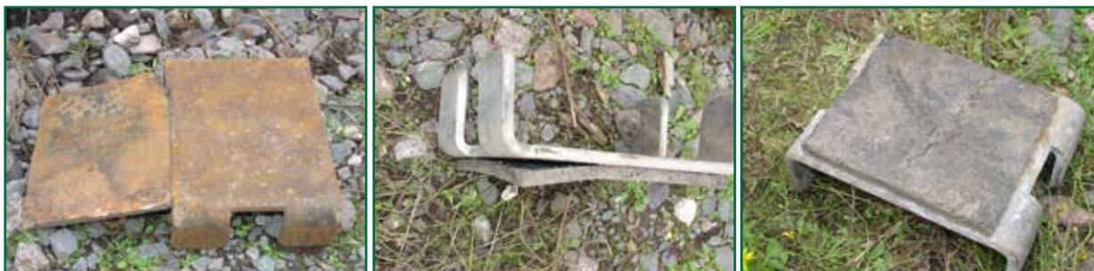
Figure 33: Loss of and damage to base plate pads
