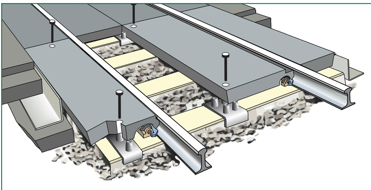
Figure 17: First version of base plate with threaded bosses
