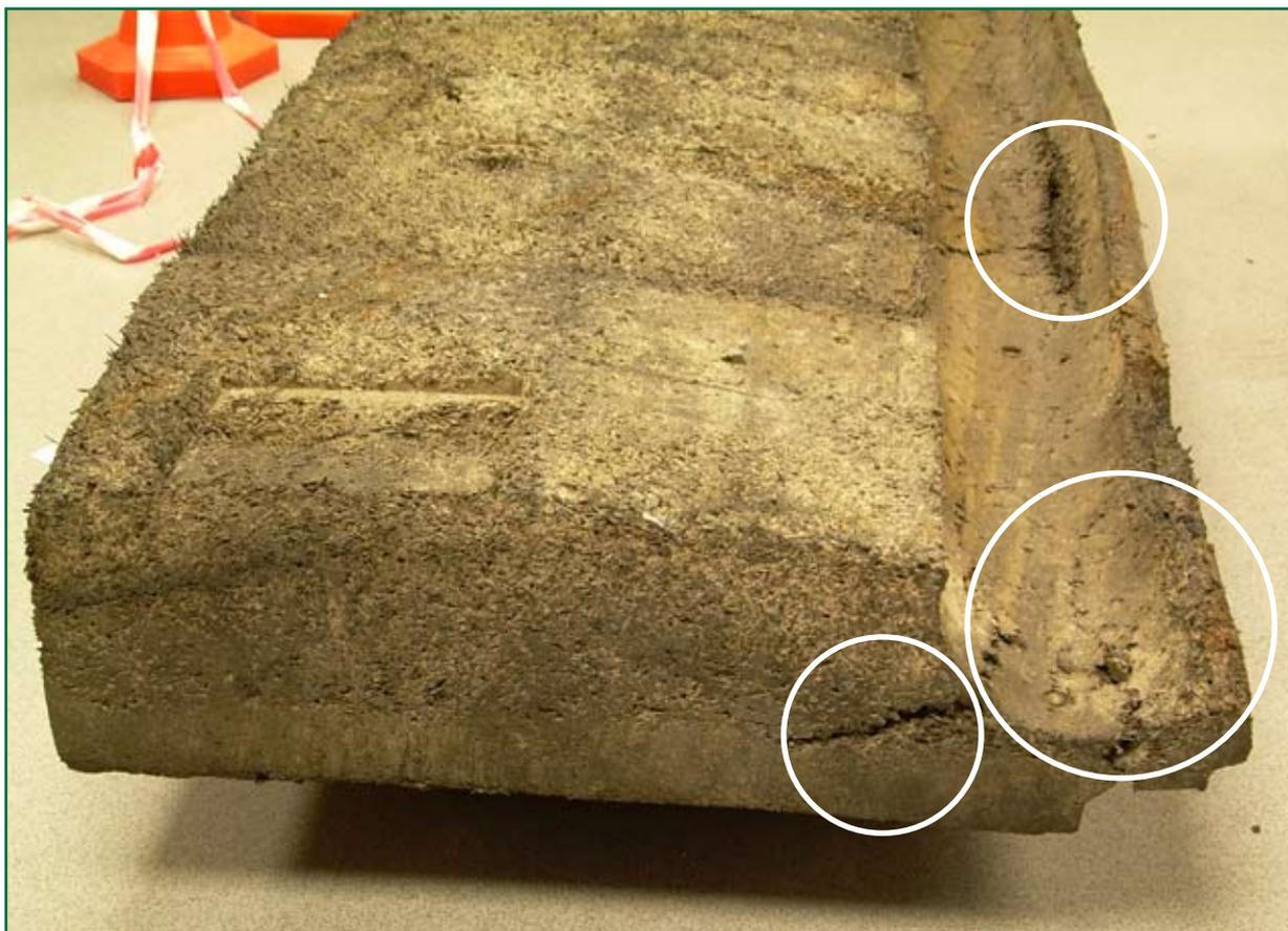
Figure 26: Panel B4 underside showing cracking in relief area and damage to nose
