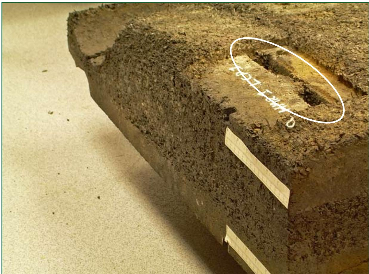
Figure 28: Panel B4 underside showing wear and cracking in the base plate location area
