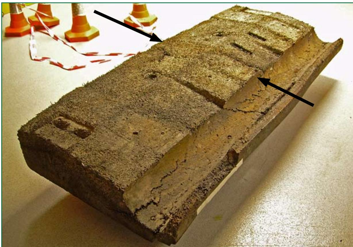
Figure 27: Panel B4 underside showing indentations from sleepers and transverse crack (arrowed)
