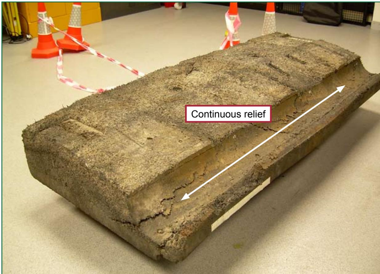
Figure 13: Continuous relief area on underside of panel B4
