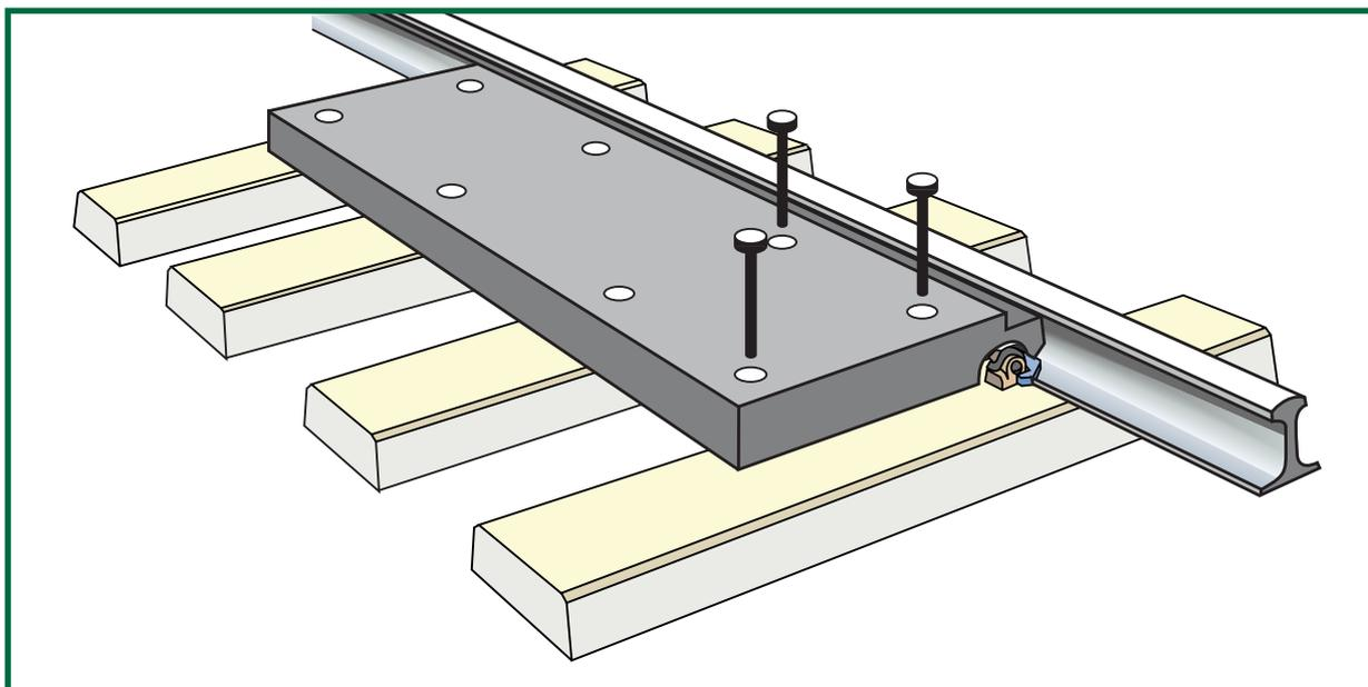
Figure 16: Original screw fixing of panels to timbers
