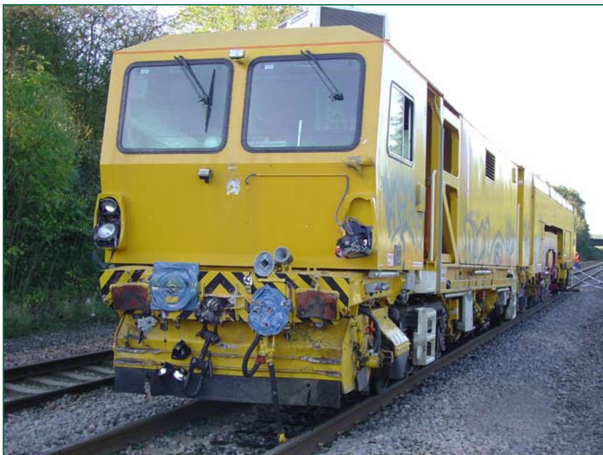
Figure 2: The tamper after the collision, showing damage to the front end
