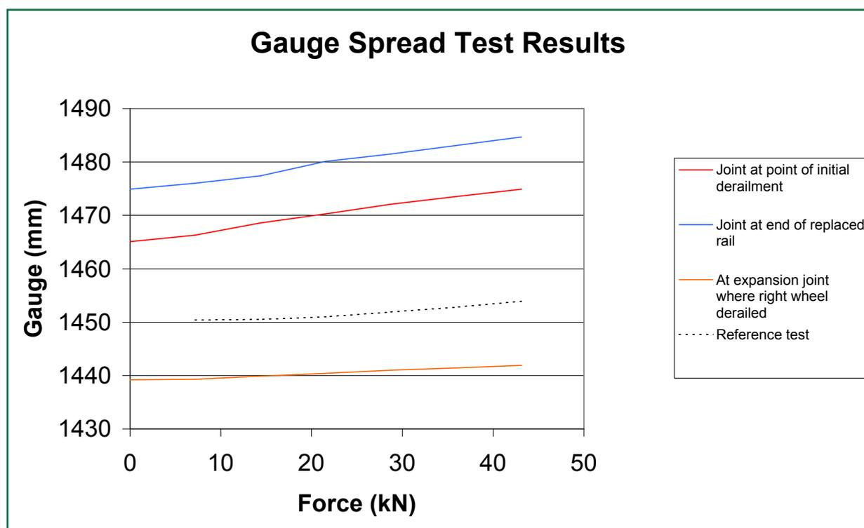
Figure 8: Gauge spread bar tests
