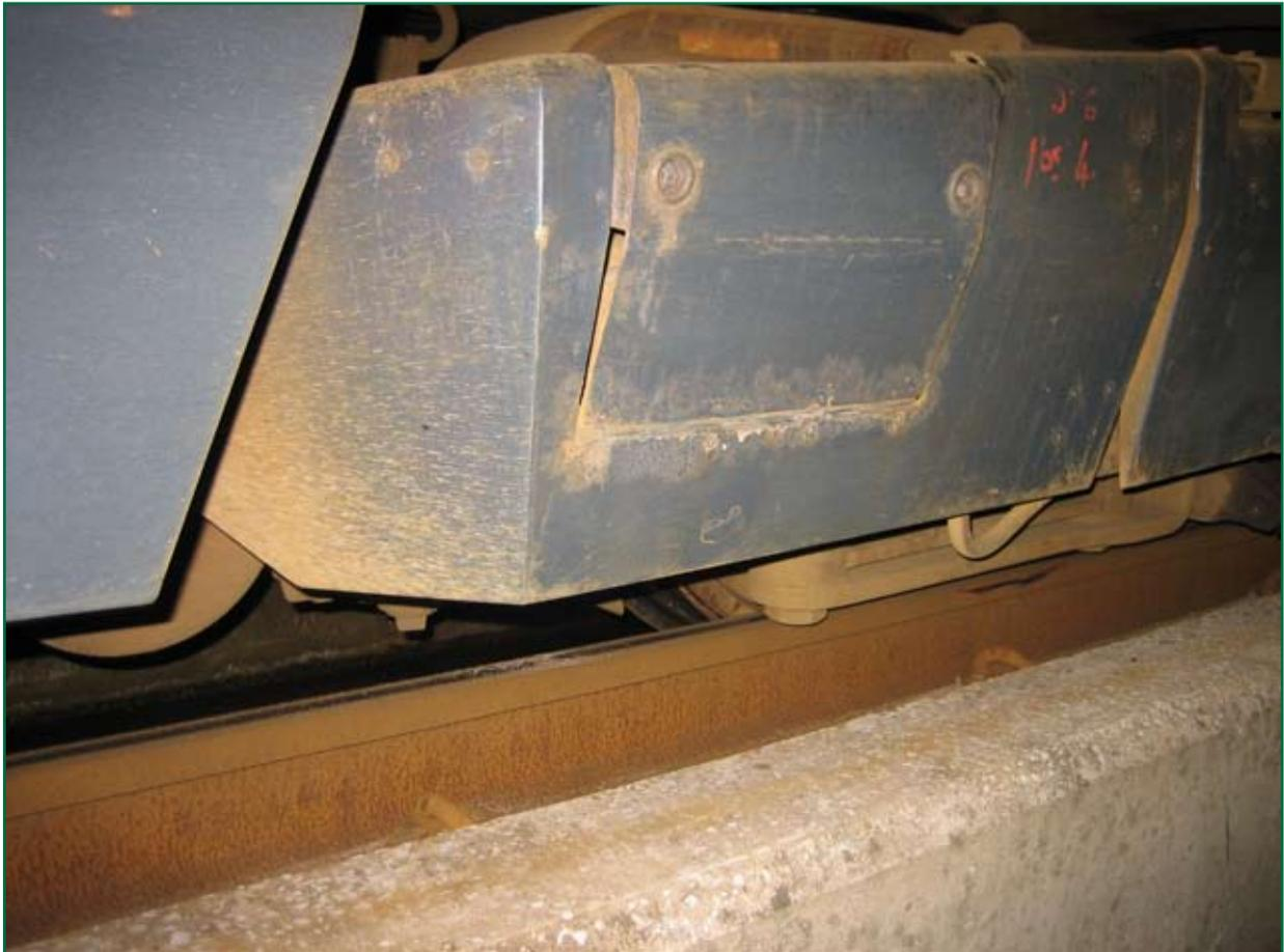
Figure 3: Derailed wheel at front left-hand side of tram
