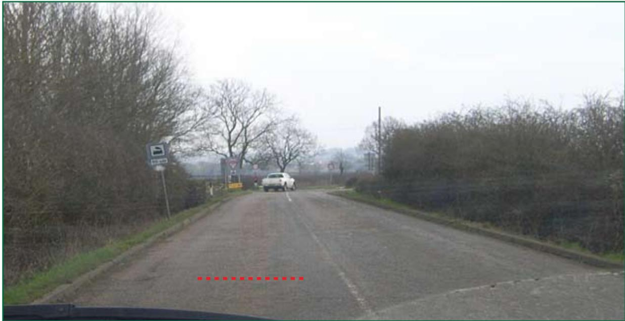
*Figure 2: View approaching Shenley Hill Road level crossing from North to South. A vehicle can be seen in space between the two give way areas waiting to turn right onto Mile Tree Road. The red line indicates the location, 40 m from the junction when the train can be partially seen from the left-hand side (LHS) in the direction of travel*
