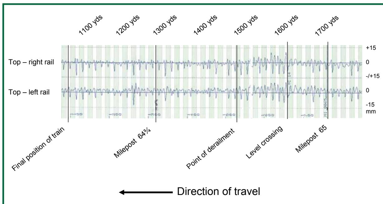
Figure 6: Track recording coach output for area of derailment on 26 August 2006
