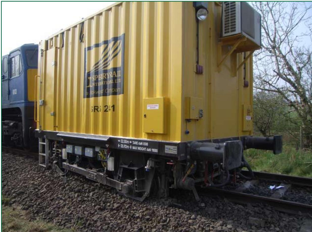
Figure 3: The Sperry ultrasonic test vehicle after the derailment
