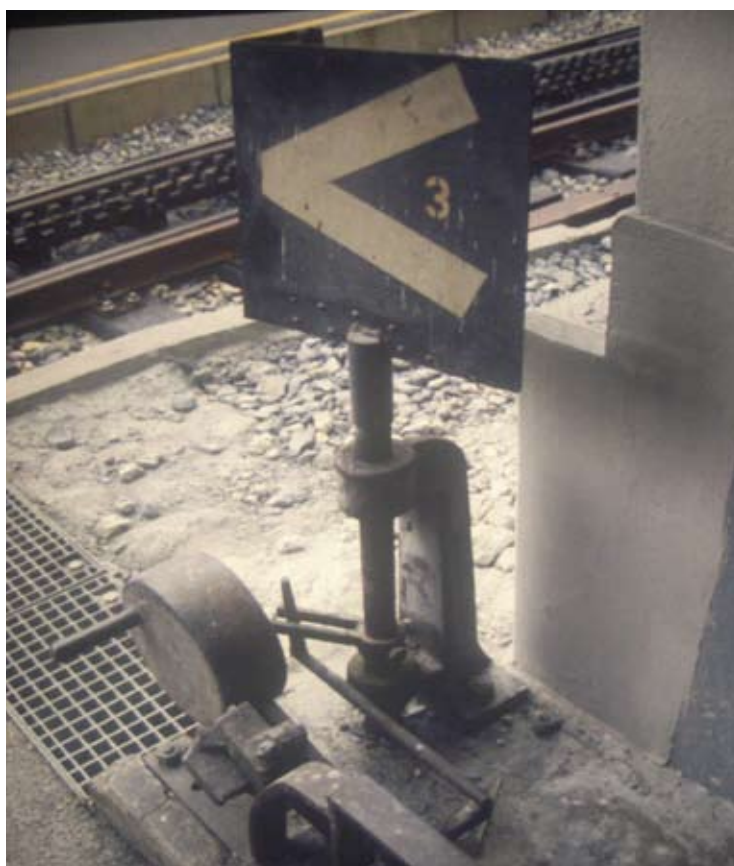
Figure 8: Point lever and indicator combined (photograph courtesy of private collection)
