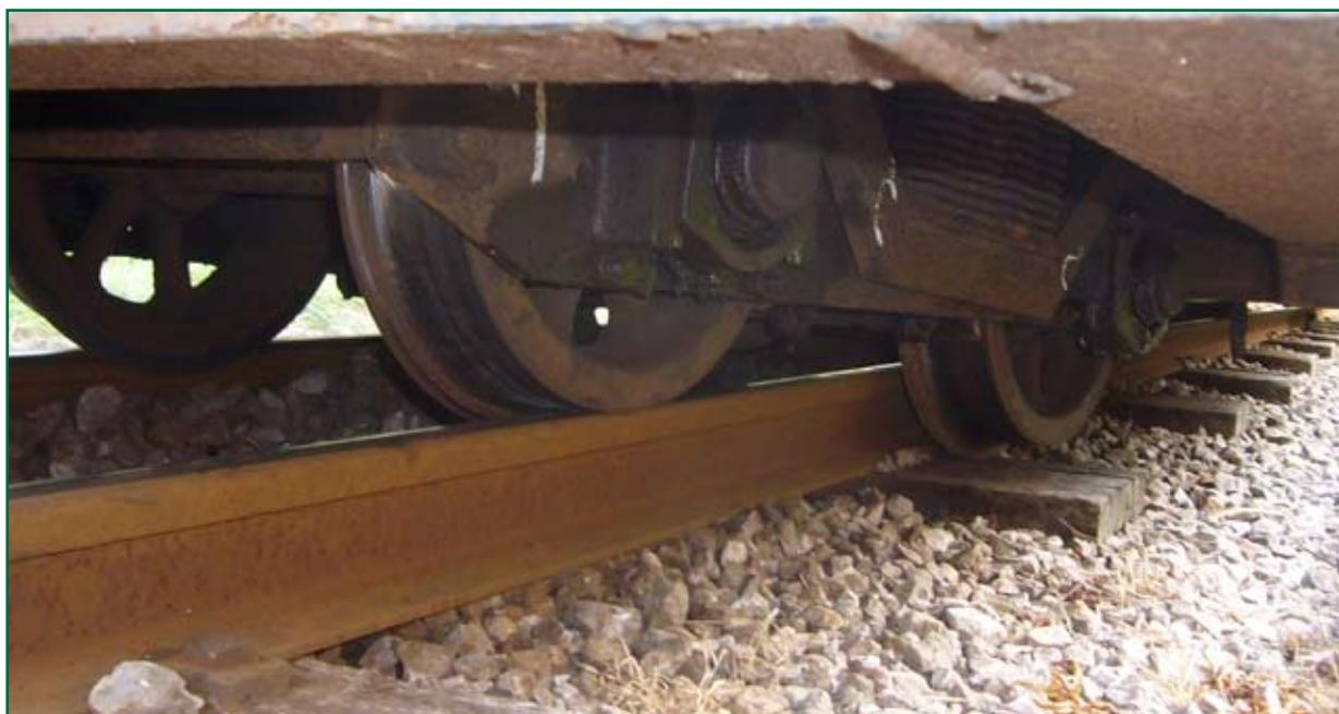
Figure 4: Derailed leading wheelset on trailing bogie of Maxi coach 131 on site at Hollin How (courtesy of R&ER)
