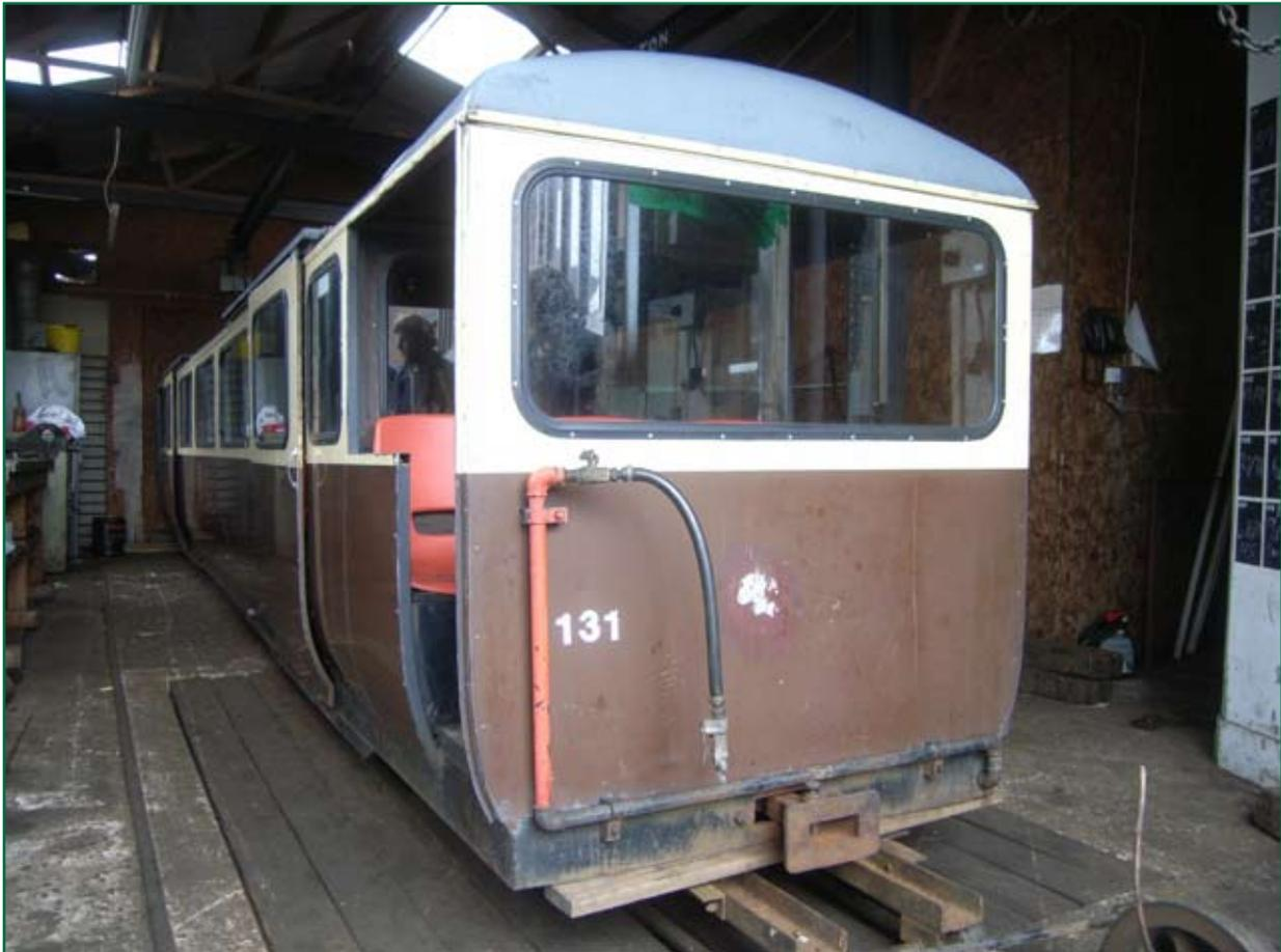
Figure 3: Maxi coach 131 with leading end (nearest) on skidder unit
