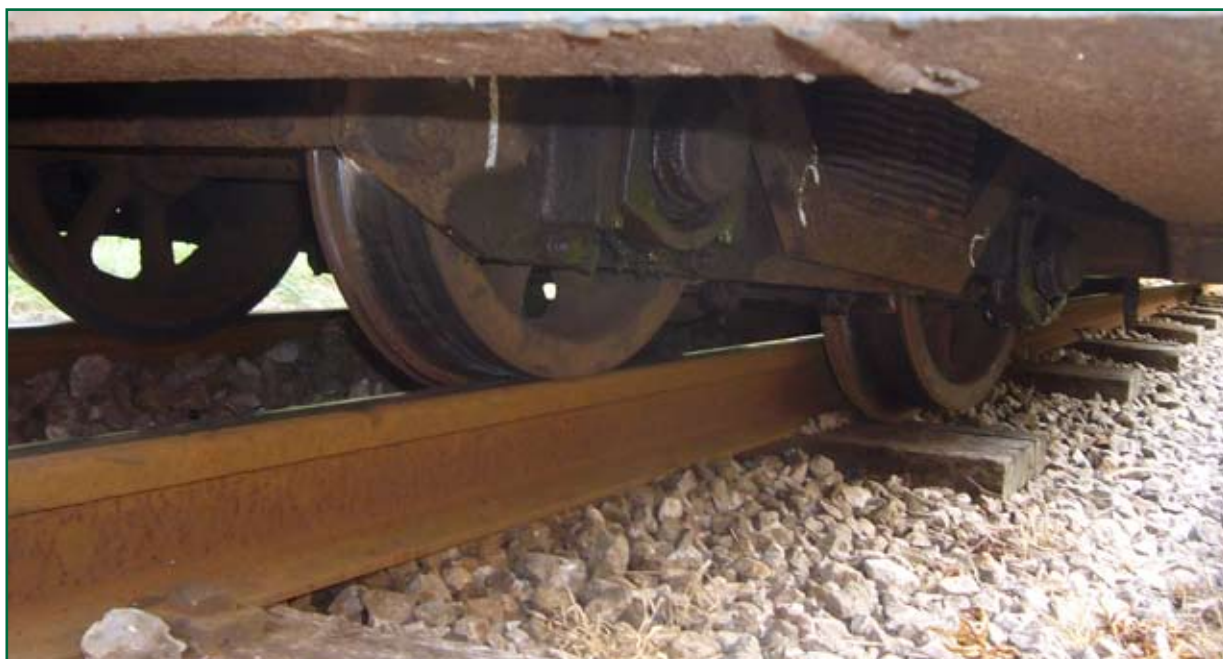
Figure 4: Derailed leading wheelset on trailing bogie of Maxi coach 131 on site at Hollin How (courtesy of R&ER)
