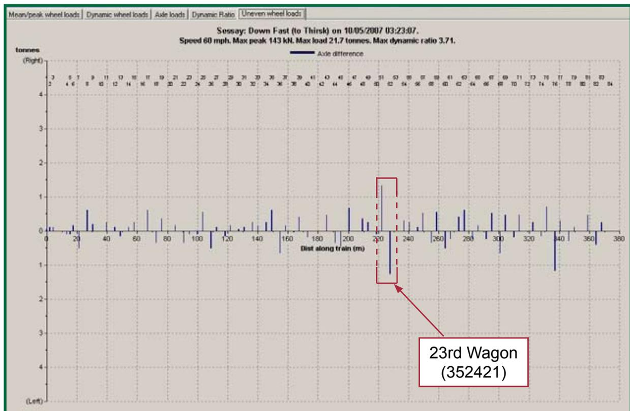
Figure 9: Uneven Wheel Load report for train 6S22
