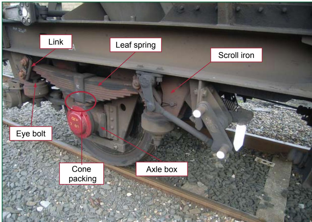
Figure 4: An HAA suspension arrangement
