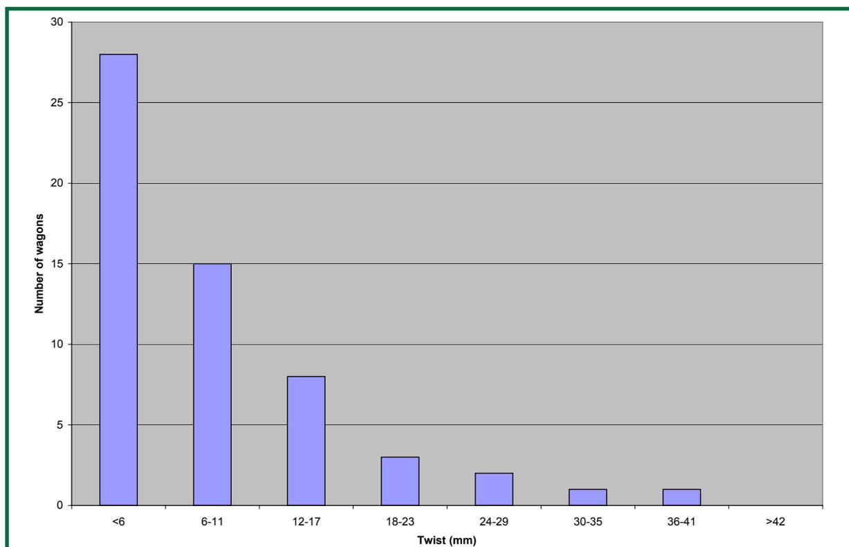
Figure 8: Results of the wagon frame twist survey
