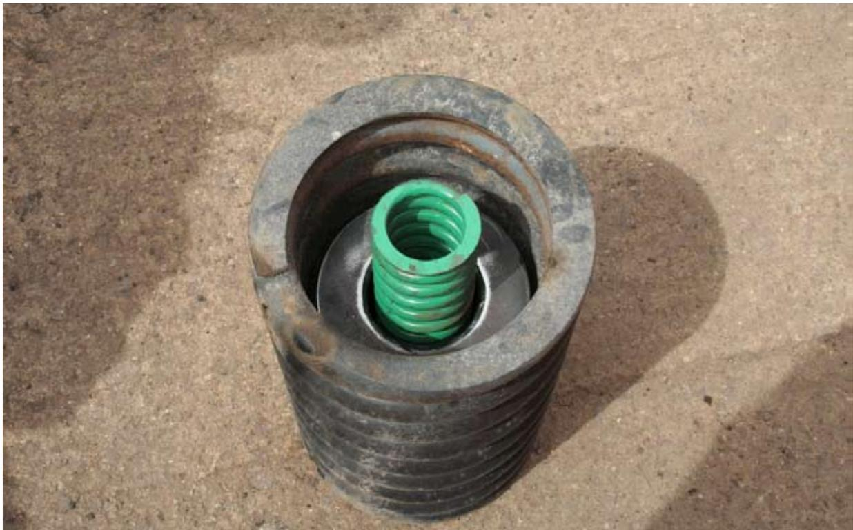
*Figure 31: Spring assembly showing primary, secondary and inner 'cup' spring sitting within the 'top hat' component. Inner cup spring is identical that found at Hawks user worked crossing*
