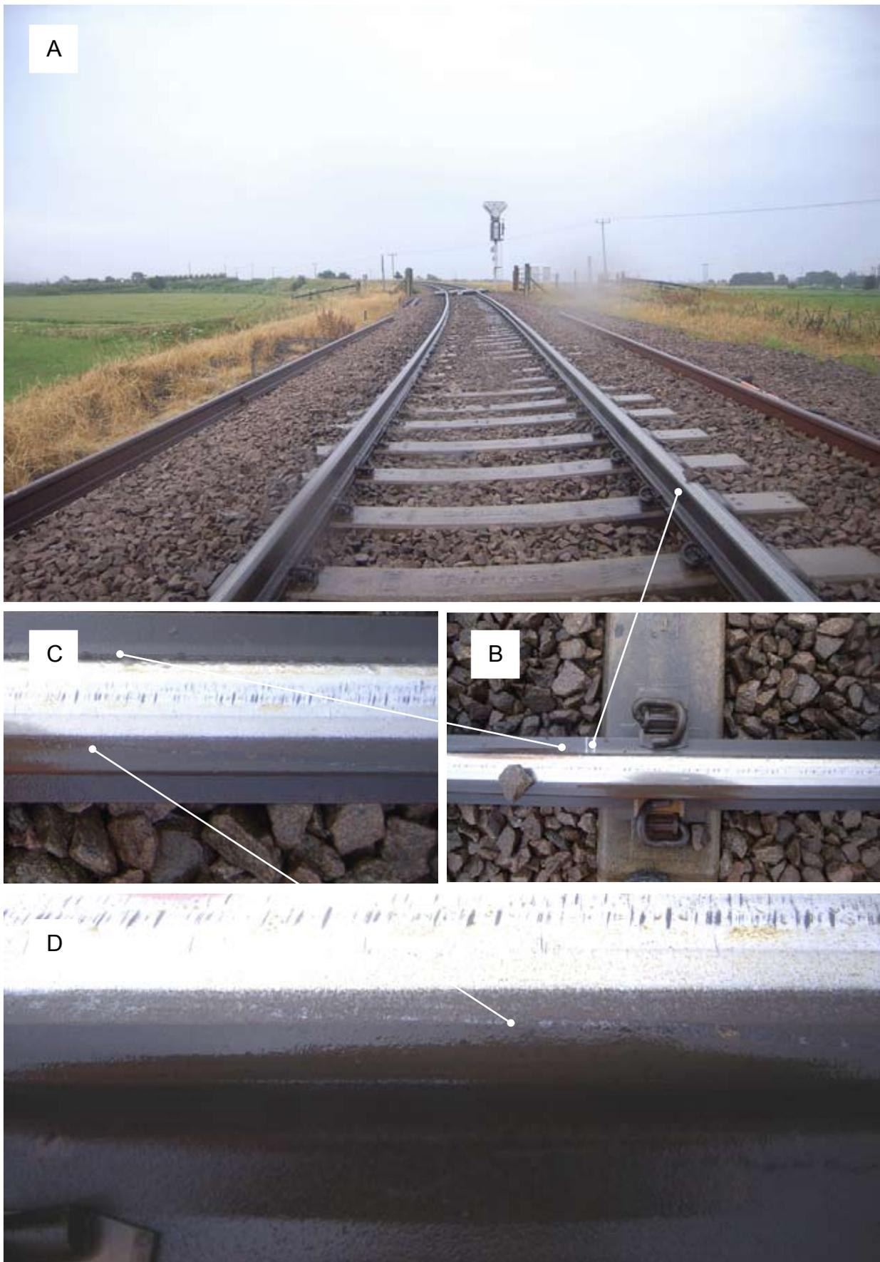
Figure 22: Sequence of images showing the area of flange climb (a), from the gauge corner onto the crown of the high right-hand rail (b & c) and the drop off mark (d)
