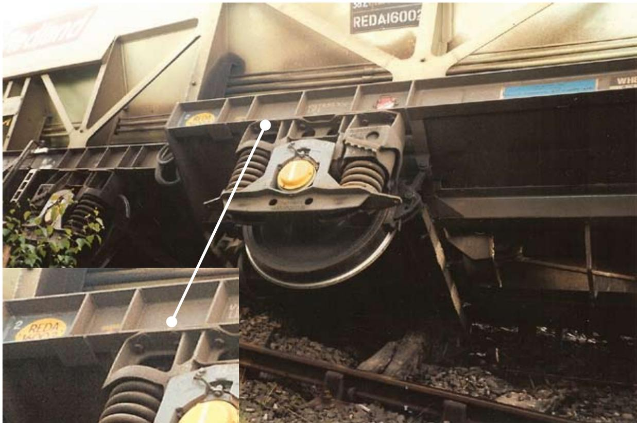
Figure 42: Detail of damage to vehicle REDA 16002 following Baguley Fold junction derailment. Inset shows no visible packing and no evidence of welding work
