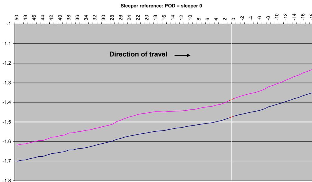
Figure 25: Diagram showing the twist features in track geometry from +50 sleepers to -19. High right-hand rail (magenta) and low left-hand rail (blue). Point of derailment marked at zero (paragraph 277)
