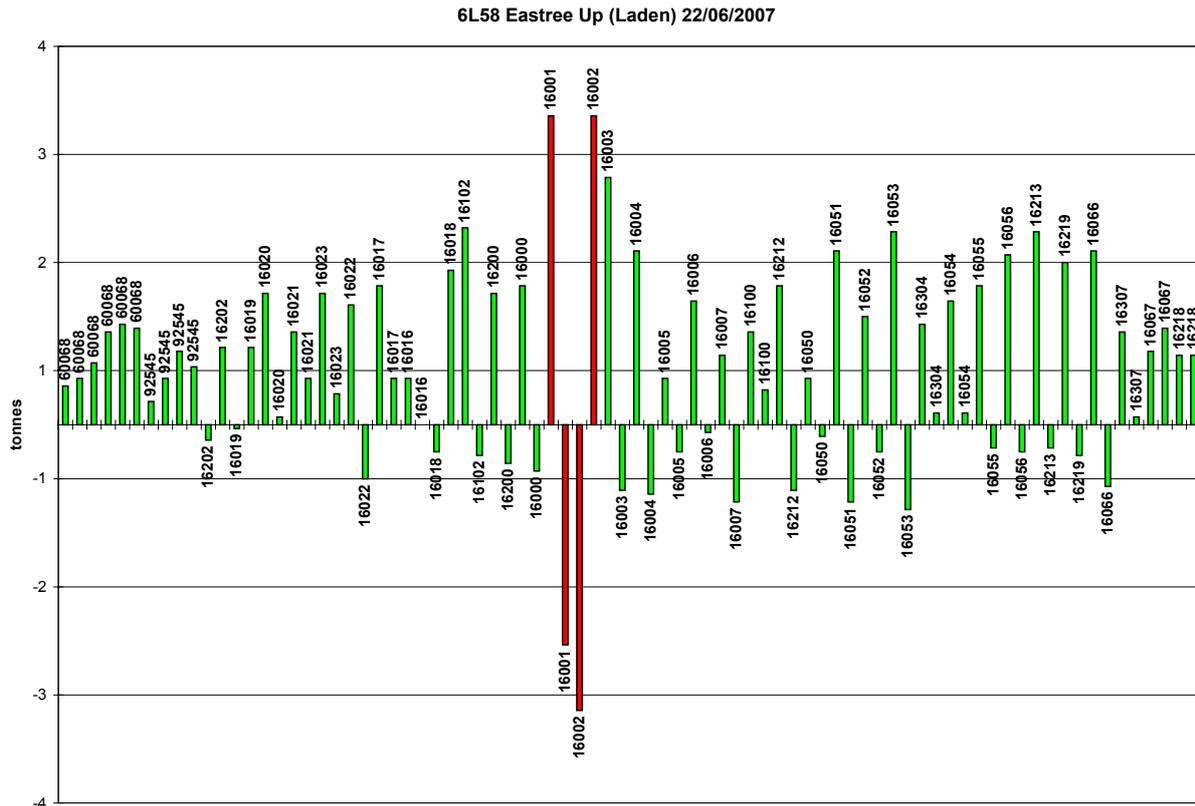
Figure 29: Train consist diagram from the Eastrea Wheelchex site showing incident wagons REDA 16001 and REDA 16002 (both shown in red) and non incident wagons (green)
