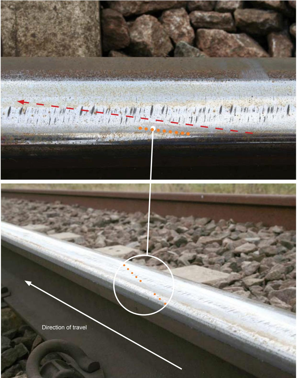
Figure 23a (top) and b (bottom): High right-hand rail showing view of derailment mark on railhead from the four-foot in direction of travel
