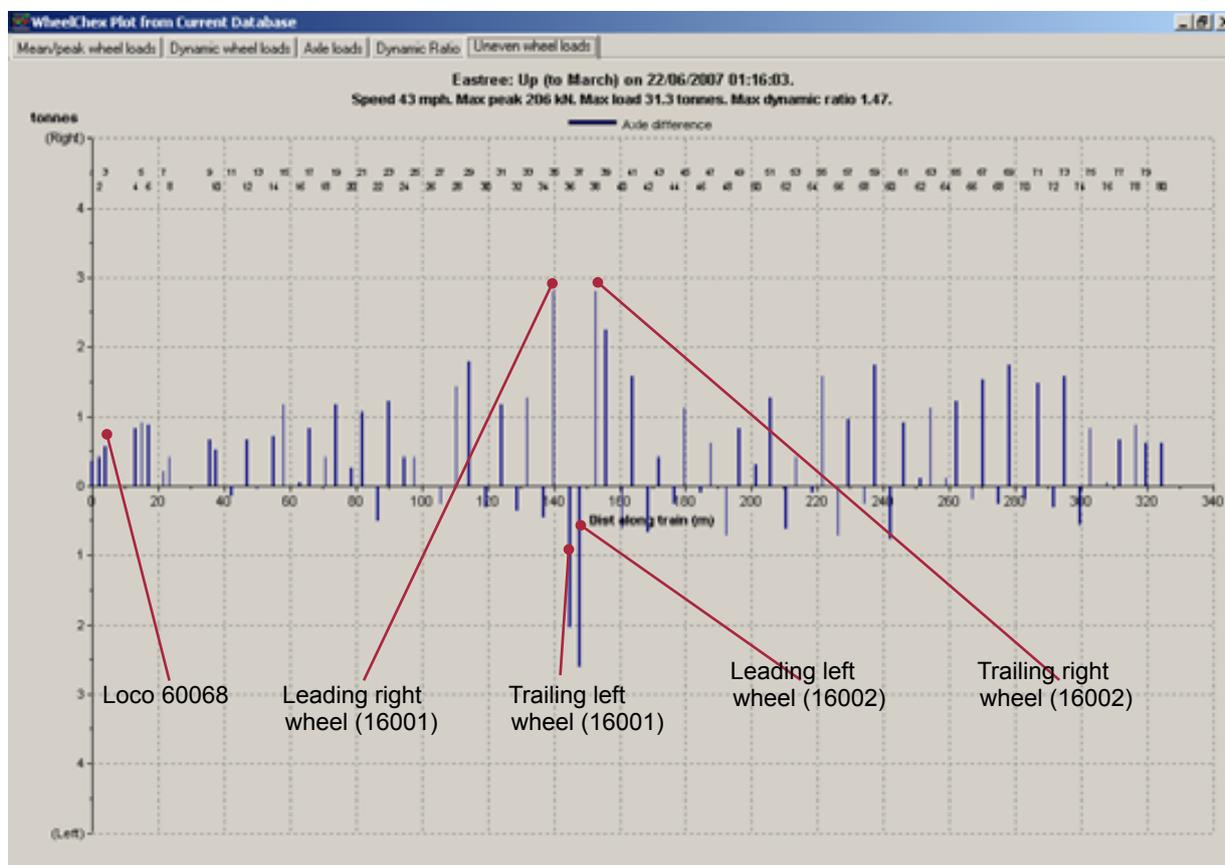
Figure 28: Wheelchex graphs showing uneven wheel loads REDA 16001 and REDA 16002
