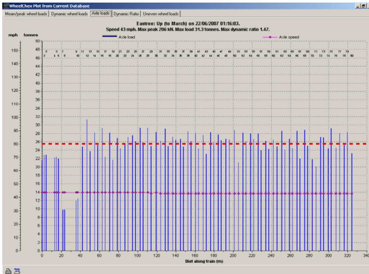
Figure 20: Data from Eastrea Wheelchex site showing axle load of 6L58. Data shows axle loads against datum line of maximum permitted tonnage on each axle (25.5 tonnes)
