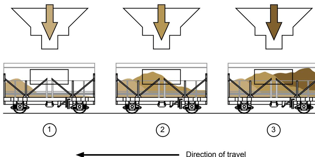
Figure 18: Diagram showing loading procedure and propensity to load wagons rear-axle-heavy
