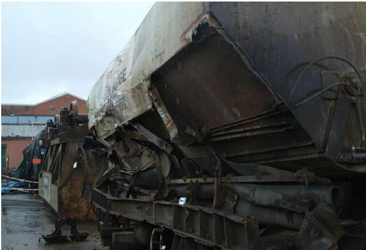
*Figure 34: Left side of wagon REDA 16002 showing severe damage and frame twist caused by incident*
