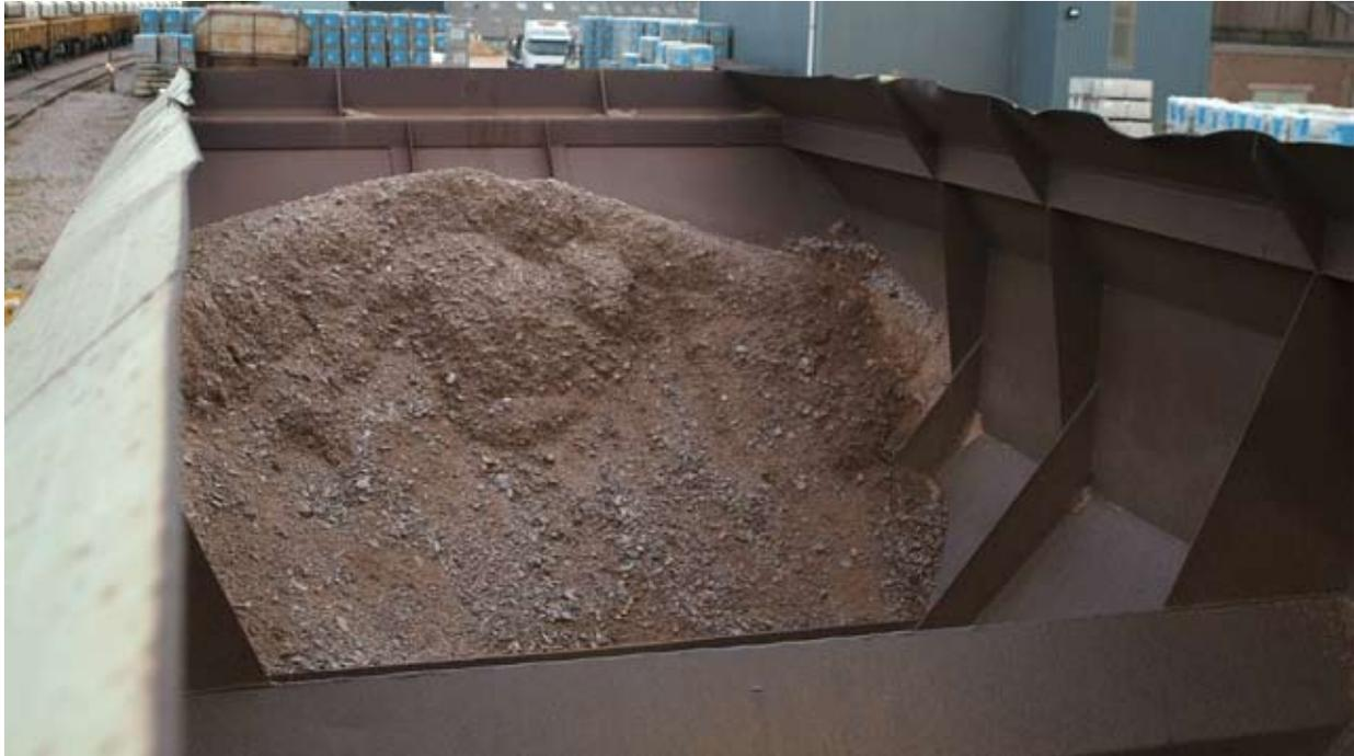
Figure 19: Residual ballast in wagon REDA 16021
