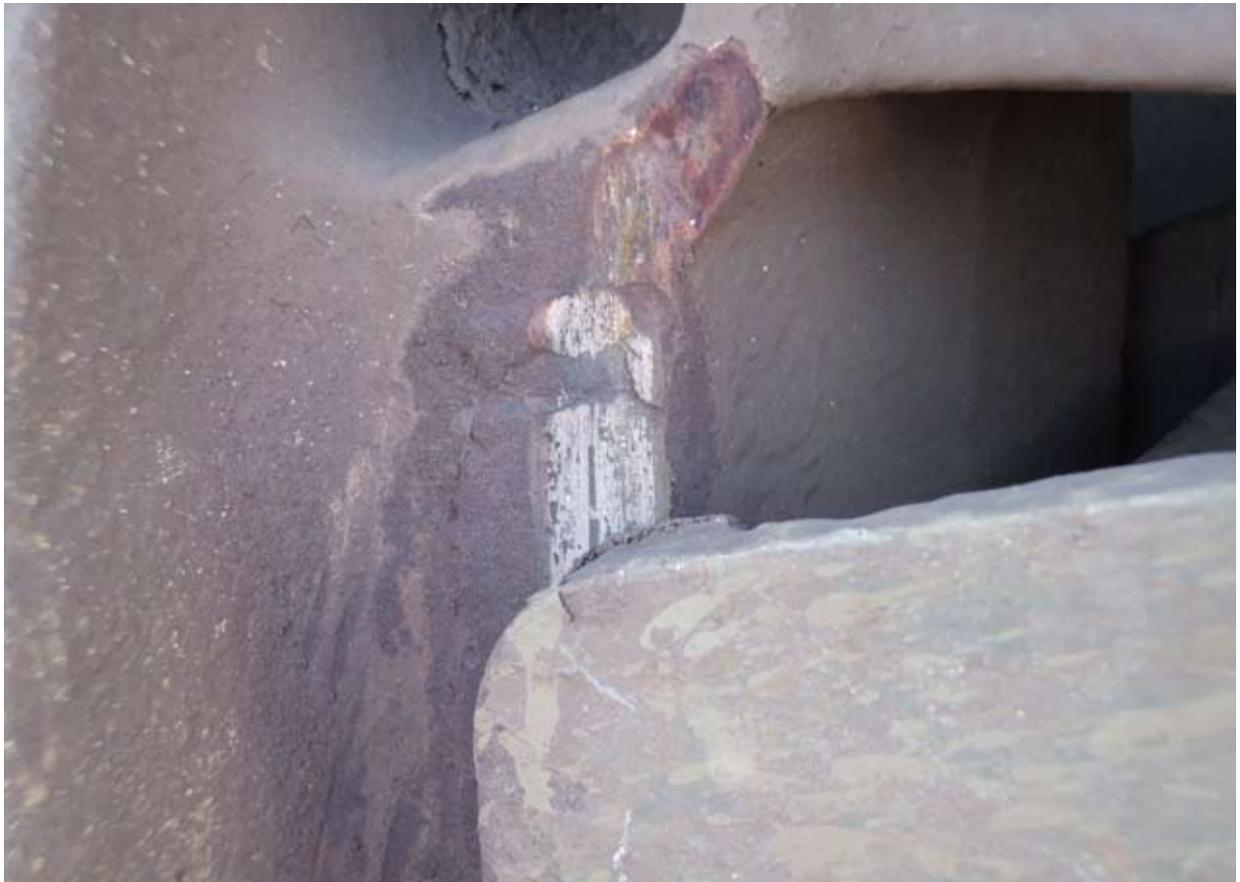
*Figures 51 & 52: Wear and heat damage to pedestal liners of SDT PHA wagons*
