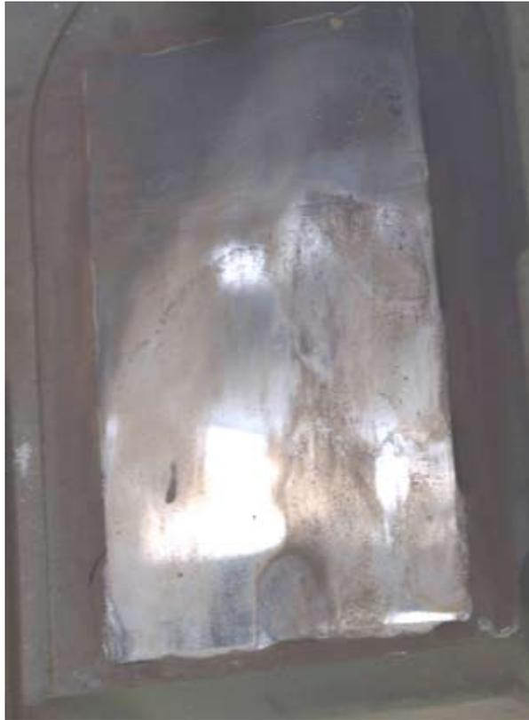
Fig 38: Wear to leading right pedestal guide on REDA 16011 showing polished surfaces but no evidence of heat damage
