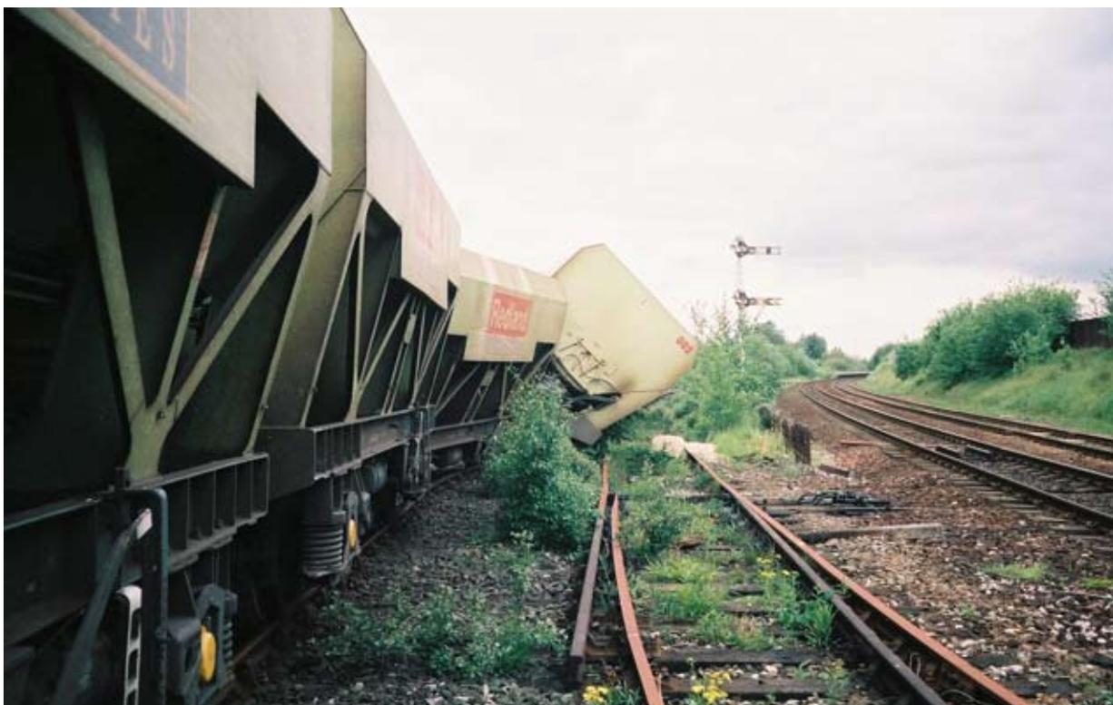
Figure 44: Image showing derailed wagon REDA16002
