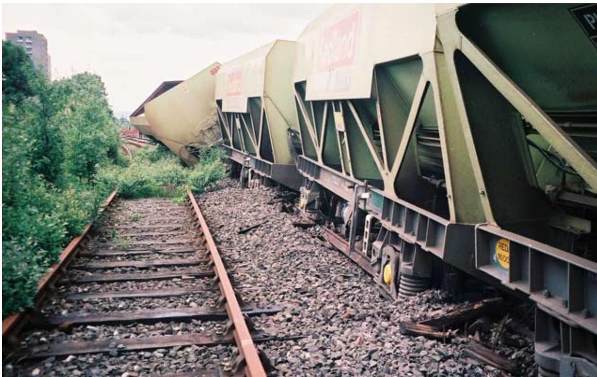
Figure 43: Image showing derailed wagon REDA 16003
