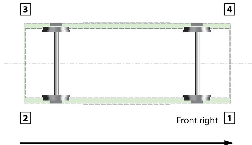
Figure 6: Plan view of PHA wagon with front right and left axle 1 - 4 and rear axle 2 - 3
