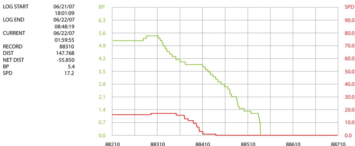
Figure 30: Locomotive 60068 OTDR reading of speed (red trace) and brakepipe pressure (green trace) at 01:59:55 seconds 22 June 2007
