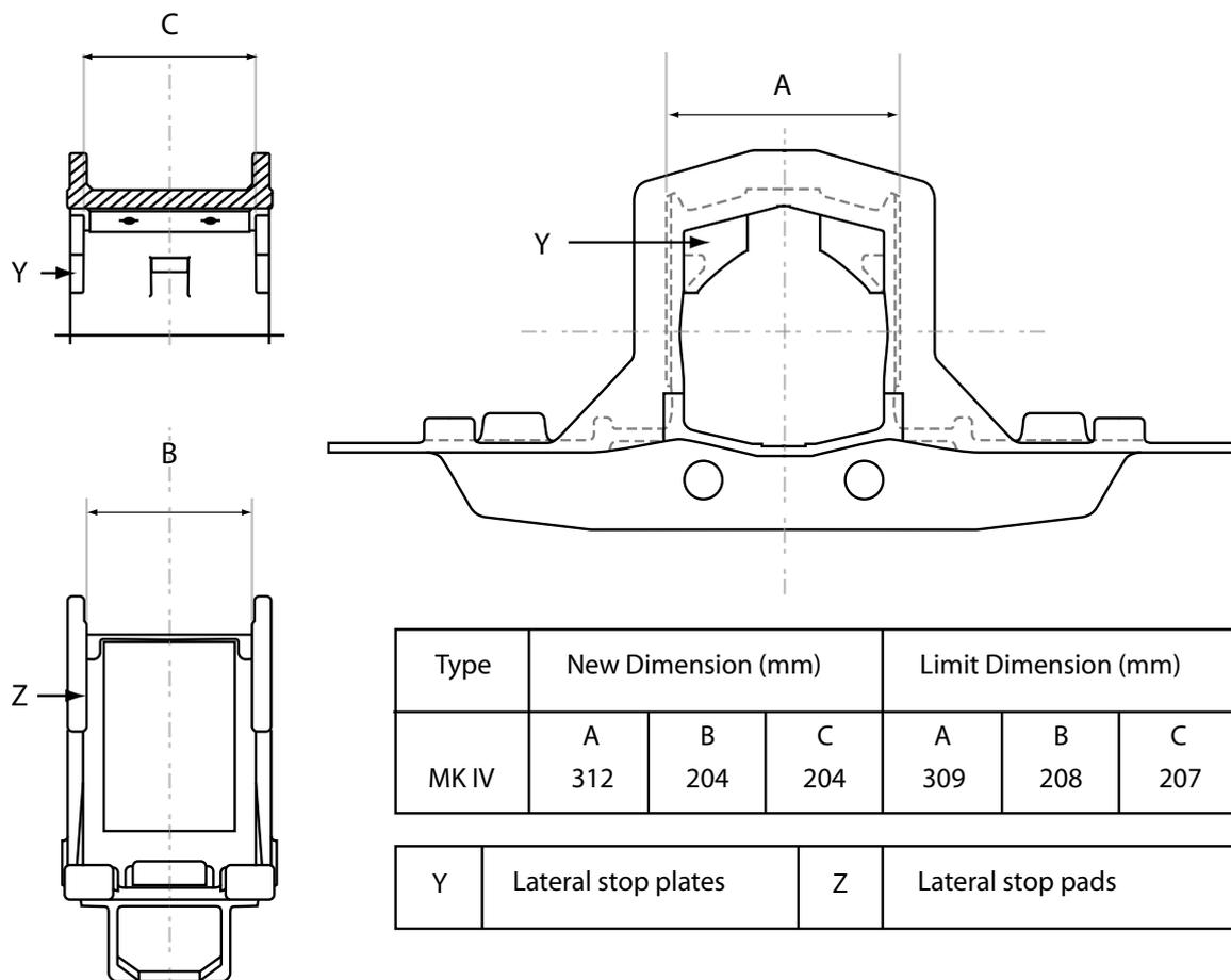
Figure 53: Saddle casting and tolerances
