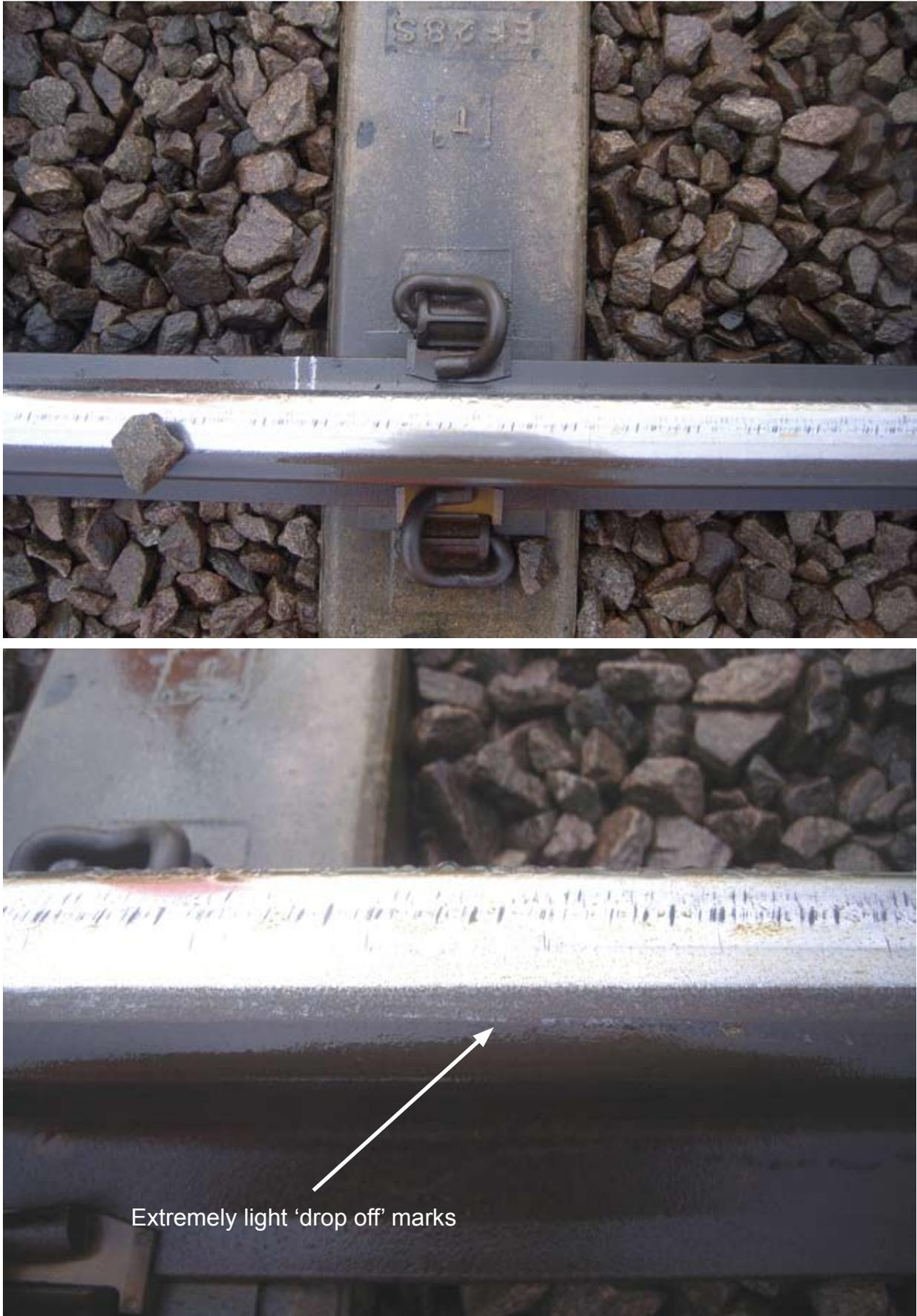
Figure 21a & b: Derailment drop-off mark on high right-hand rail
