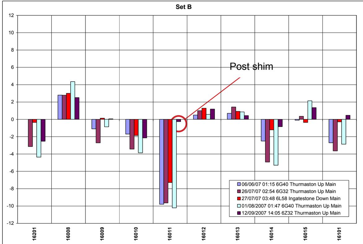
Figure 39: Graph showing analysis of raw Wheelchex data of pre and post frame twist on REDA 16011
