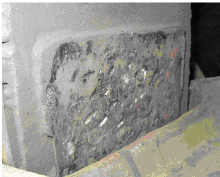
Figure 41: Abnormal wear pattern on friction liner of wagon 14503 identified during Network Rail's audit of Lafarge vehicles in May 2007
