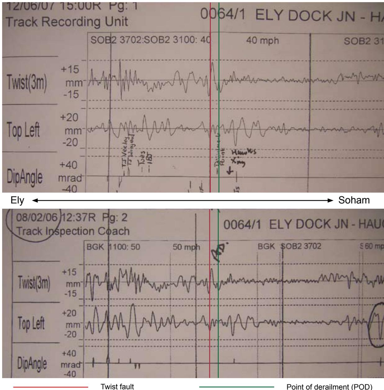
Figure 27: Track recording vehicle data trace from 8 February 2006 (bottom) and 12 June 2007 (top). The horizontal dotted line indicates the intervention limit. The track twist and POD are also shown
