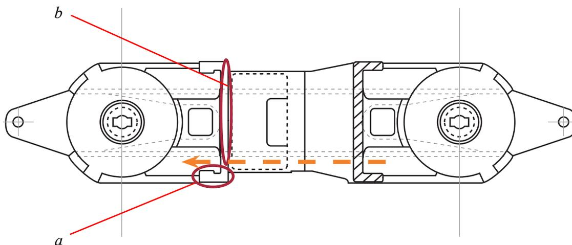
Figure 50: Plan view of Leading RHS pedestal and saddle showing area of frictional heat generation at (a) lateral guide and (b) friction liner
