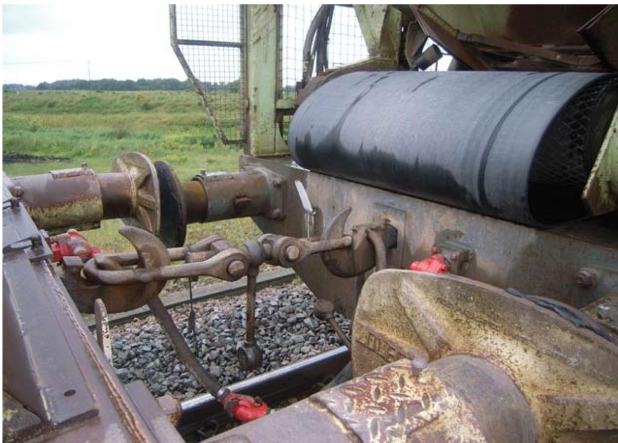
Figure 4: REDA coupling arrangement
