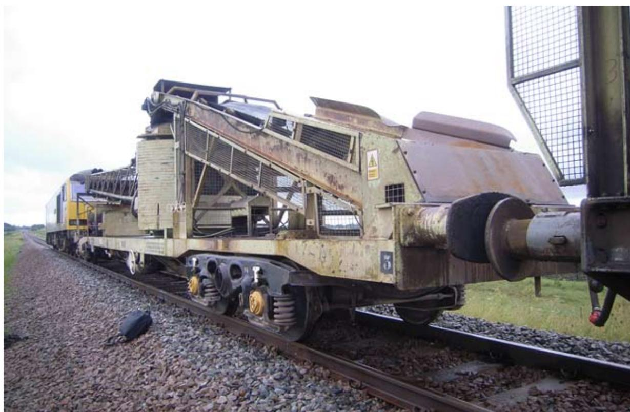
Figure 5: Self-discharge train incorporating the off-load wagon showing the conveyer belt arrangement
