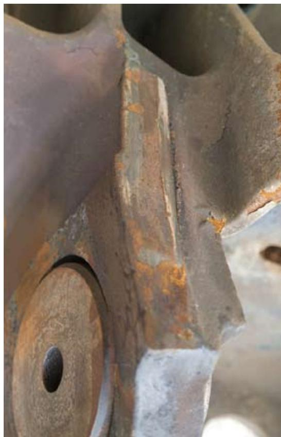
Figures 32 (left) with inset. Front portion of inner aspect of the right-hand pedestal showing heat damage. Figure 33 (right). Heat damage to rear portion of inner aspect of pedestal guide.
