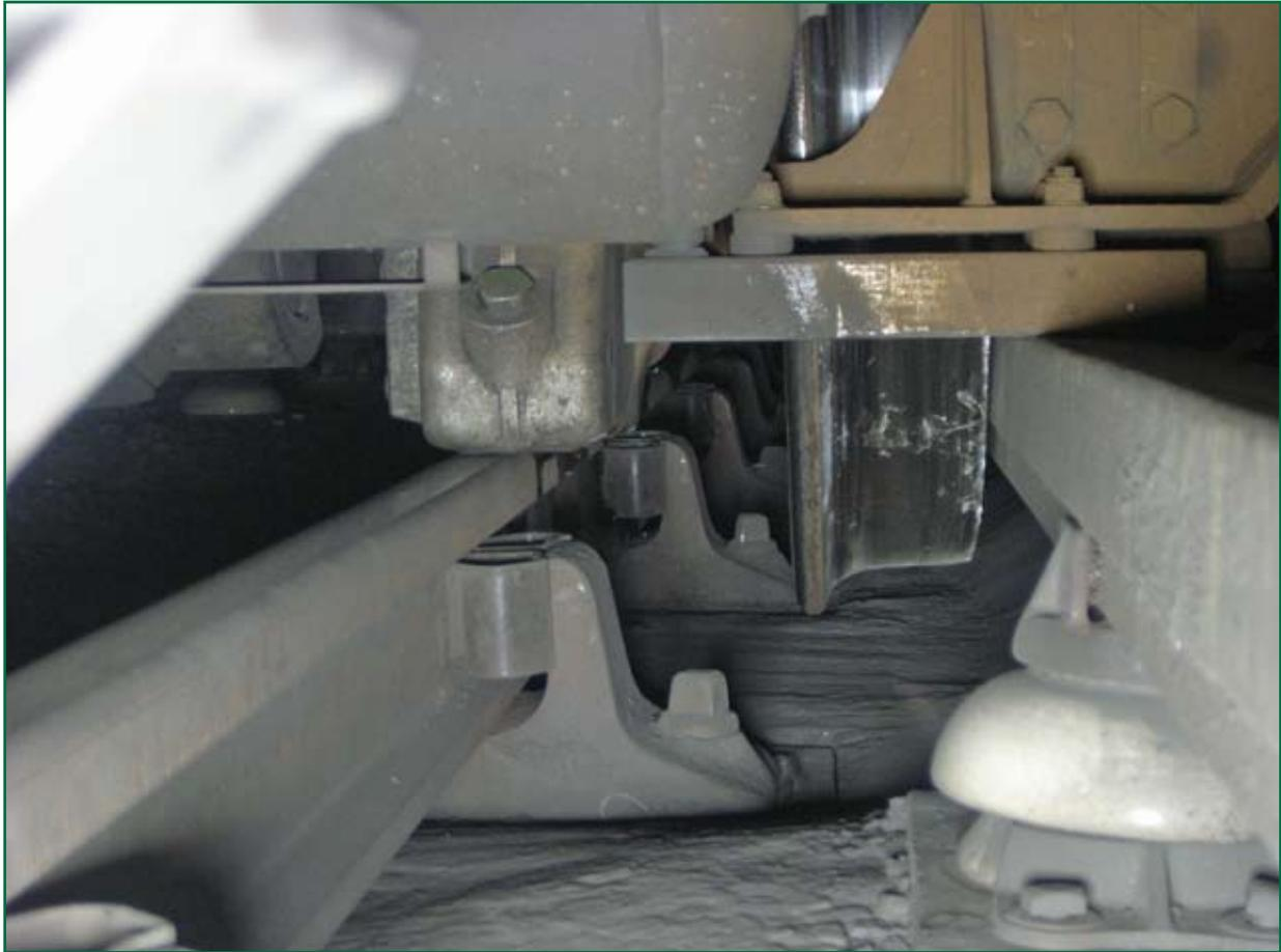
*Figure 15: Photograph showing how the conductor rail has helped to guide the bogie*
