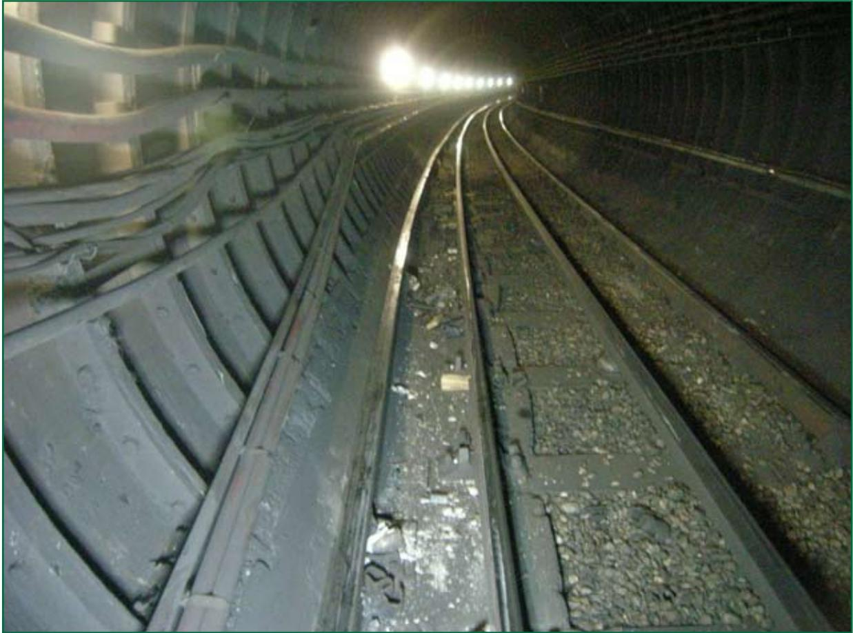
Figure 6: Track damaged by the derailment after the train had been removed
