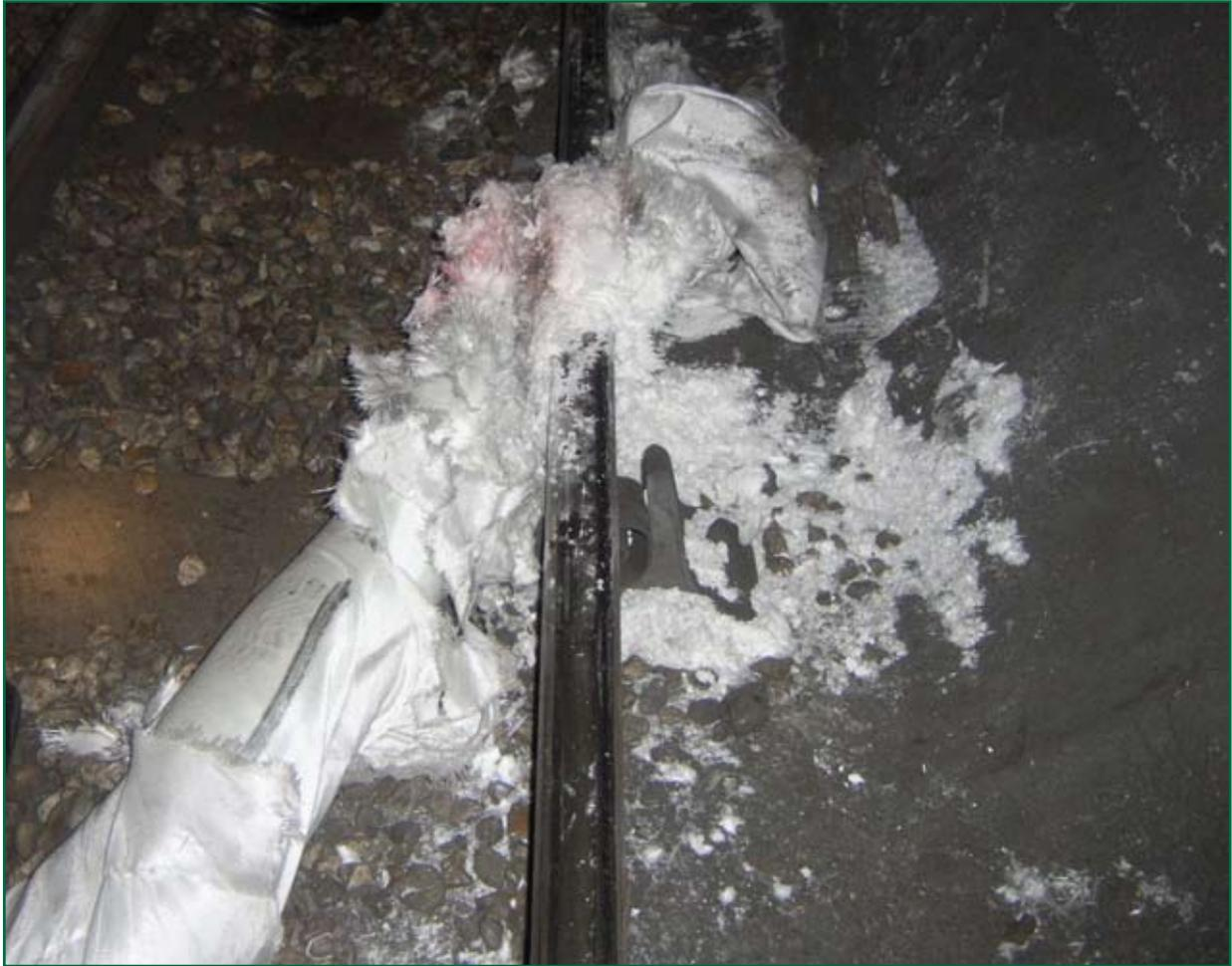
Figure 4: The remains of the fire-blanket after train 117 had passed over it
