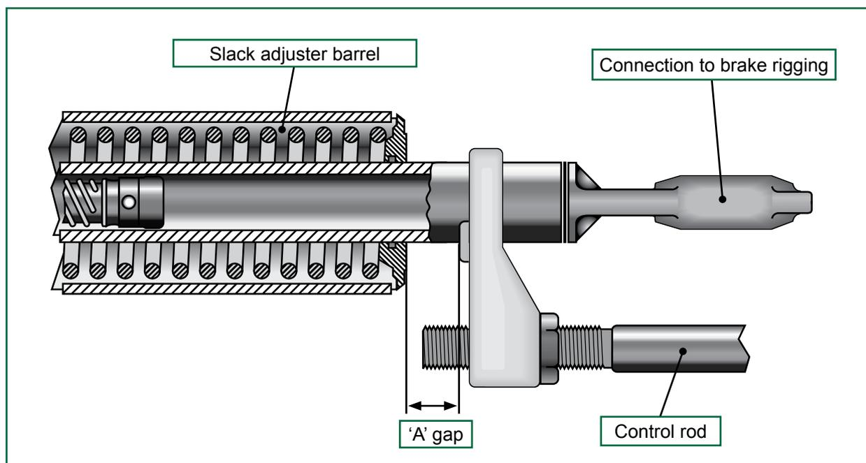
Figure 15: Slack adjuster ‘A’ gap
