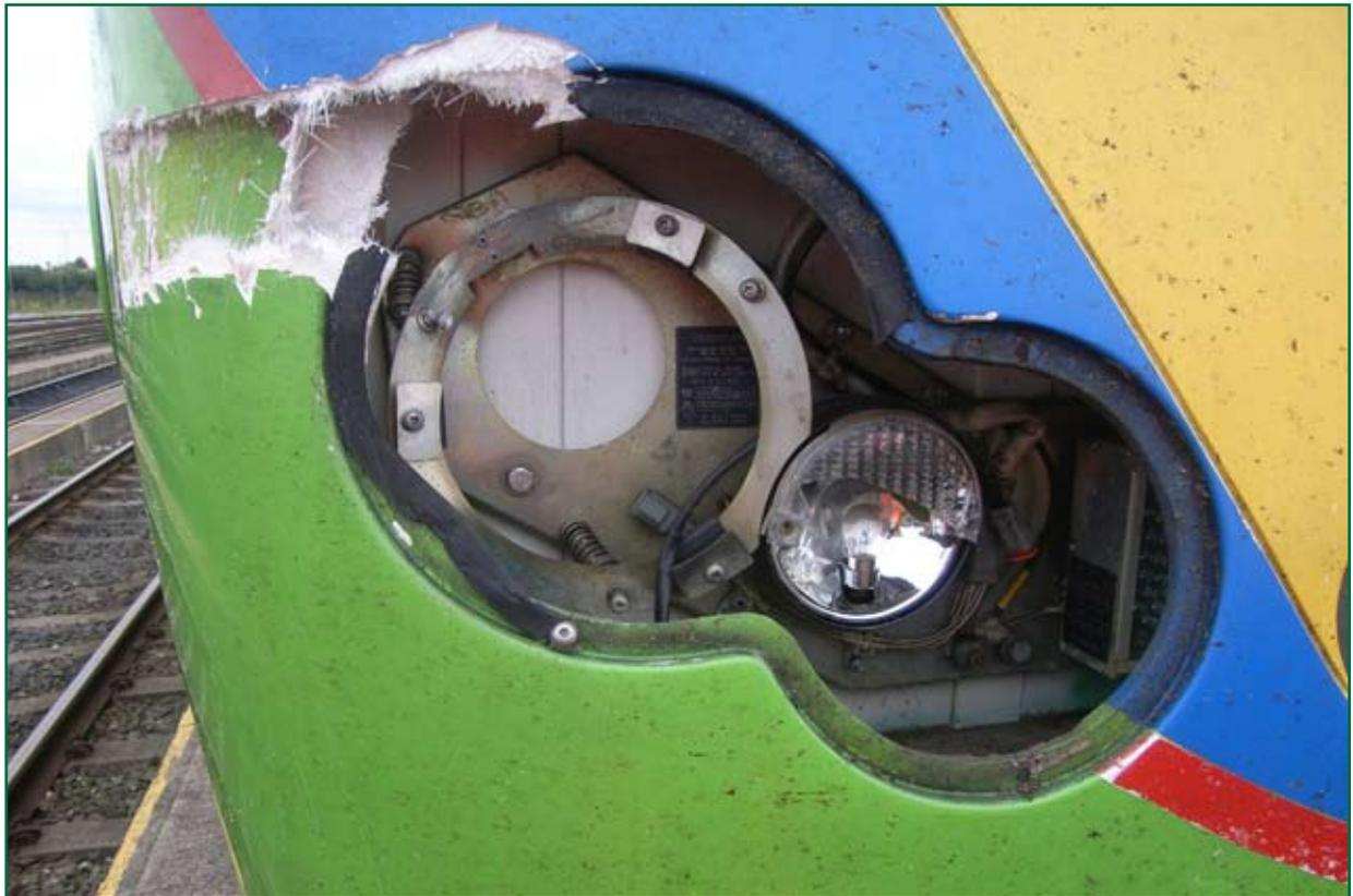
Figure 7: Damage to the cab and light unit
