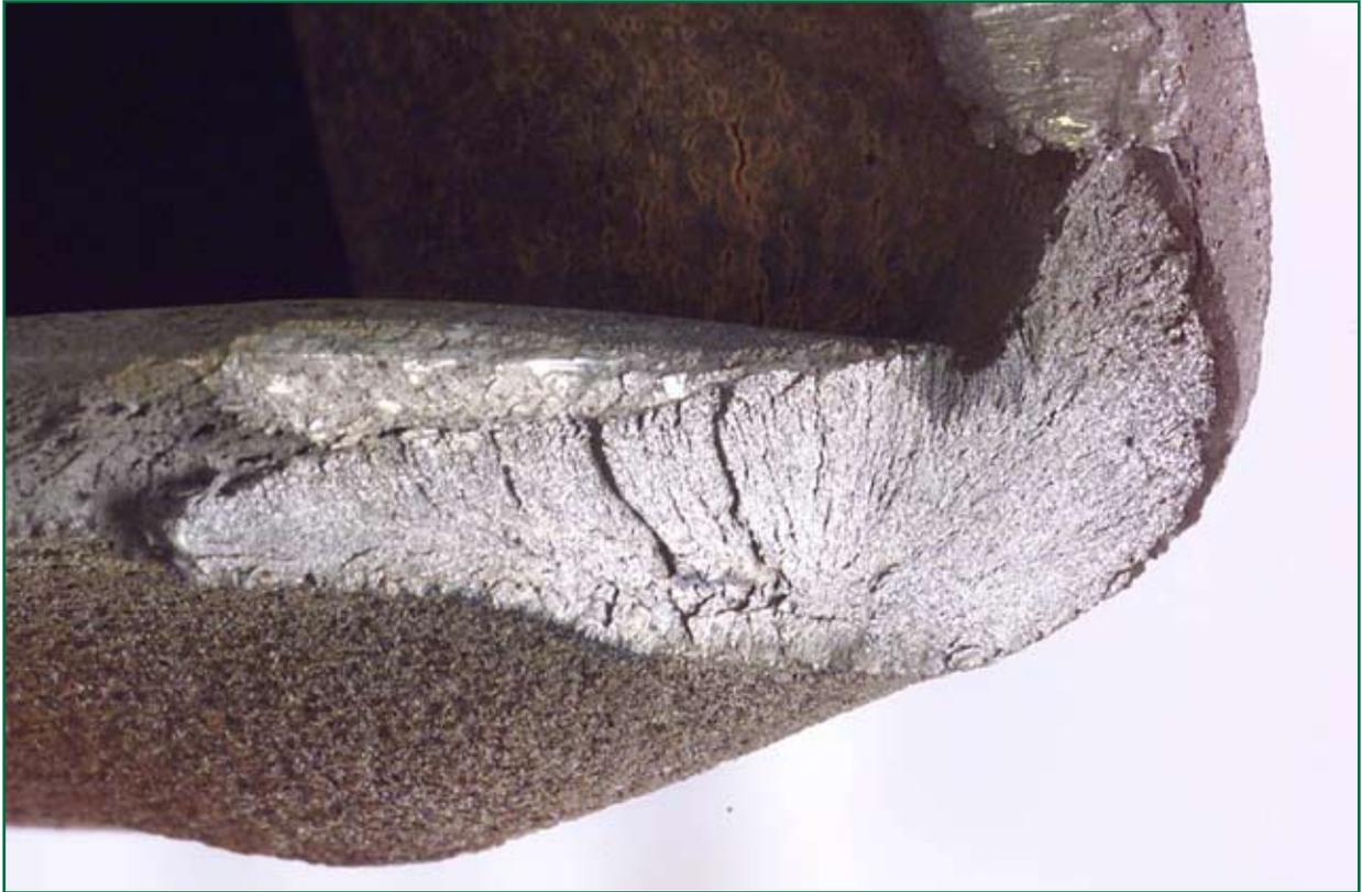
Figure 15: Cracking from the outside of one corner after corrosion removal (photograph courtesy of Serco Technical & Assurance Services, Derby)
