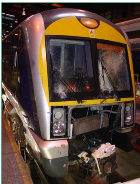
Figure 3: Damage to the front of unit 3014 (3 August 2007)
