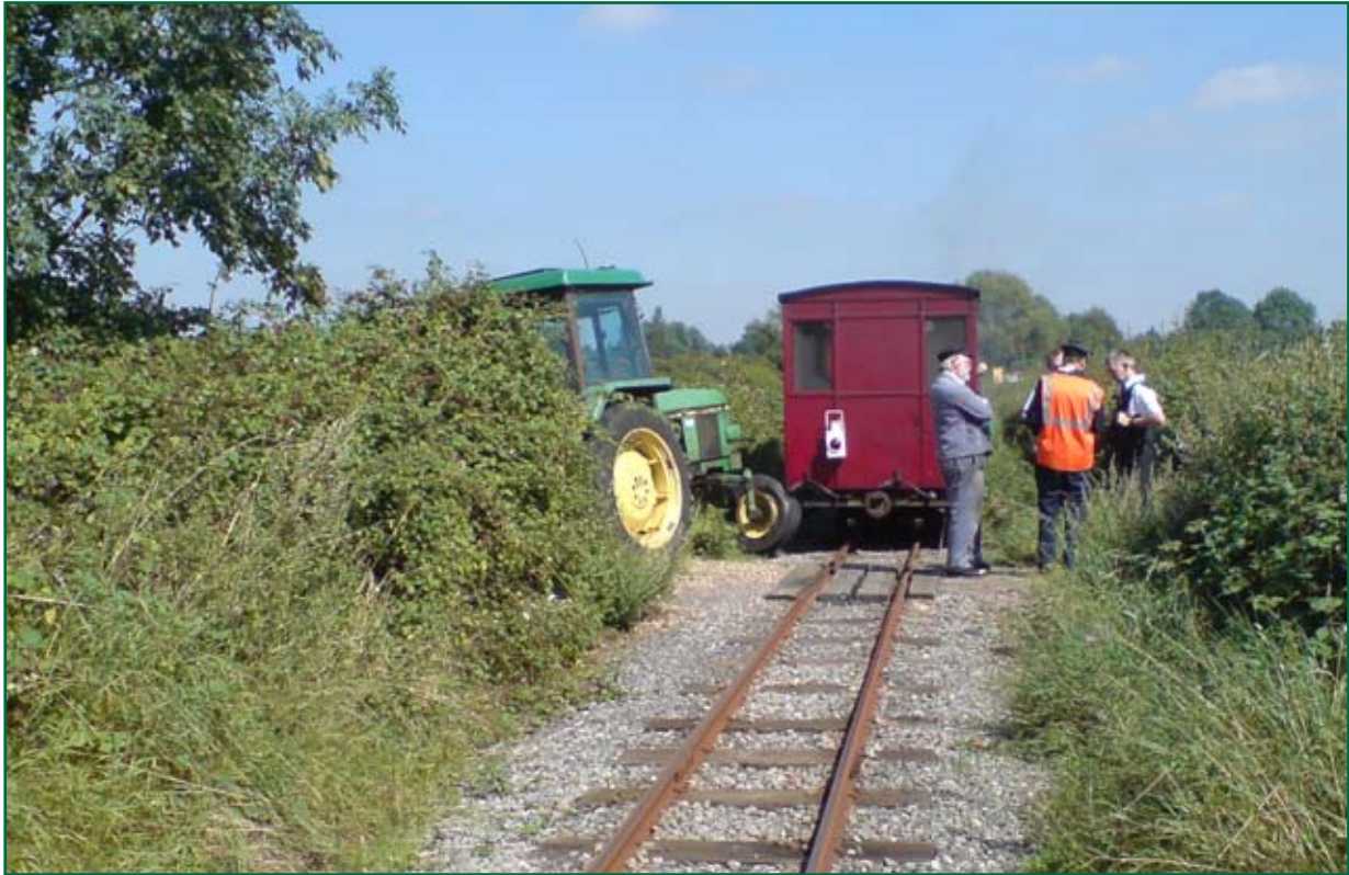
Figure 3: Position of train and tractor after collision (courtesy Leighton Buzzard Railway)
