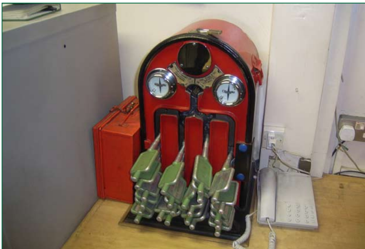
Figure 5: Token instrument at Aylesbury traincrew supervisor's office
