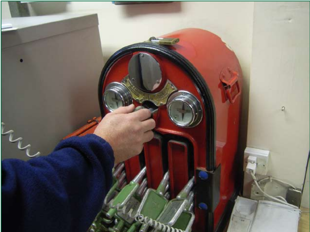
Figure 6: Token being taken from the machine
